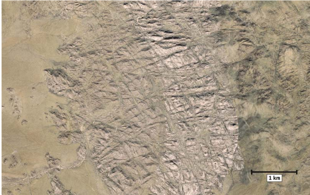
Figure 1.1 Fractures at many scales and orientations can occur at a single site. The satellite image shows the superposition of multiple large-scale fracture sets (lineaments) of different orientations in the quartz monzonite of Joshua Tree, California. The scale line in the lower right hand corner represents 1 km (Engelder, 2013 workshop presentation). SOURCE: Imagery © 2015 Google, Map data © 2015 Google.
