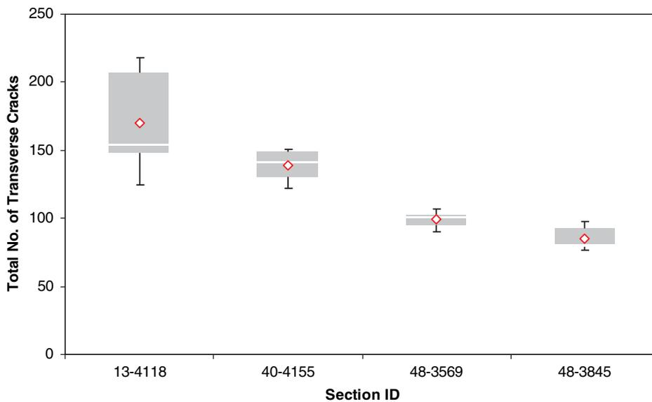
**Figure B.17.** Distribution of number of transverse cracks for CRCP sections.
