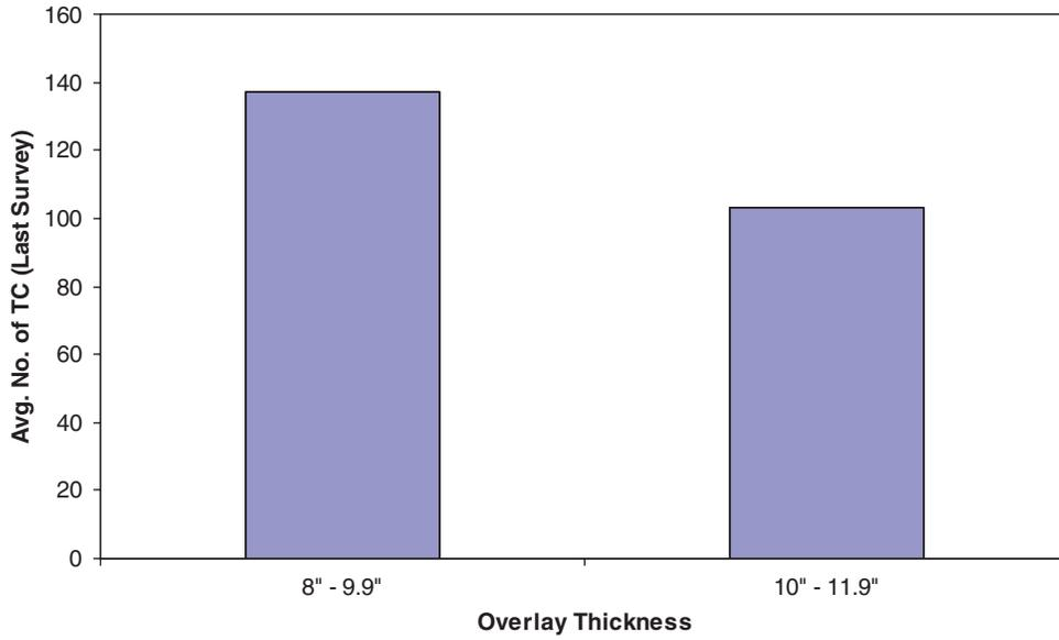
**Figure B.18. CRCP overlay thickness versus average number of transverse cracks.**
