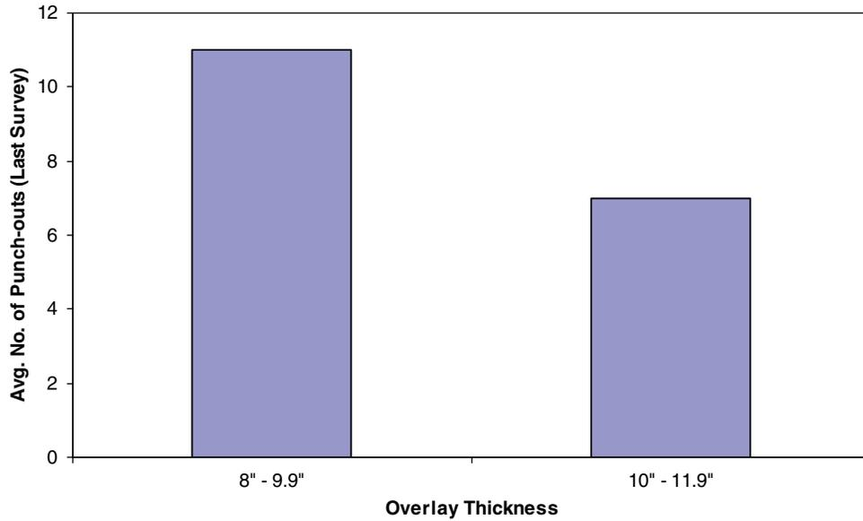
Figure B.21. CRCP overlay thickness versus average number of punchouts.
