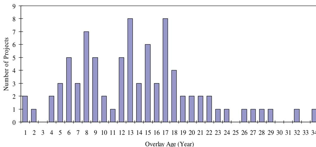
Figure B.1. Frequency of overlay age within experiment GPS-6A.
