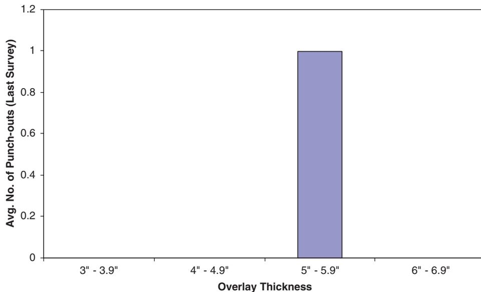
**Figure B.44. CRCP and PCP overlay thickness versus number of punchouts.**
