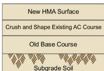
**Figure A.2. Schematic of HMA over crushed and shaped HMA pavement.**
