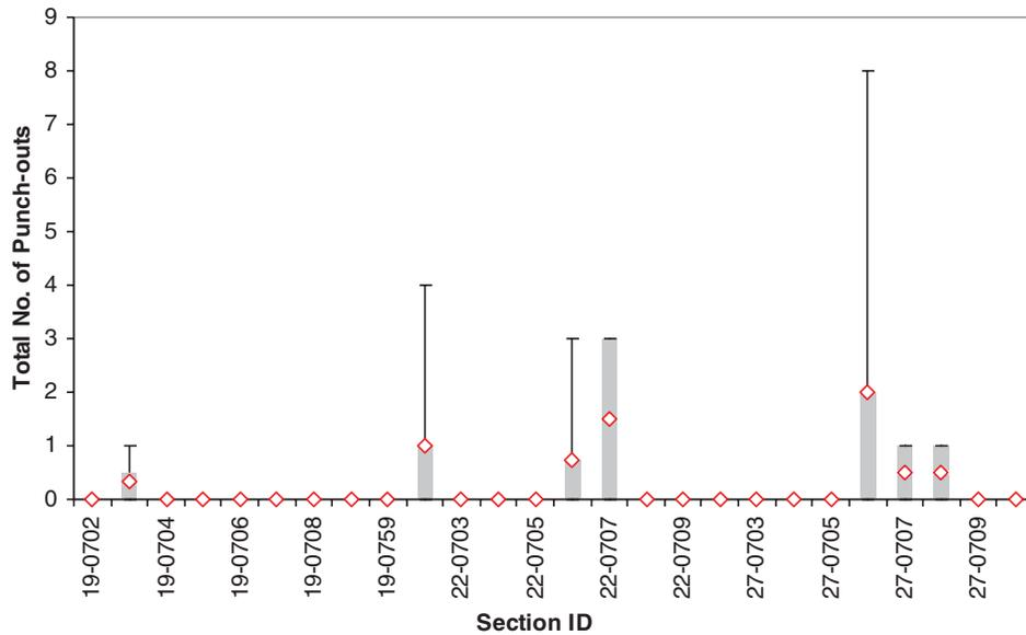
**Figure B.43. Distribution of number of punchouts for CRCP and PCP sections.**
