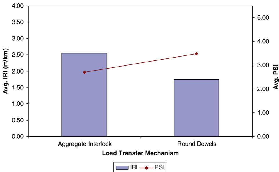
**Figure B.31. JPCP load-transfer mechanism versus average IRI and average PSI.**
