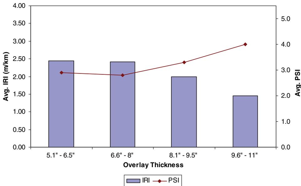
Figure B.24. Overlay thickness versus average IRI and average PSI.
