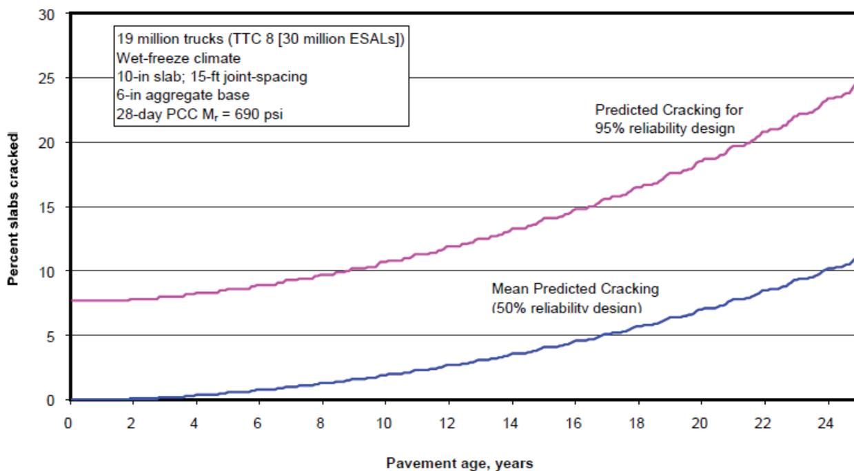
**Figure D.1. Slab cracking.**
