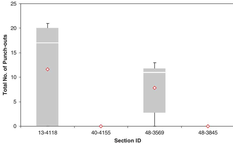
Figure B.20. Distribution of number of punchouts for CRCP sections.
