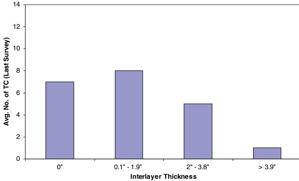
**Figure B.28. JPCP interlayer thickness versus average number of transverse cracks.**
