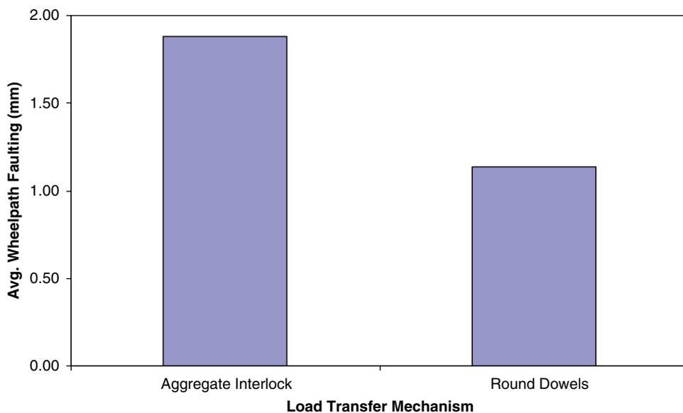
**Figure B.30. JPCP load-transfer mechanism versus average wheelpath faulting.**
