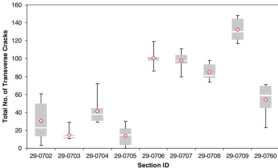
Figure B.39. Distribution of number of transverse cracks by JPCP sections.
