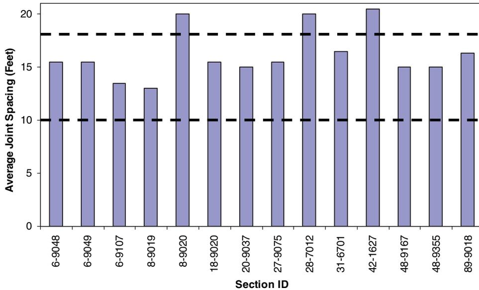
Figure B.13. JPCP average joint spacing.
