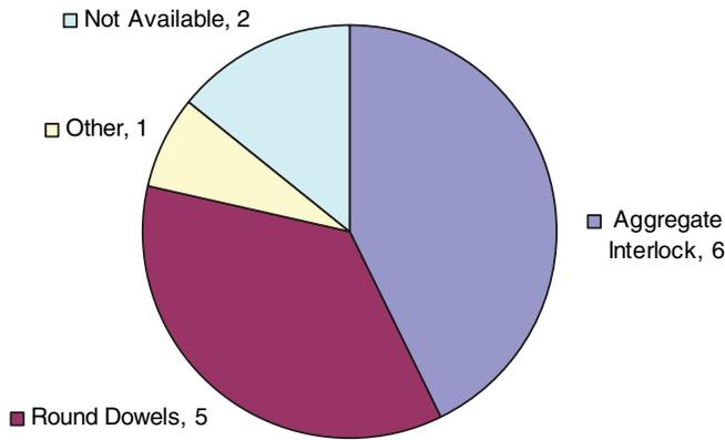
**Figure B.14. JPCP load-transfer mechanisms.**
