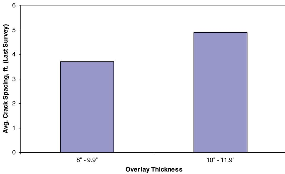
**Figure B.19. CRCP overlay thickness versus average crack spacing.**
