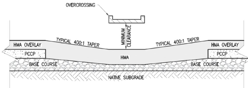
**Figure 3.8. Illustration of flexible pavement transitions to overcrossings.**
