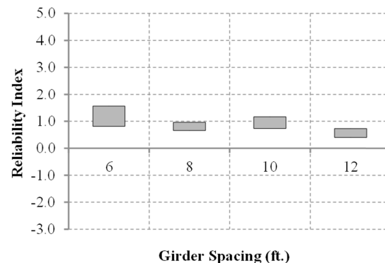
Figure 6.29. Reliability indices of various bridge decks designed using a 1.0 live load factor over a 1-year return period (ADTT = 5,000) for negative moment region, Class 2 exposure.
