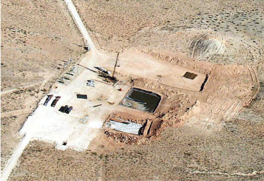
Drilling activity in the Permian Basin, which accounts for most of Texas' oil production. Roads at each site must be able to handle approximately 1,054 two-way truck trips.
