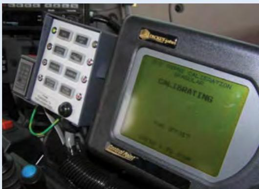
A ground-speed controller in calibration mode.
