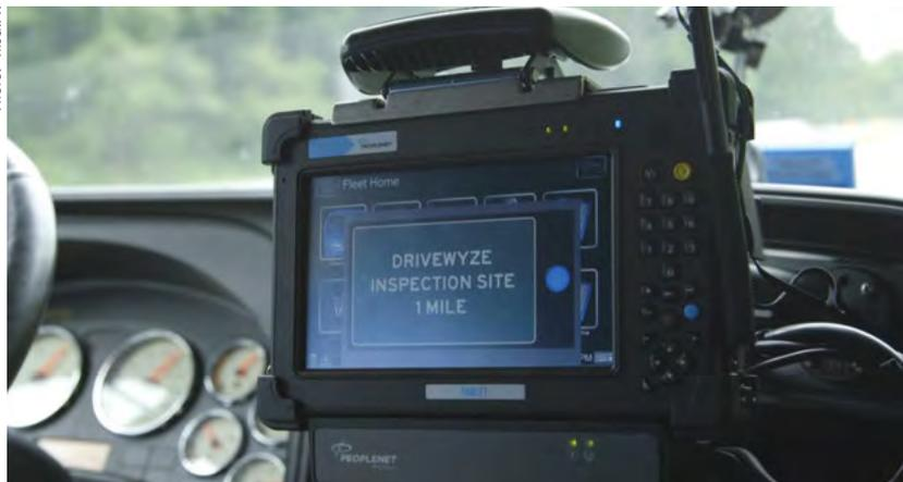
Many commercial vehicle-to-infrastructure technologies already are on the market, including the Drivewyze system that provides weigh-station bypasses for truck drivers.
