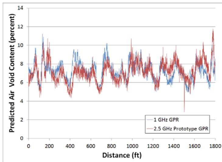
**Figure 3.7. Correcting for drift with 2.5 GHz data results in favorable comparison with a 1 GHz system.**
