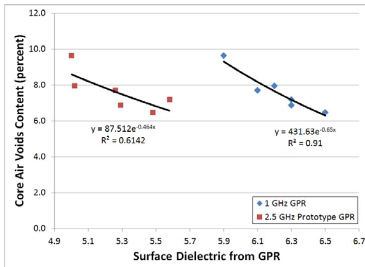
**Figure 3.12. Calibration of air voids to GPR from Route 3.**
