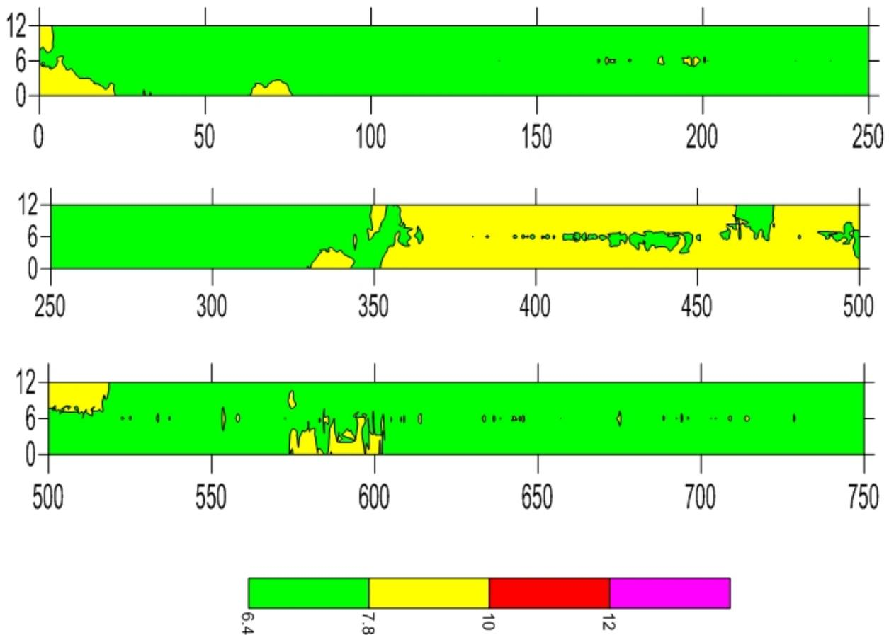
**Figure 3.15. Geospatial distribution of air voids on Route 3 from 2.5 GHz GPR.**
