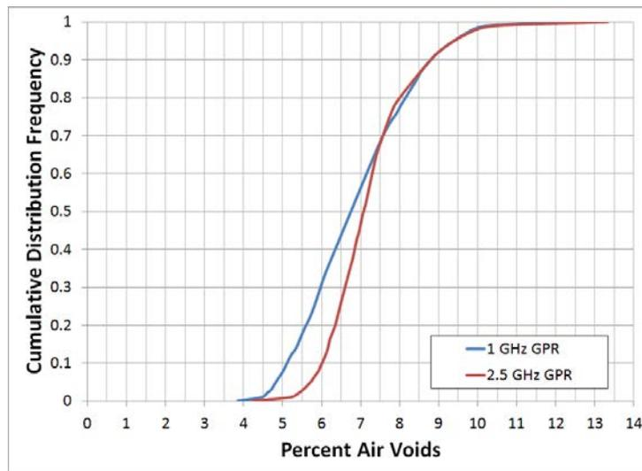
**Figure 3.21. Expected distribution of air voids on SR-220.**
