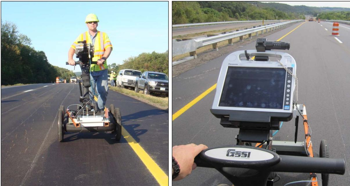
**Figure 3.19. Collection of GPR data on SR-220 with real-time data processing.**
