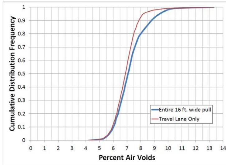
**Figure 3.23. Expected entire pull and travel lane distribution of air voids on SR-220 from 2.5 GHz GPR.**
