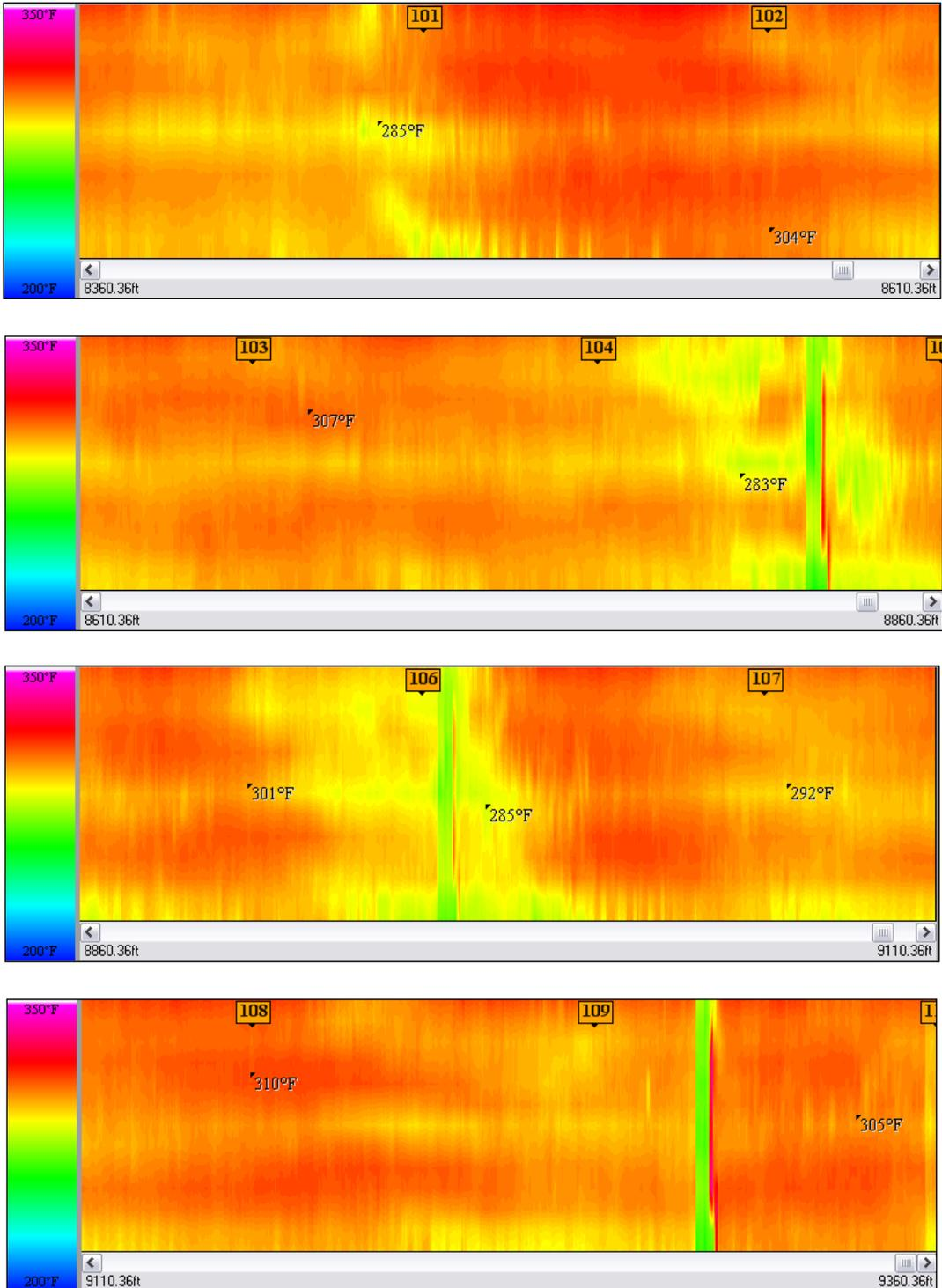
Figure 3.18. Thermal profile from last 1,000 ft of SR-220 placed 09/06/2013.
