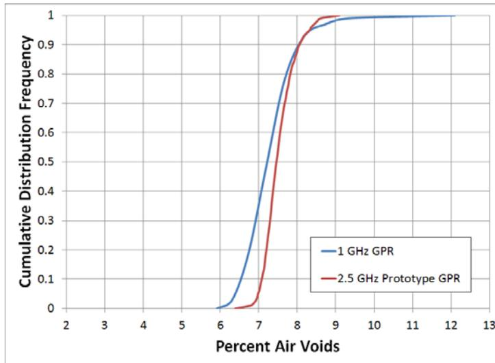
**Figure 3.13. Expected distribution of air voids on Route 3 from GPR. Note: VDOT desired density is  $\leq 7.8\%$  air voids.**
