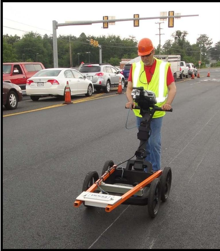
**Figure ES.2. GPR System for measuring asphalt mixture uniformity.**
