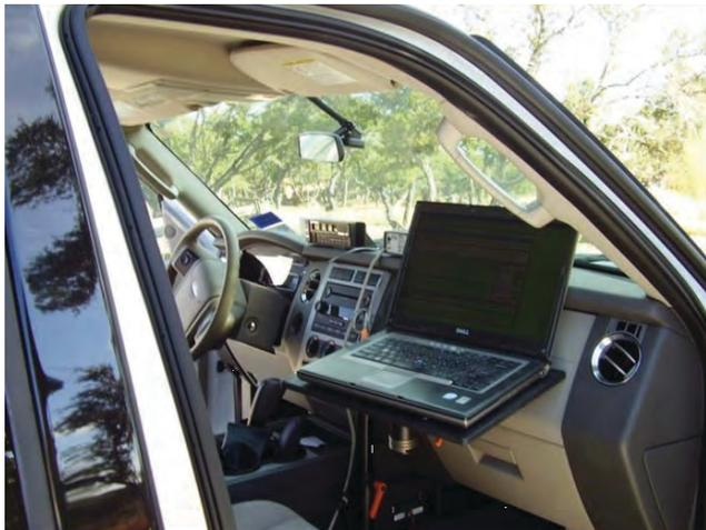
FIGURE 12 Instrumented vehicle used in Tennessee data collection.
