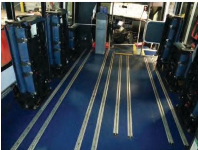
**Figure 4-1. Laketrans vehicle with full-length securement tracking, looking forward from the rear (photo courtesy of Laketrans).**
