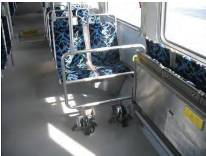
**Figure 4-4. Modified “reach-through” panel behind securement area, designed by GET (photo courtesy of GET).**
