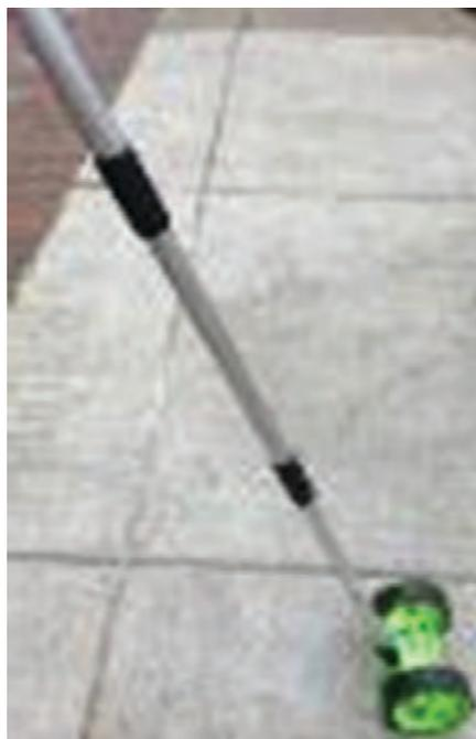
**Figure 5-5. Measuring wheel.**
