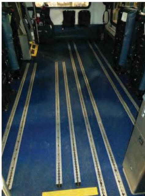
**Figure 4-2. Laketrans vehicle with full-length securement tracking, looking rearward from the front. (photo courtesy of Laketrans).**
