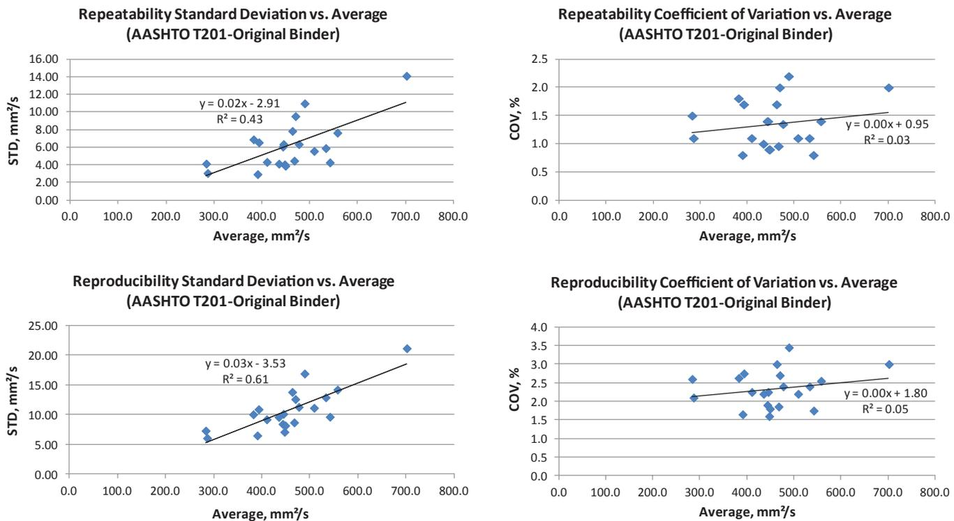
**Figure 2-1** Relationship between average and standard deviation and between average and coefficient of variation of kinematic viscosity (AASHTO T 201) test results for original asphalt.
