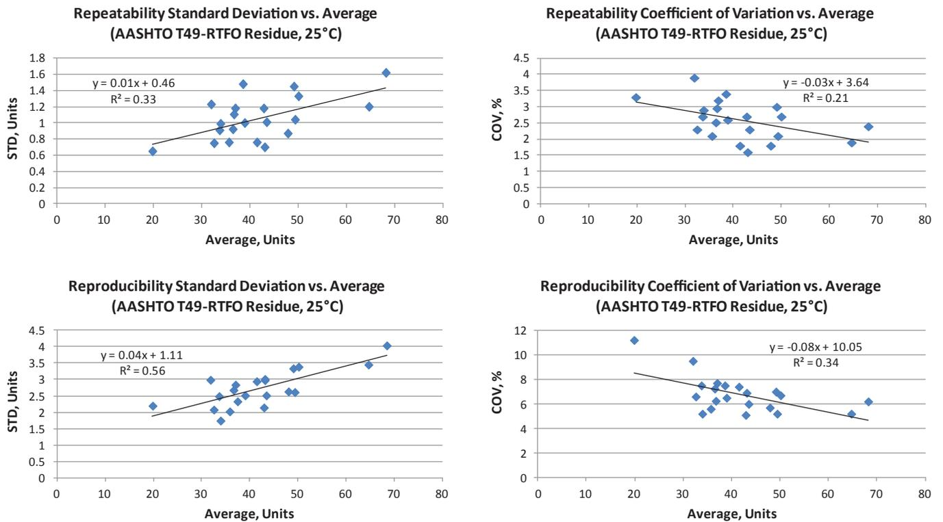
**Figure 2-8** Relationship between average and standard deviation and between average and coefficient of variation for penetration (AASHTO T 49) of RTFO residue at 25°C.
