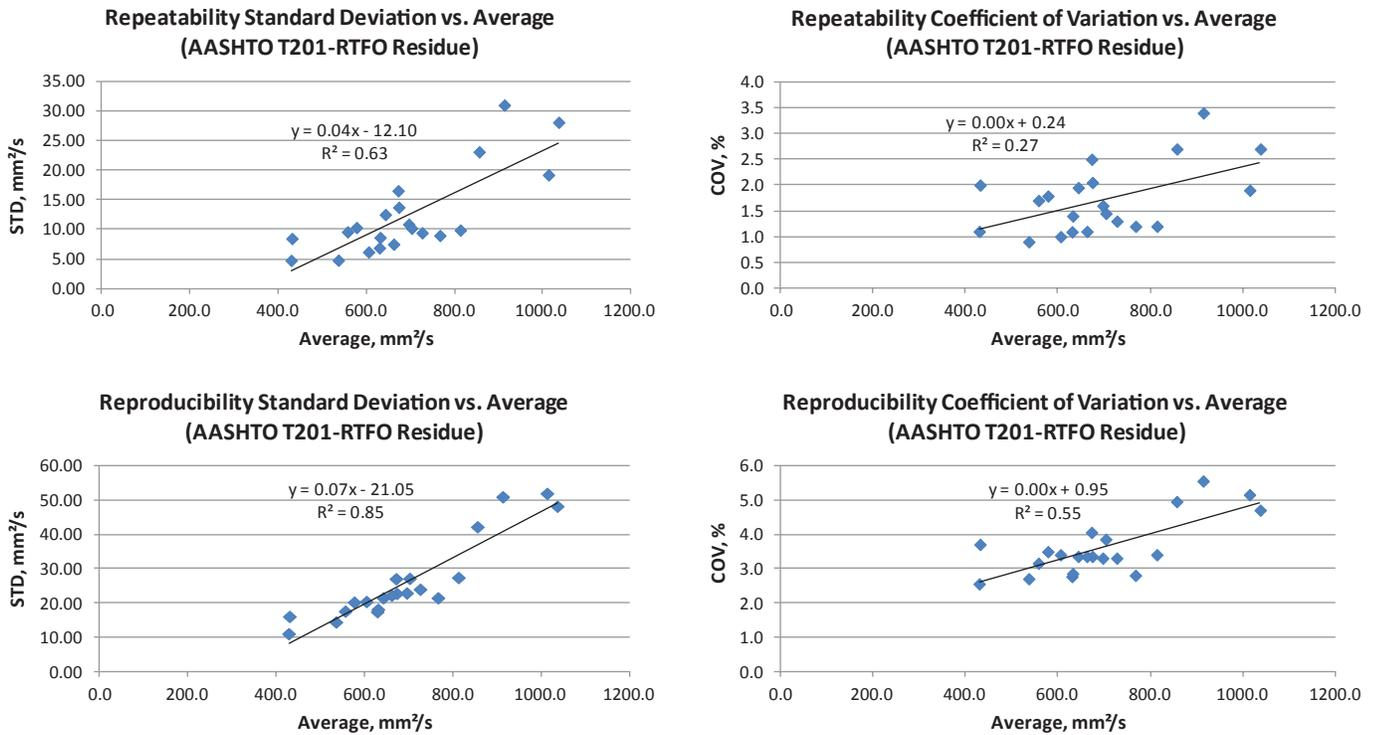
**Figure 2-2** Relationship between average and standard deviation and between average and coefficient of variation of kinematic viscosity (AASHTO T 201) test results for RTFO residue.
