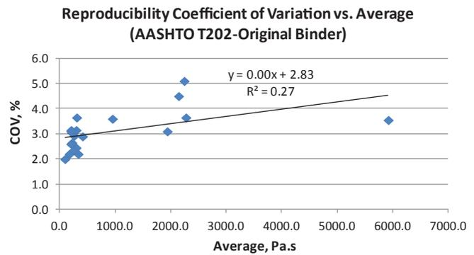
**Figure 2-3** Relationship between averages and standard deviations and between averages and coefficients of variation of the viscosity of asphalts by vacuum capillary viscometer of original asphalt (AASHTO T 202) test method.
