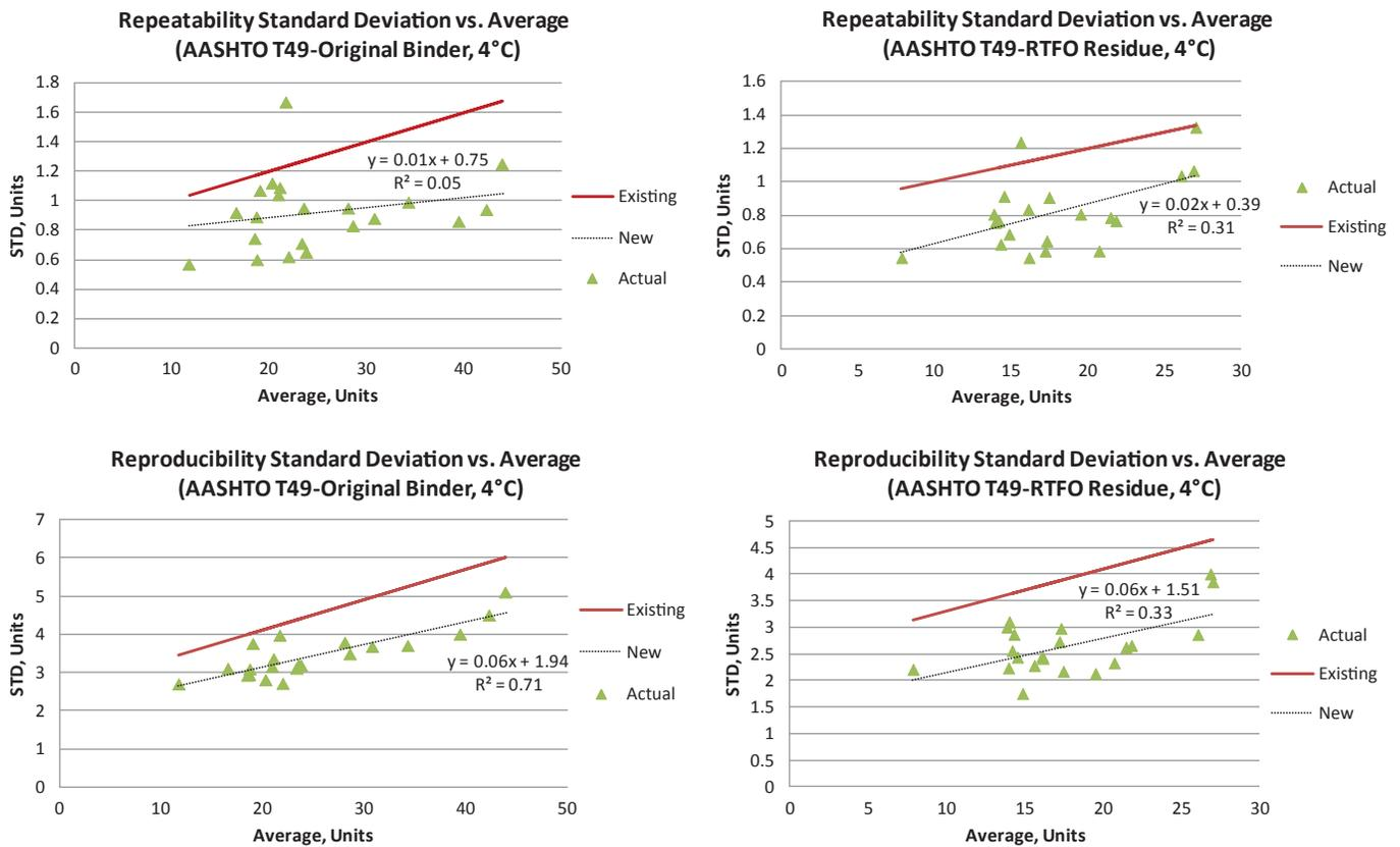
**Figure 2-9** Comparison of the existing and new repeatability/reproducibility standard deviations for penetration (AASHTO T 49) of original binder and RTFO residue at 4°C.
