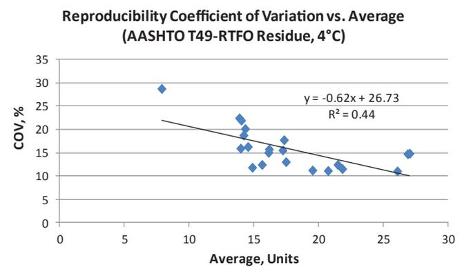
**Figure 2-6** Relationship between average and standard deviation and between average and coefficient of variation for penetration (AASHTO T 49) of RTFO residue at 4°C.
