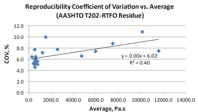
**Figure 2-4** Relationship between averages and standard deviations and between averages and coefficients of variation of the viscosity of asphalt by vacuum capillary viscometer of RTFO residue (AASHTO T 202) test method.
