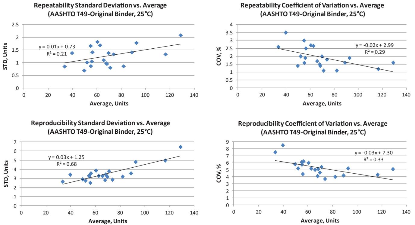
**Figure 2-7** Relationship between average and standard deviation and between average and coefficient of variation for penetration (AASHTO T 49) of original asphalts at 25°C.
