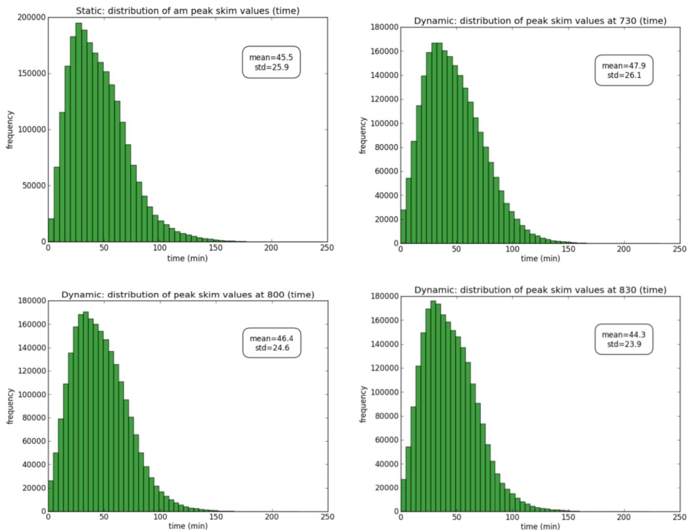
Figure 3.8. Static and dynamic skim differences, a.m. peak period.
