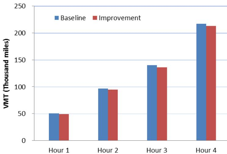
**Figure 3.10. Variation in VMT of all source types from DynusT simulation by hour for baseline and intersection improvement scenarios.**
