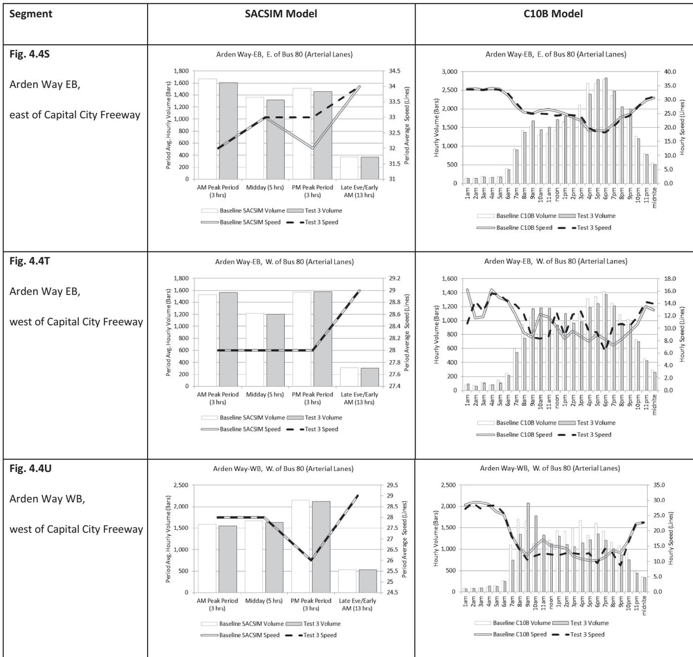
**Figure 4.4. Vehicle volumes and speeds on key test segments—Test 3 (continued).**
