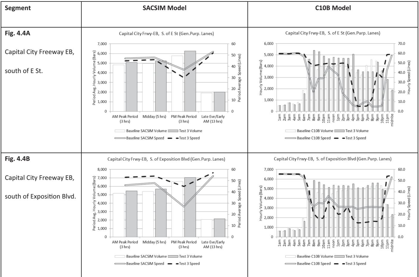
Figure 4.4. Vehicle volumes and speeds on key test segments—Test 3. (Continued on next page.)
