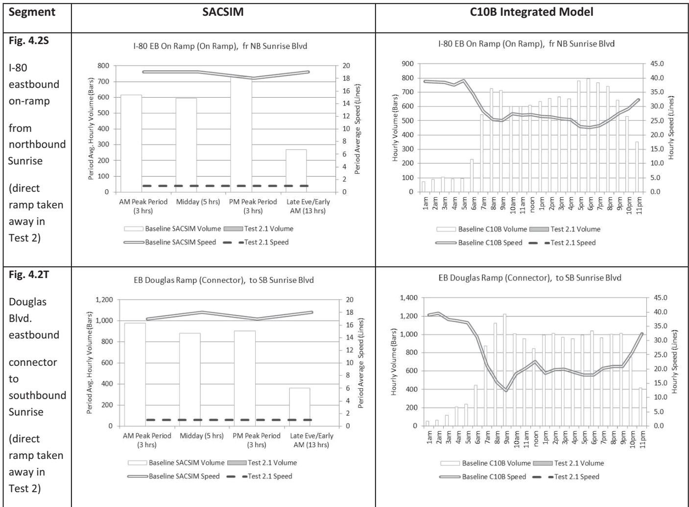
Figure 4.2. Vehicle volumes and speeds on key test segments—Test 2 (continued).
