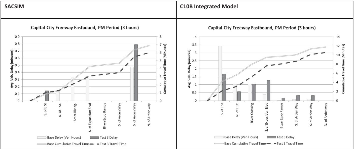
Figure 4.3. Travel time and average delay by segment, p.m. peak period—Test 3.
