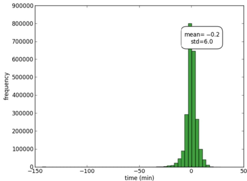
**Figure 3.7. Differences between static and dynamic travel times, a.m. peak period.**
