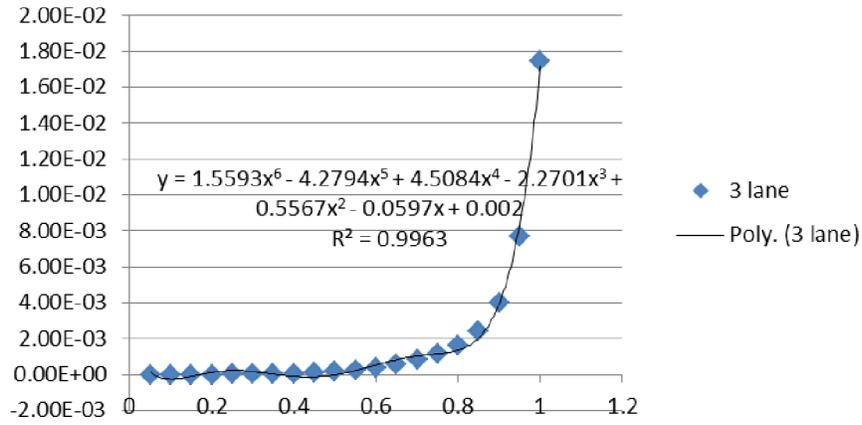
Figure 2.8. Incident delay for three-lane roadways.
