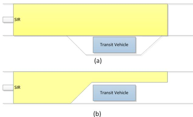
**Figure 2.3. SIR areas with (a) and without (b) bus pullouts.**
