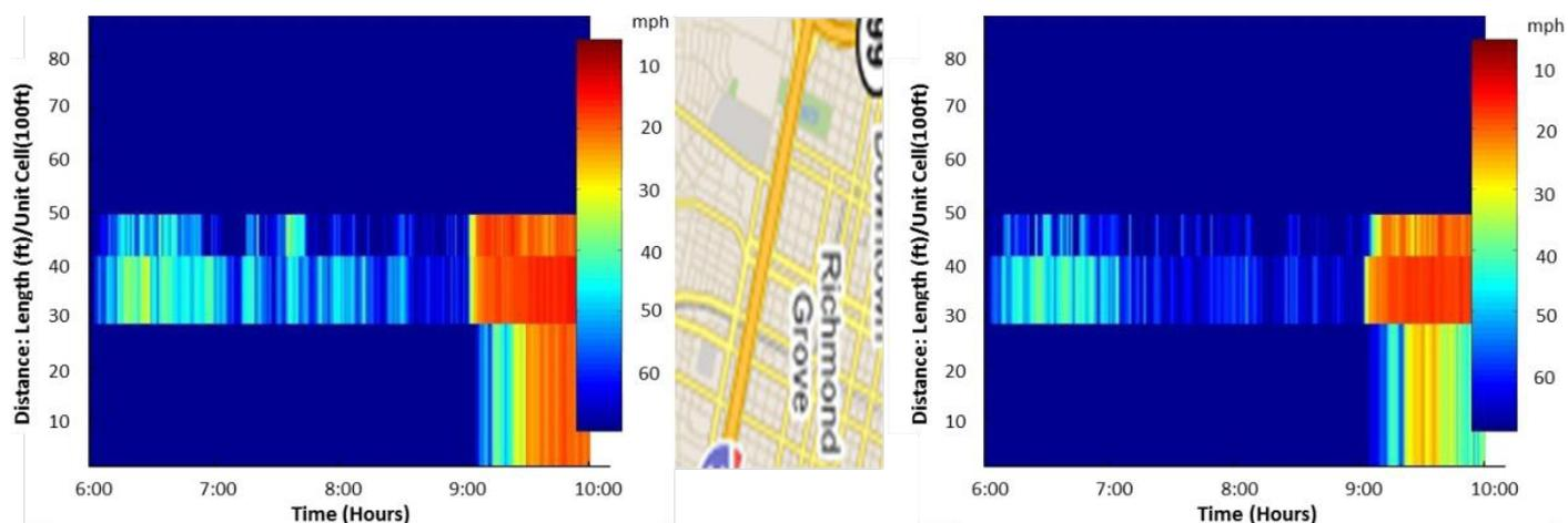
**Figure 3.11. Comparison of speeds between baseline (left) and improvement (right) scenarios.**
