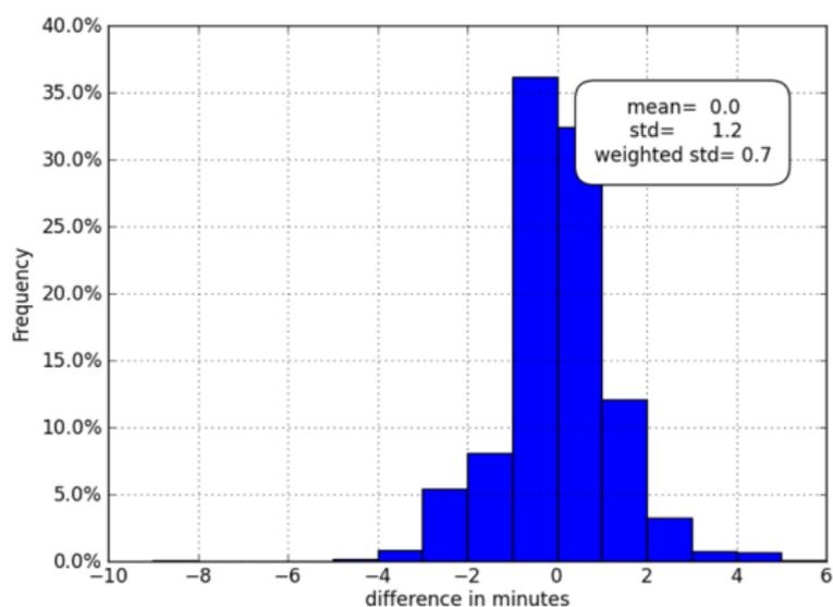
**Figure 3.3. Differences in mean travel times between Iterations 20 and 21, 8:00 a.m.**
