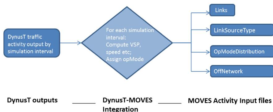
**Figure 2.10. Data flow and organization of MOVES and DynusT integration.**
