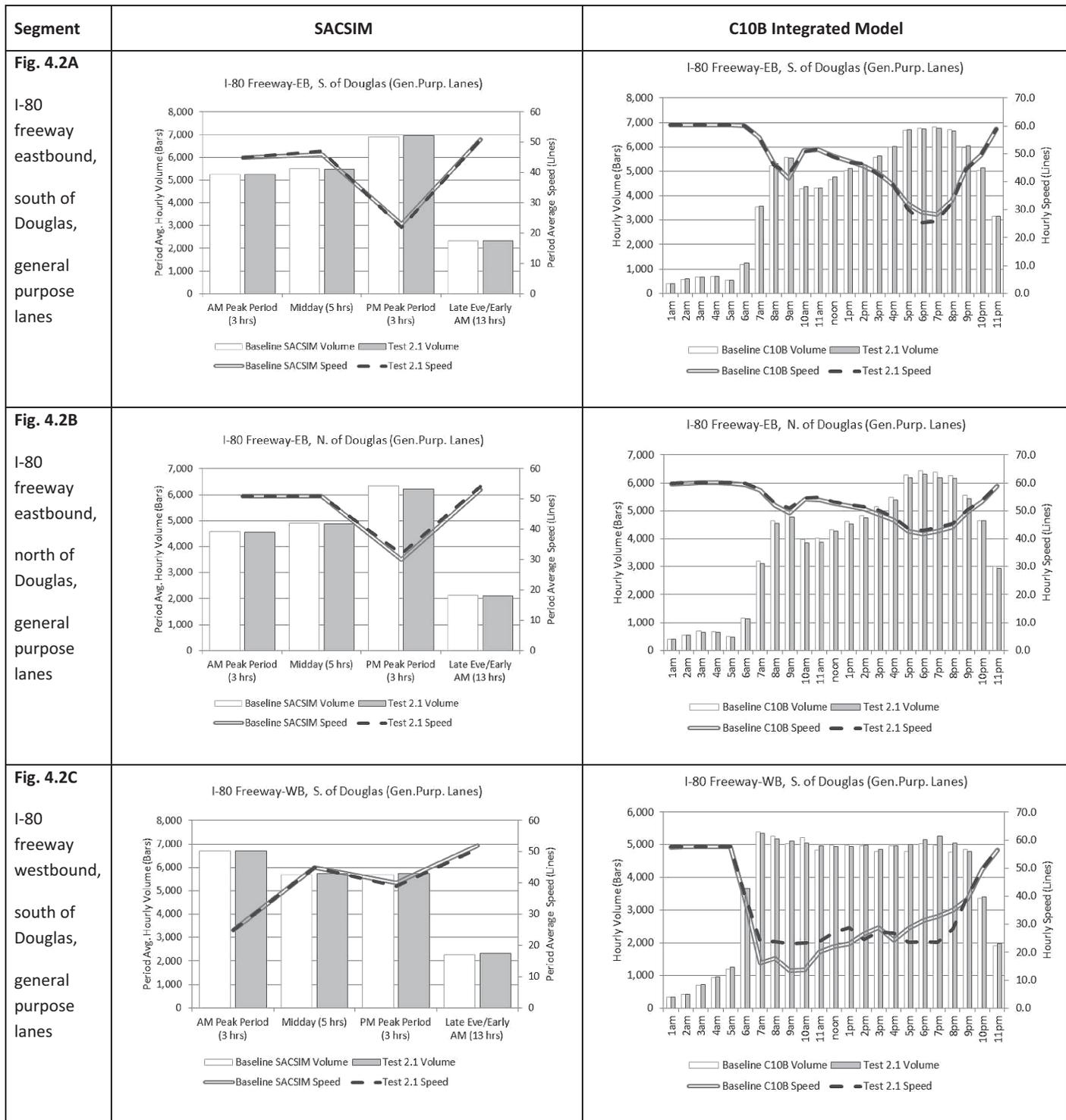
Figure 4.2. Vehicle volumes and speeds on key test segments—Test 2. (Continued on next page.)
