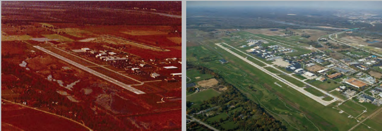
Aerial view of KSUS with wetland present left of AOA in the 1980s ( left ) replaced by specially drained and irrigated golf course ( right ) (Source: KSUS).
