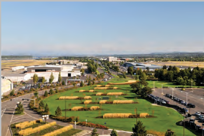
Goose deterrents at PDX. Raised vegetation berms ( left ) and silt fencing ( right ) (Source: Port of Portland).
