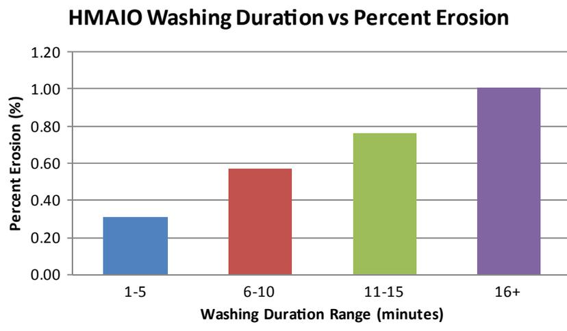
**Figure 4-11** Percent increase in degradation of ignition oven aggregate with increase in mechanical washing duration.
