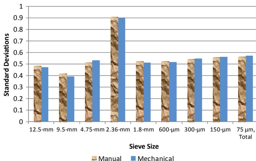
**Figure 4-6** Reproducibility standard deviations of percent passing various sieve sizes from manual and mechanical washing pooled from HMAIO 19-20, 21-22, 23-24, and 25-26 samples.
