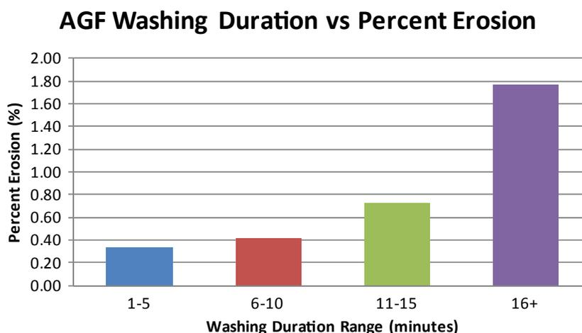
**Figure 4-9** Percent increase in degradation of fine aggregates with increase in mechanical washing duration.
