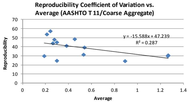
**Figure 3-3** Relationship between average and standard deviation and between average and coefficient of variation of percent material finer than a 75- $\mu\text{m}$  (No. 200) sieve by washing of AGC.
