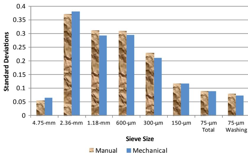
**Figure 4-3** Repeatability standard deviations of percent passing various sieve sizes after manual and mechanical washing pooled from AGF 171-172, AGF 175-176, and AGF 179-180 samples.
