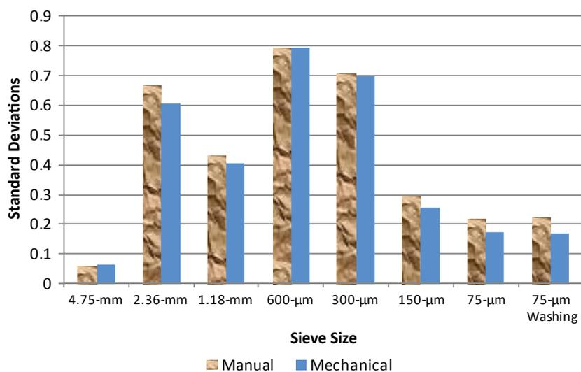
**Figure 4-4** Reproducibility standard deviations of percent passing various sieve sizes from manual and mechanical washing pooled from AGF 171-172, AGF 175-176, and AGF 179-180 samples.
