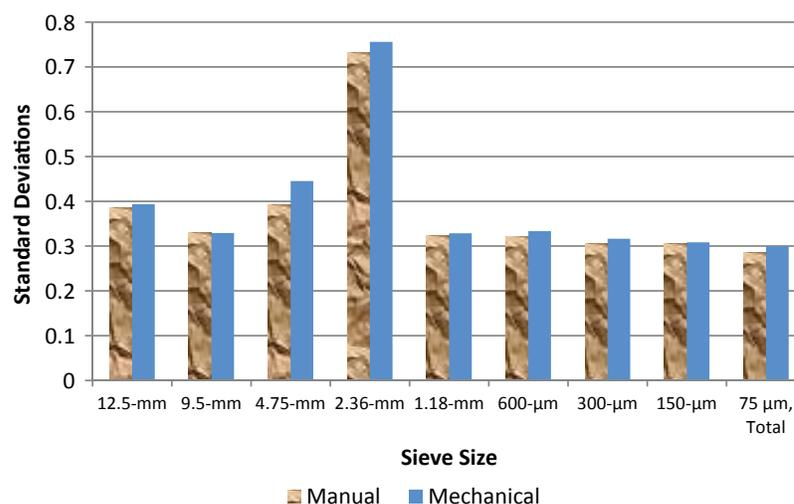
**Figure 4-5** Repeatability standard deviations of percent passing various sieve sizes from manual and mechanical washing pooled from HMAIO 19-20, 21-22, 23-24, and 25-26 samples.
