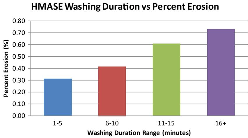
**Figure 4-12** Percent increase in degradation of solvent extracted aggregates with increase in mechanical washing duration.
