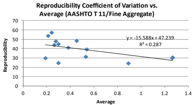
**Figure 3-4** Relationship between average and standard deviation and between average and coefficient of variation of percent material finer than a 75- $\mu\text{m}$  (No. 200) sieve by washing of AGF.
