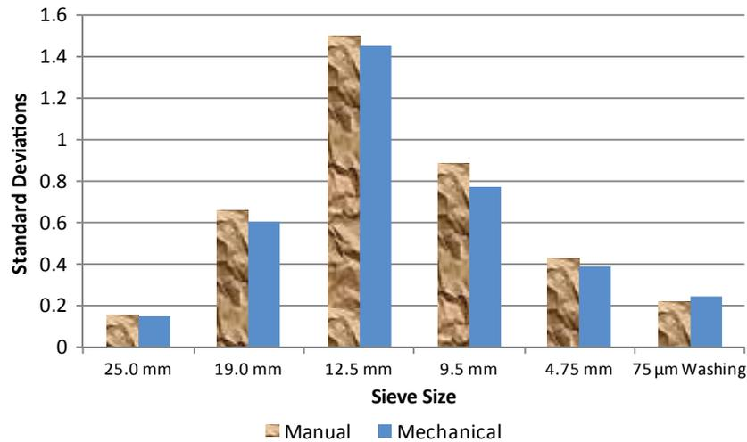
**Figure 4-2** Reproducibility standard deviations of percent passing various sieve sizes after manual and mechanical washing pooled from AGC 169-170, AGC 173-174, and AGC 177-178 samples.
