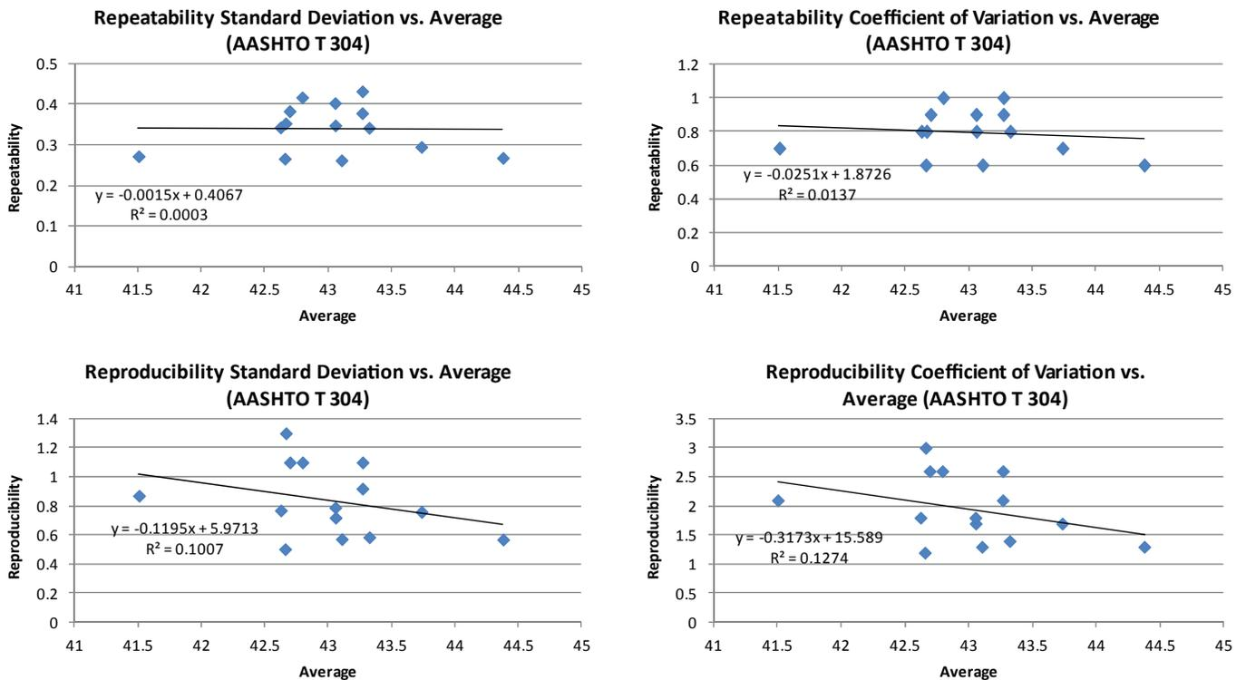
**Figure 3-2** Relationship between average and standard deviation and between average and coefficient of variation of the AASHTO T 304 data.
