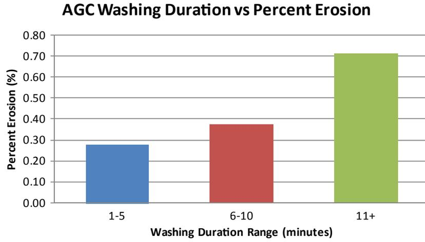
**Figure 4-10** Percent increase in degradation of coarse aggregates with increase in mechanical washing duration.
