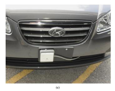
Figure 2.2. Instrumentation installed in vehicles: (a) head unit mounted behind rearview mirror containing four cameras, passive alcohol sensor, infrared illuminator, accelerometers, and GPS; (b) NextGen main unit with 128 GB SSD, power controller, and sensors mounted in trunk; and (c) forward radar mounted on front license plate holder.
