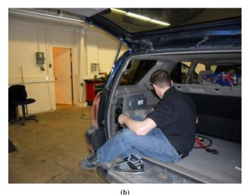
Figure 3.7. Installation of cabling from head unit to DAS NextGen computer in trunk: (a) kick panel on driver side removed and (b) connection of cabling to NextGen.
