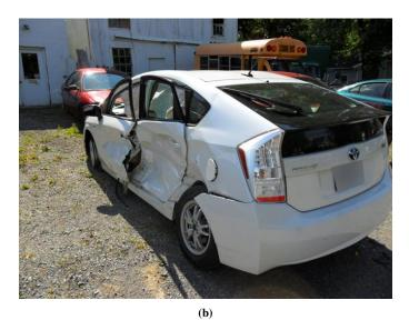
Figure 3.21. Examples of Level 1 and Level 2 crash damage sustained by NDS vehicles: (a) Level 1 crash with damage to vehicle, no airbag deployment and (b) Level 2 crash with damage to vehicle, airbag deployed.
