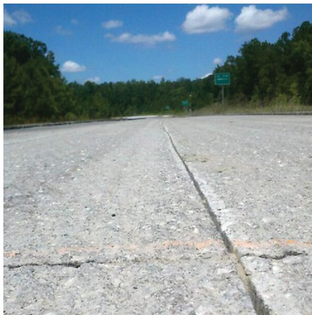
FIGURE 5 Saw-cut sections at NCAT Test Track to simulate structural cracking. (Source: Buzz Powell, NCAT.)
