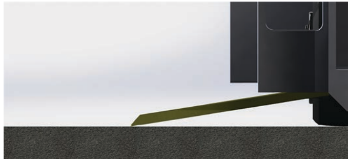
Figure 9. Ramp for vehicles with 1:6 slope.
