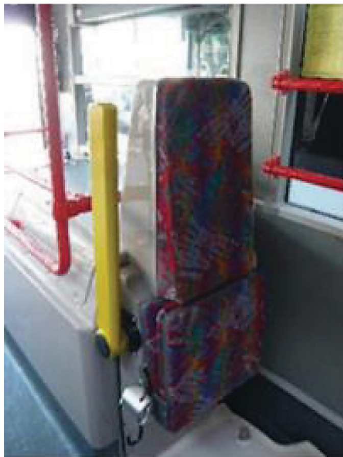
Figure 19. Rear facing on the curb side of bus with pivoting aisle arm rest to prevent tipping (BC Transit Canada).
