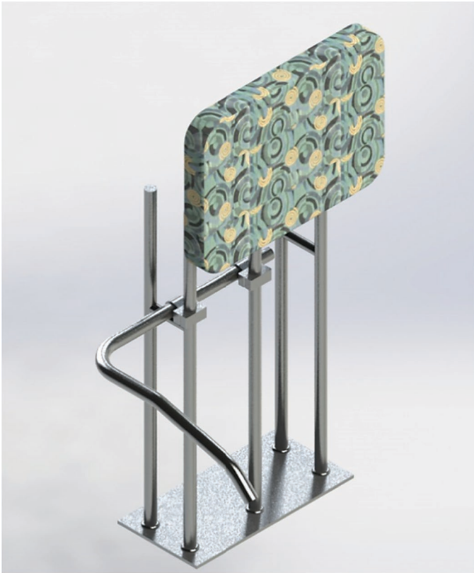
Figure 20. Extended width back panel and aisle side restraint for rear facing on BRT vehicles (center door loading).
