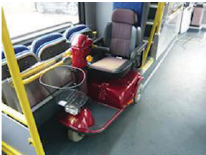
Figure 18. Example of rear facing on road side of bus (BC Transit, Canada).
