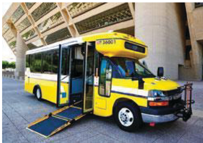
Figure 11. Bi Fold ramps on transit bus (DART) and low floor paratransit vehicle (ARBOC).
