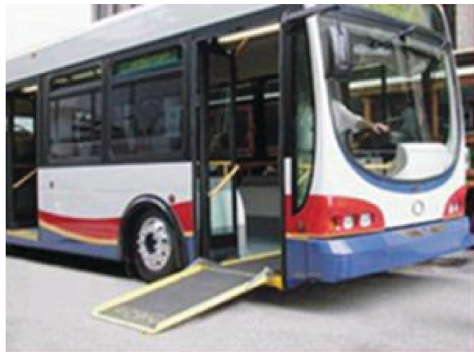
Single flip ramp, front door, kneeling bus at 7 inch height. Source: Rutenberg Design Inc.
