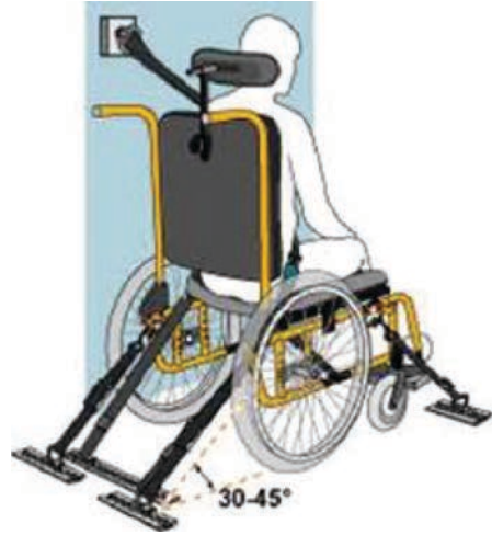
Figure 8. Forward facing four belt securement system [ www.travelsafer.org ].
