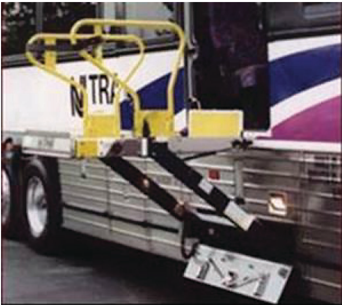
Figure 13. Wheelchair lift for intercity/OTRB high floor coach (NJ Transit).
