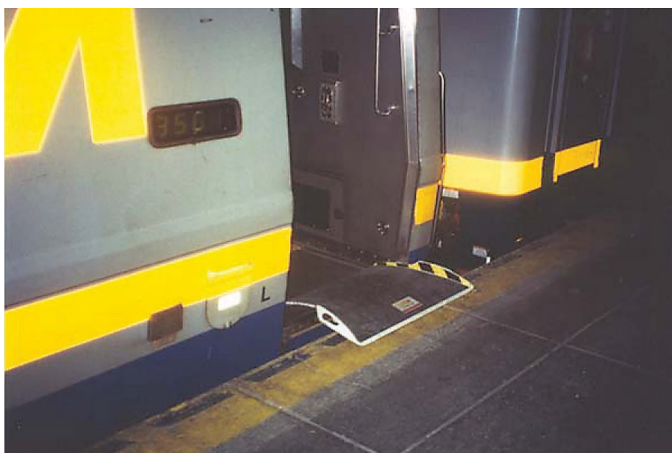
Figure 14. Manual bridge plate for use in rail cars (VIA Rail Canada).
