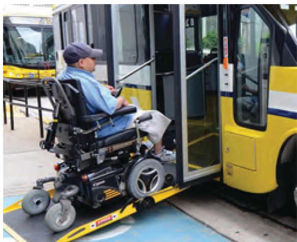
Figure 11. Bi Fold ramps on transit bus (DART) and low floor paratransit vehicle (ARBOC).
