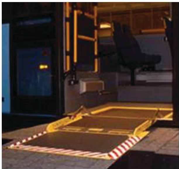
Bi-fold ramp for low floor bus, extended ramp length, Ricon Corp Source: Ricon Corporation.
