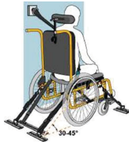
Figure 15. Forward facing securement with four belt securement [Source: www.travelsafer.org/ ].
