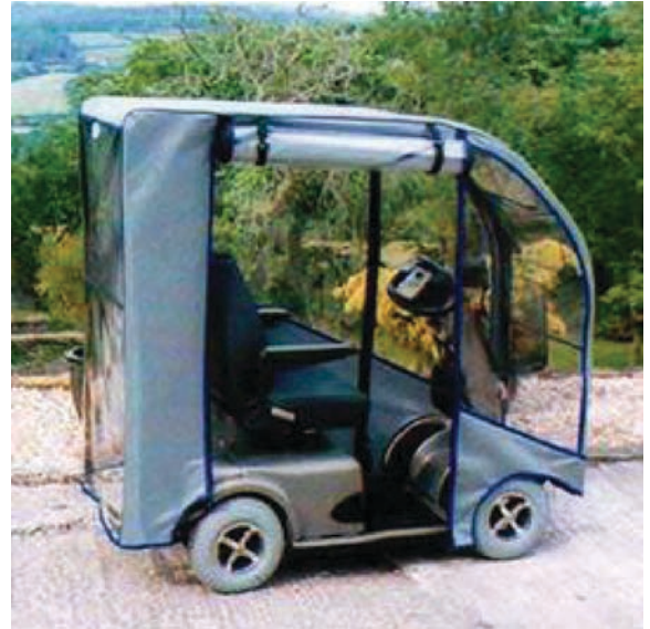
Figure 1. 3- and 4-wheeled mobility devices designed for outdoor use only. (Source: X-Treme Scooters; http://electricbikeandscooterstore.com/ebssxtreme420.htm .)
