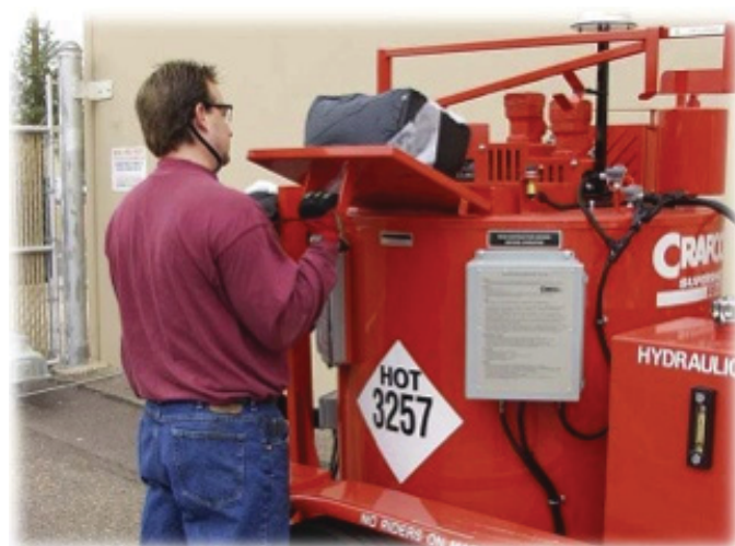
Photograph 4-12. Loading Crafcro melter (courtesy Crafcro).
