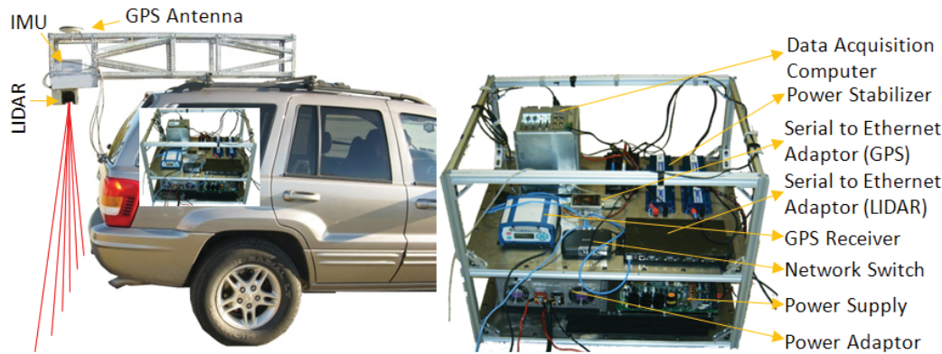
Figure 12. Instrumented vehicle data collection system.
