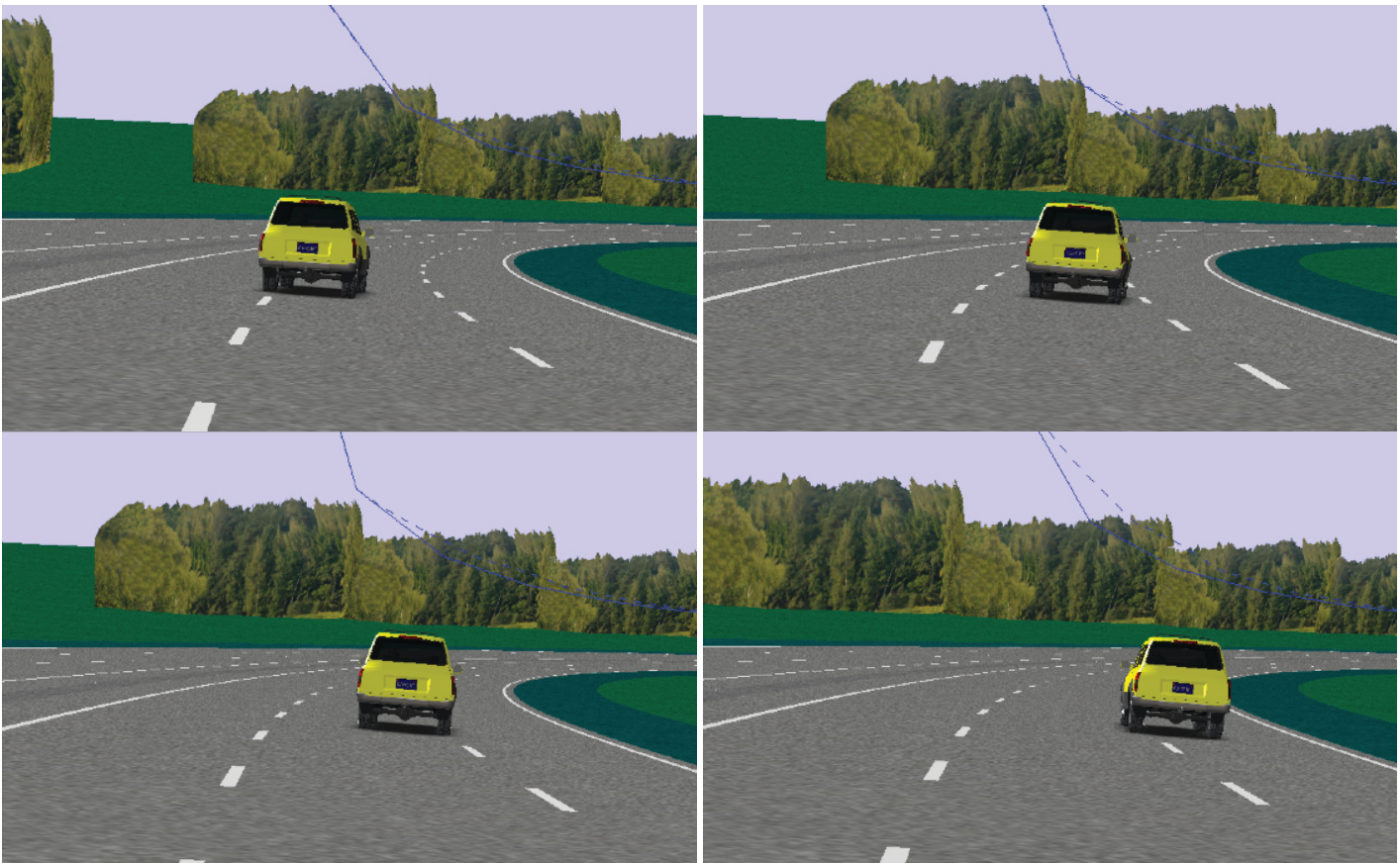
Figure 103. Three-dimensional rendering of simulated road within CarSim/TruckSim; situation shows an E-class SUV skidding while changing lanes and emergency braking.
