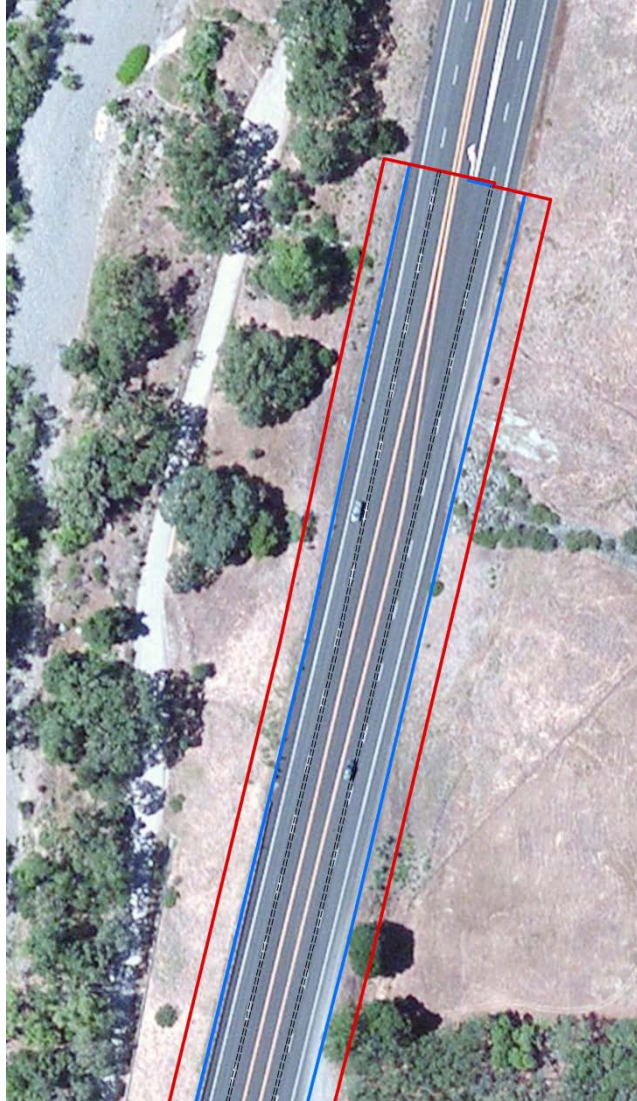
Figure 2.1. An example of how buffers are used to estimate the extent of impact from a new project. Black dotted lines represent road centerlines, blue lines represent the edges of existing roads, and red lines are the estimated buffered impacts.
