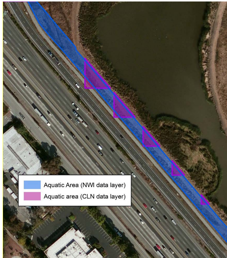
Figure 3.4. A section of Highway 101 in District 4 showing aquatic impacts from the NWI (freshwater emergent wetland) and CLN (water, permanent freshwater marsh) layers. Nonaquatic areas in the CLN layer that overlap are classified as urban.
