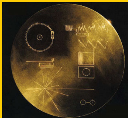
Visual information can be essential to understanding—as on the etched gold aluminum covers of the "Sounds of Earth" records aboard the Voyager probes, the farthest human-made objects from Earth. The etchings offer a pictorial key to playing the record.
