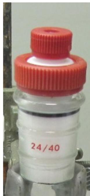
**Figure A-6.** Detail of liquid addition/septum closure fitting with septum installed (not visible). Note that this is a friction fit closure of the vessel.
