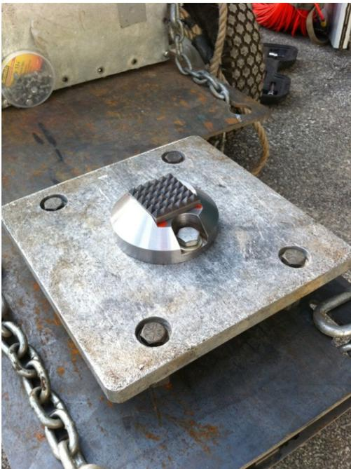
**Figure 3.13.** Ground coupler base late for MicroVib.
