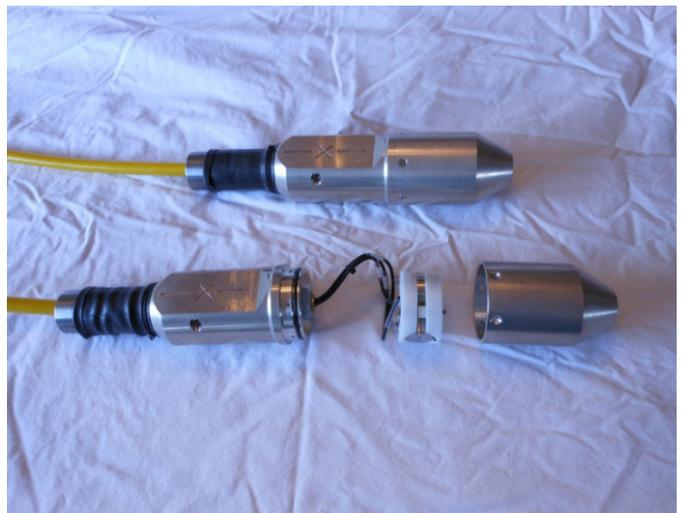
**Figure 3.14.** Housing probe and triaxial accelerometers.
