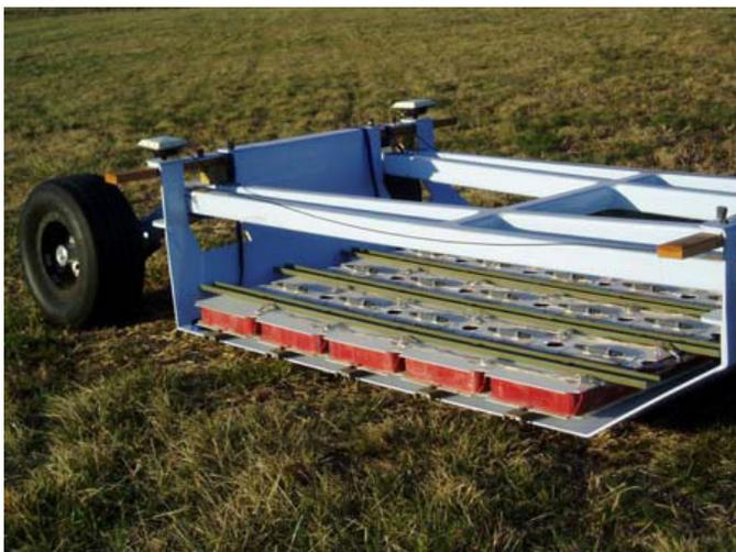
**Figure 2.5. SAIC/NRL TDEMI array for buried-object location and classification.**
