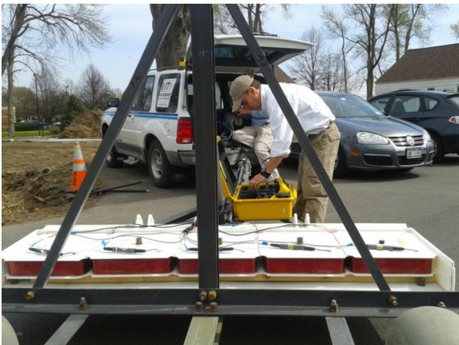
Figure 3.73. Configuration and testing of the 5-by-1 TDEMI sensor array on UIT’s metal-free trailer.
