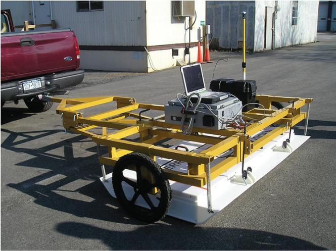
**Figure 2.1.** *UIT's Multichannel GPR system, the TerraVision II.*
