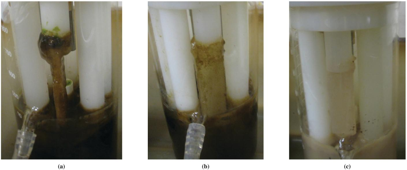
Figure 5-6. Close-up views of reactor rods at the conclusion of the experiment, Day 28. ([a] 25 percent full sunlight, [b] 12 percent full sunlight, and [c] dark.)
