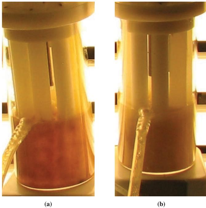
**Figure 5-12. Reactor appearance at Day 28. ([a] Nitrogen-varied reactor and [b] Phosphorus-varied reactor.)**
