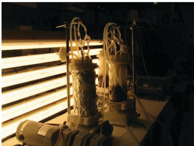
**Figure 4-4. Biofilm growth reactors in dark, at 12 percent full sunlight, and at 25 percent full sunlight.**
