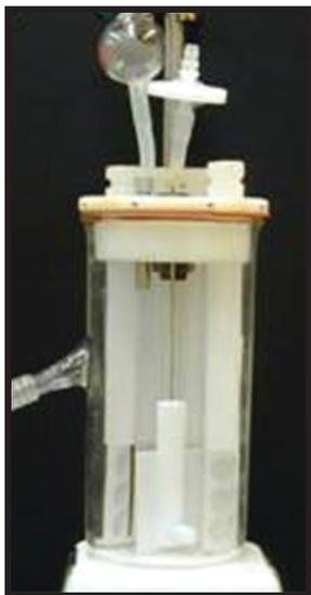
**Figure 4-3.** CDC biofilm reactor.
