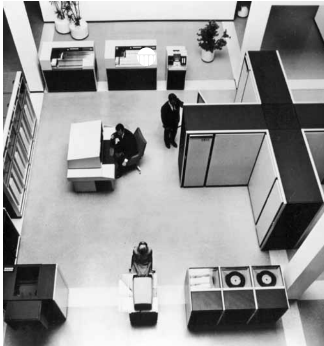
The elegant CDC 6600, with its plus-sign shaped panels, held the supercomputer speed record from 1964 to 1969.
