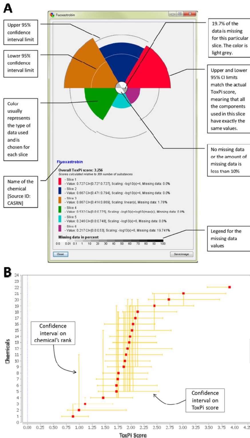
FIGURE C-4 ToxPi confidence intervals. A: Uncertainty in size of each slice. B: Confidence intervals in overall ToxPi score and relative rank of each compound.
