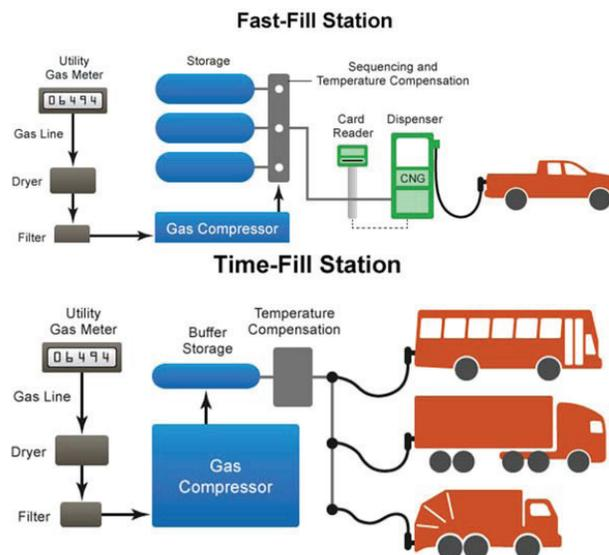
FIGURE 5-6 Conceptual diagram of compressed natural gas filling stations. SOURCE: [http://www.afdc.energy.gov/fuels/natural\\_gas.html](http://www.afdc.energy.gov/fuels/natural_gas.html).
