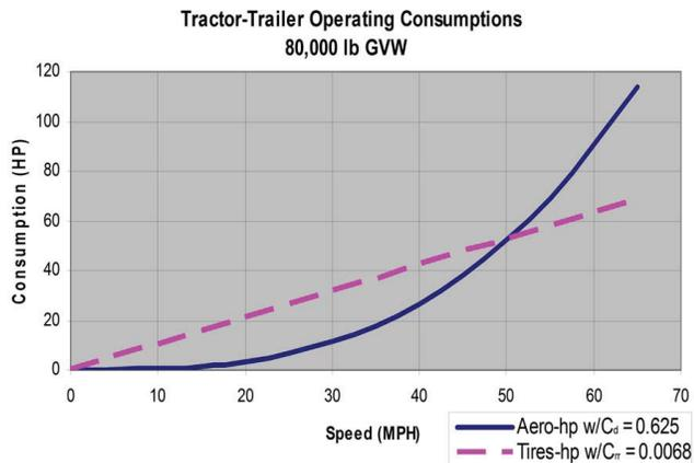
FIGURE 6-2 Aerodynamics and tire power consumption for a late-model tractor-trailer combination with GVW of 80,000 lb. SOURCE: NRC, 2012, Figure 5-1.
