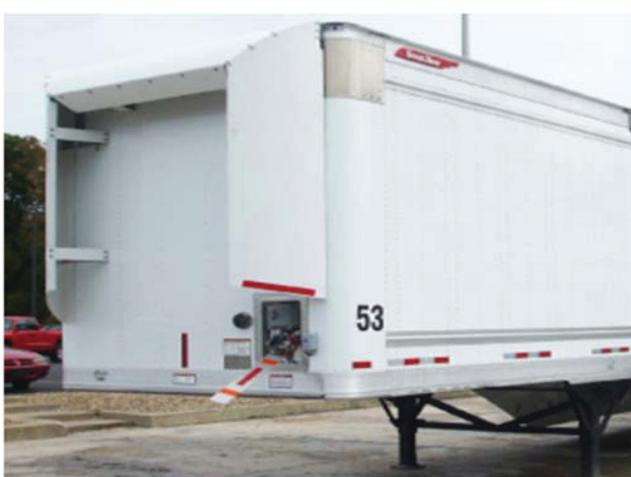
FIGURE 6-6 Trailer front gap fairing. SOURCE: Freight Wing. Available at [http://www.freightwing.com/gap\\_fairing.php](http://www.freightwing.com/gap_fairing.php). Accessed November 14, 2013.
