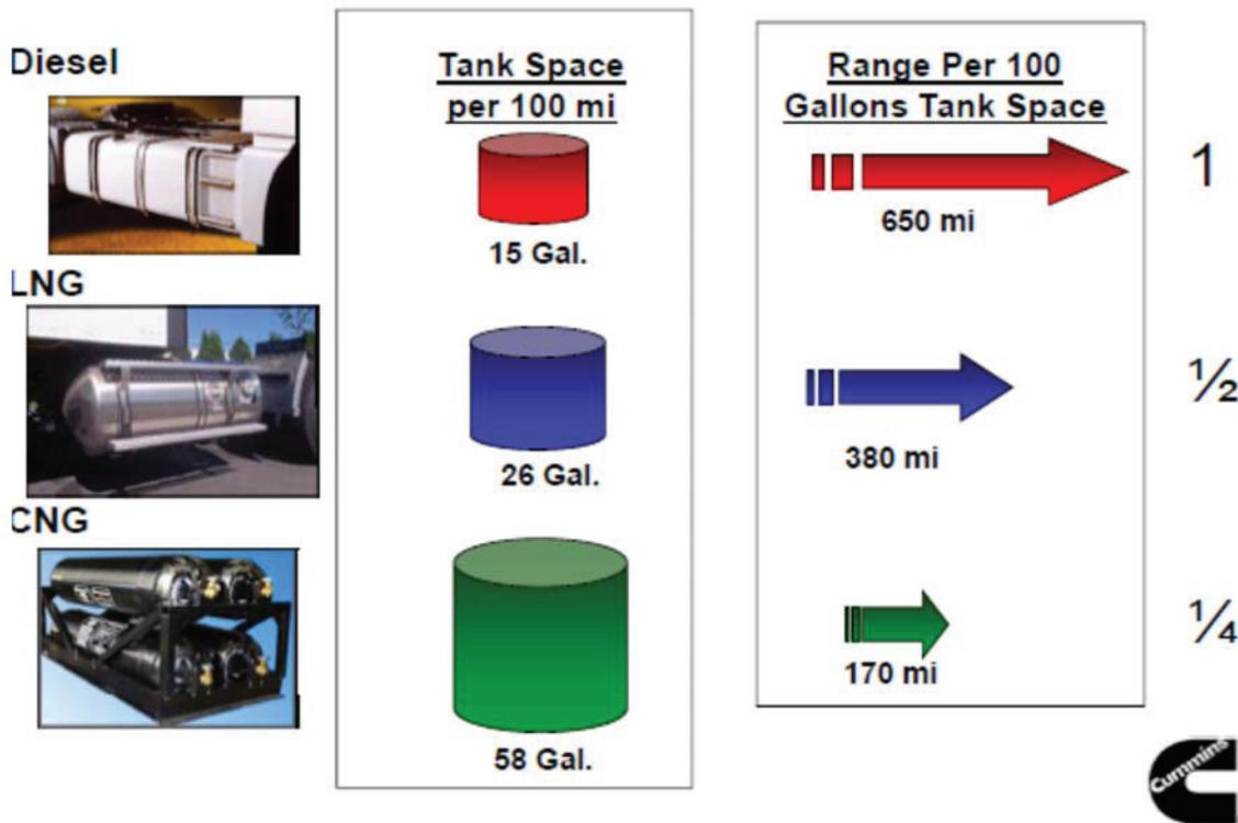
FIGURE 5-3 Comparison of diesel and NG fuel tanks. SOURCE: John Wall, Cummins, Inc., “Opportunities and barriers for natural gas: Expanding natural gas in transportation,” Presentation to the Board on Energy and Environmental Systems on September 11, 2012.
