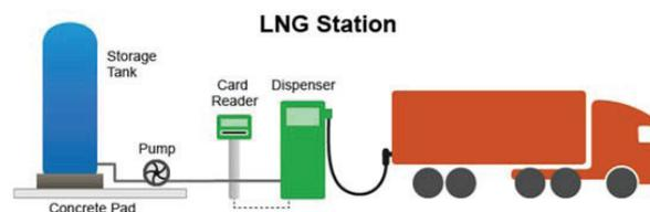
FIGURE 5-7 Conceptual diagram of LNG filling stations. SOURCE: [http://www.afdc.energy.gov/fuels/natural\\_gas.html](http://www.afdc.energy.gov/fuels/natural_gas.html).
