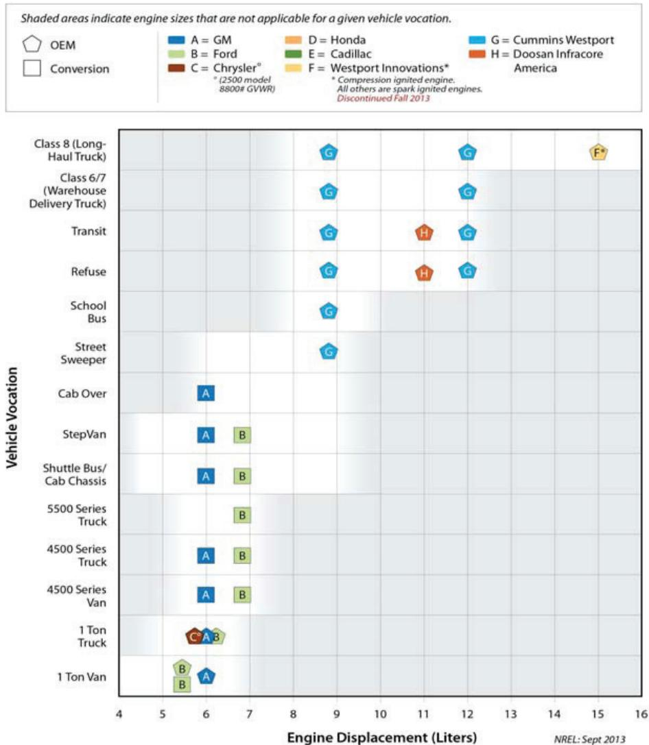
FIGURE 5-4 Available natural gas vehicles and OEM-authorized conversions. SOURCE: NREL.
