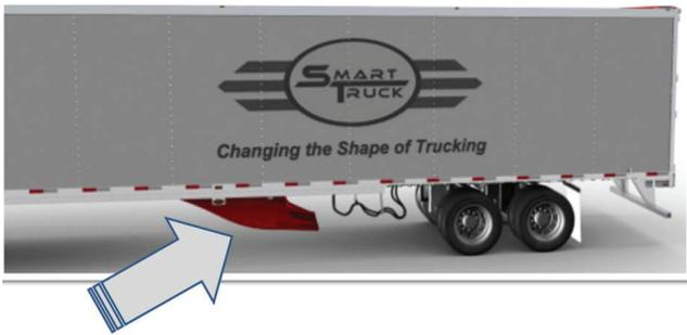
FIGURE 6-8 SmartTruck undertray: UT-1. Available at <http://smarttrucksystems.com/undertray-UT1Base.php>. Accessed November 14, 2013.
