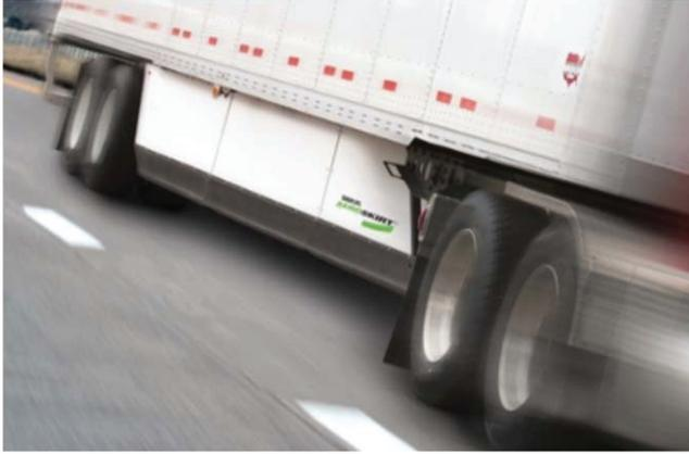
FIGURE 6-7 Wabash trailer skirt. Available at <http://wabash-composites.com/compositeshome/products/trailer-side-skirts/duraplate-aeroskirt-for-truckload-applications>. Accessed November 14, 2013.
