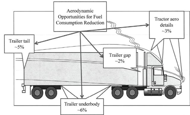
FIGURE 6-3 Tractor-trailer combination truck illustrating regions of potential fuel consumption reduction; combined  $C_d$  base of 0.625. SOURCE: NRC, 2010, Figure 5-8.
