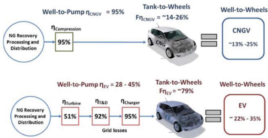
FIGURE 5-8 Comparison of efficiencies of compressed natural gas vehicles (CNGVs) and battery electric vehicles (BEVs). SOURCE: Curran, 2013.
