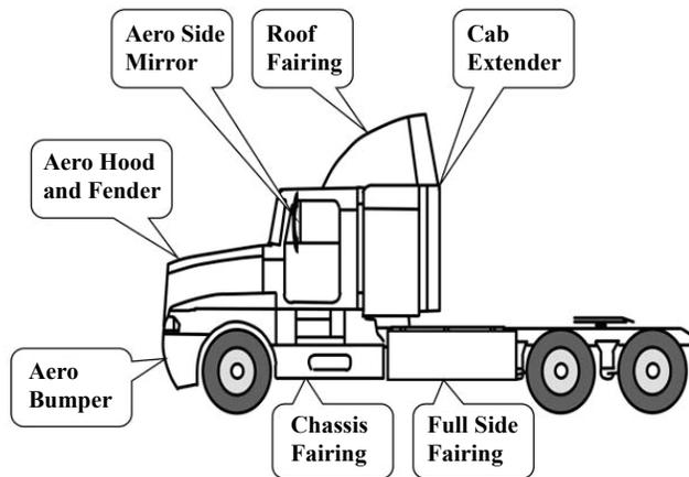
FIGURE 6-4 Sleeper tractor with aerodynamic features identified. SOURCE: NRC, 2010, Figure 5-5.
