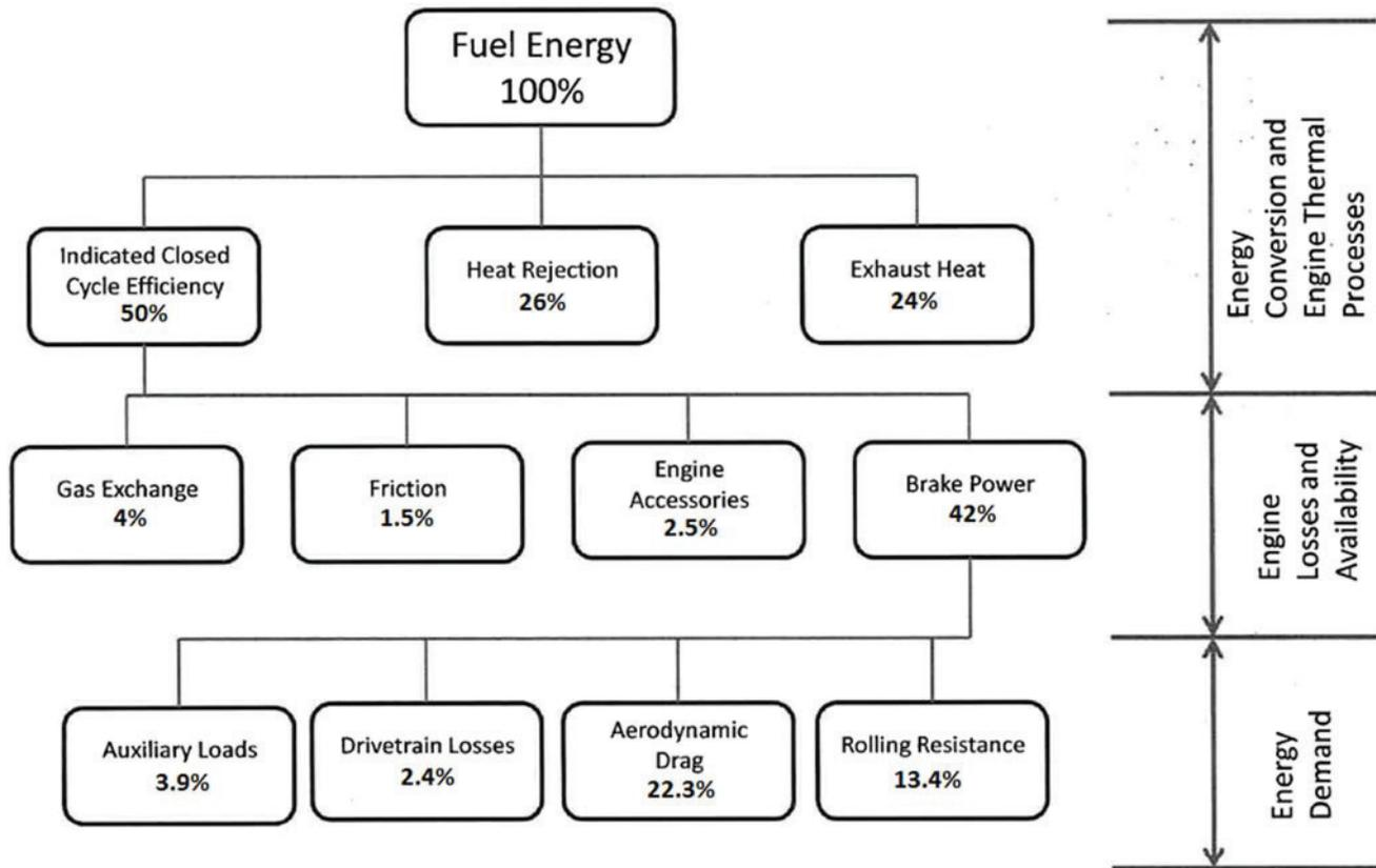
FIGURE 6-1 Energy balance of a fully loaded Class 8 tractor-trailer on a level road at 65 mph. SOURCE: NRC (2010), Figure 5-1.
