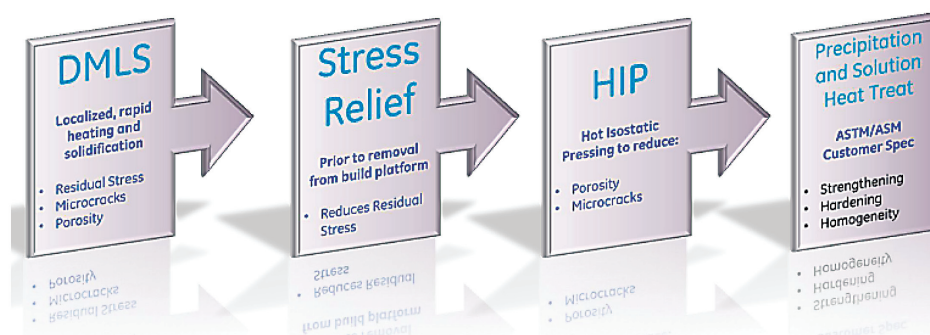
FIGURE 1 Processing steps needed to create a structural material. SOURCE: Courtesy of Dale Carlson, GE Aviation. Slide no. 6.
