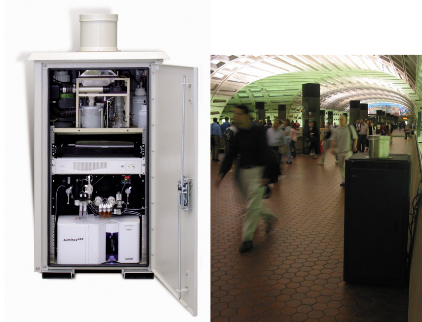
FIGURE G-2 Autonomous pathogen detector system.
