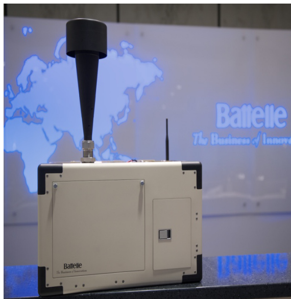
FIGURE H-7 Battelle’s Resource Effective Bio-Identification System (REBS) provides collector, detector, and identifier functions within a single, portable system.
