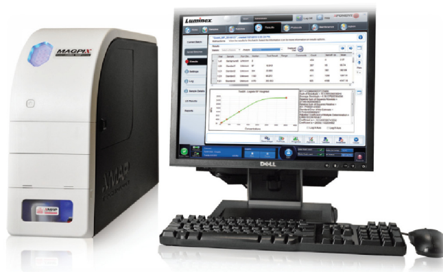
FIGURE H-4 Image of the complete MagPix system with computer interface.
