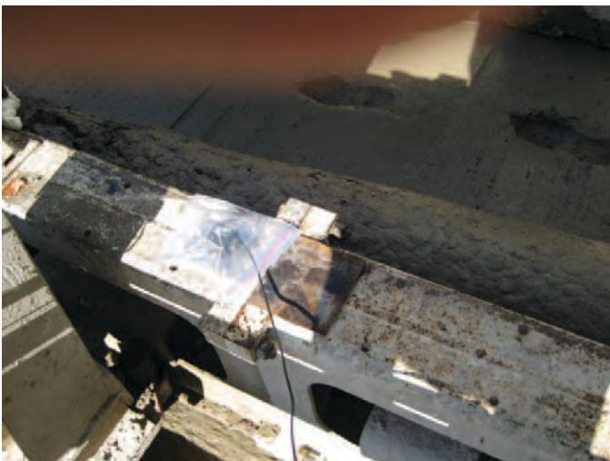
Figure 2.55. Inertia-Link mounted to the OCB.
