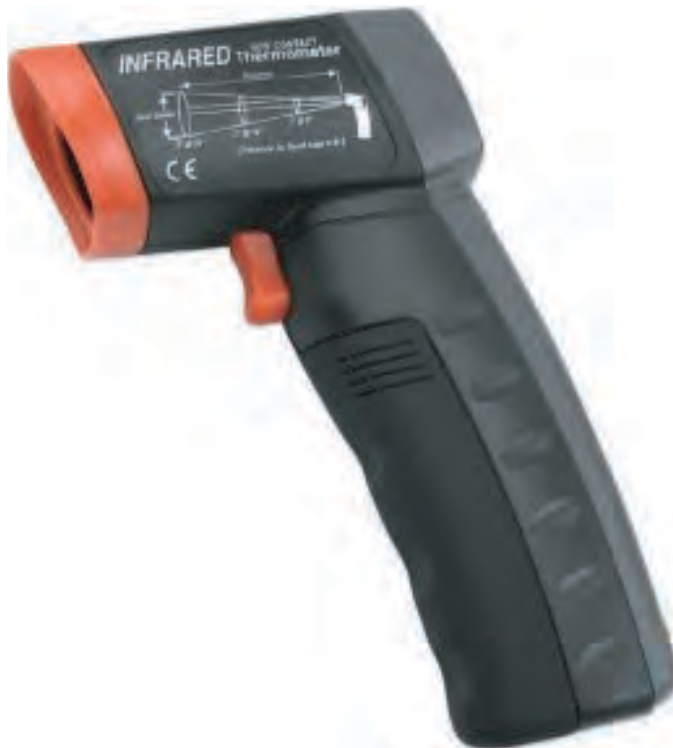
Figure C.3. Noncontact infrared thermometer for pavement surface temperatures. The manufacturer is Neiko.
