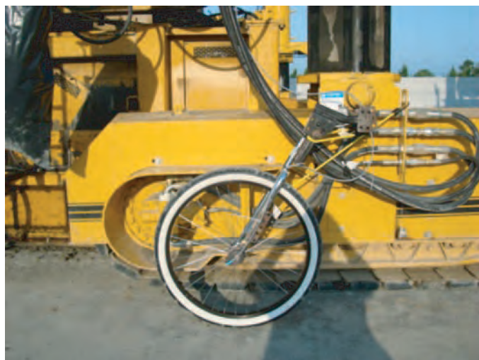
Figure 2.23. Fifth wheel mounted to the paver.
