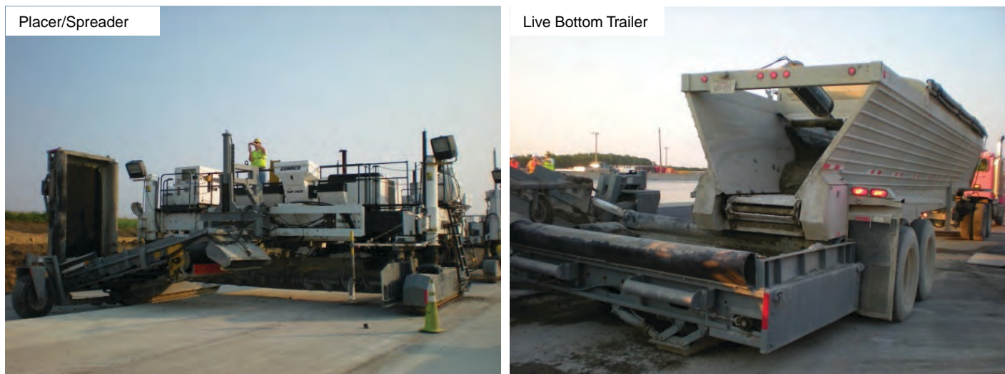
Figure 2.49. Belt placer/spreader used for concrete placement and live bottom trailer.
