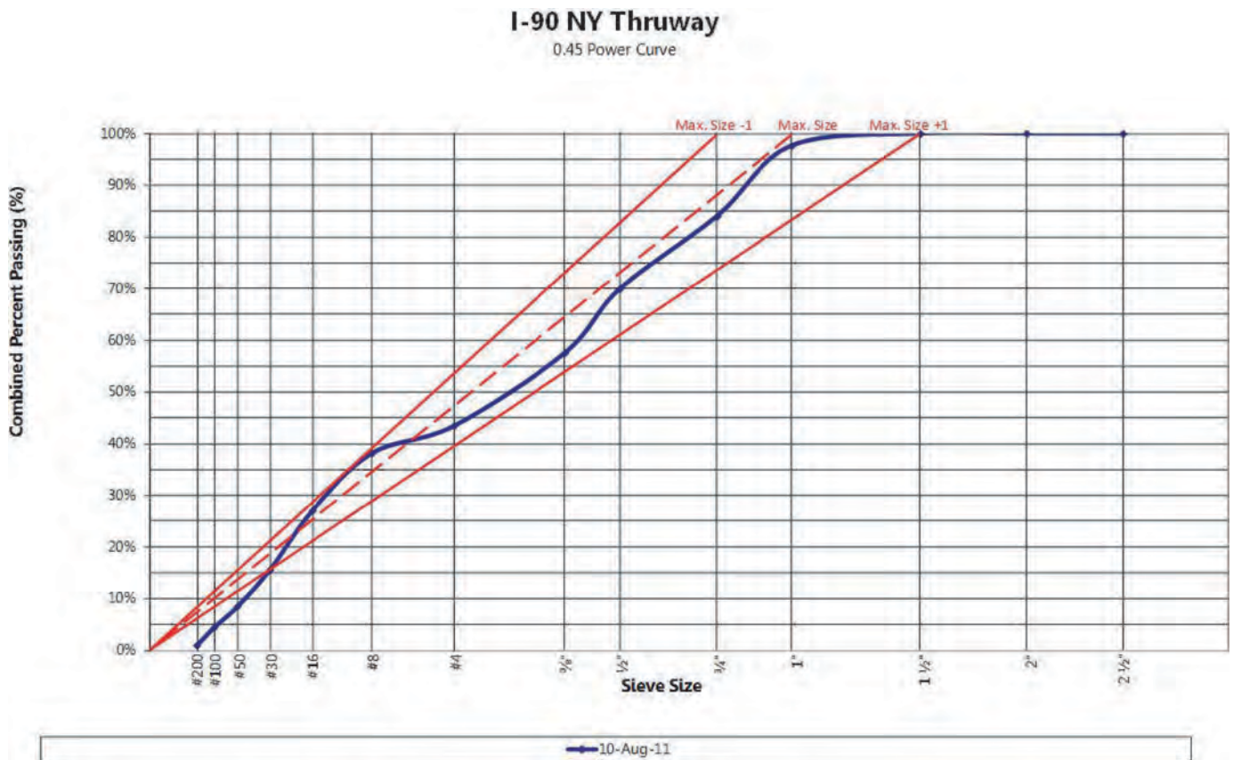
Figure G.25. Combined percent retained on individual sieves for New York site.
