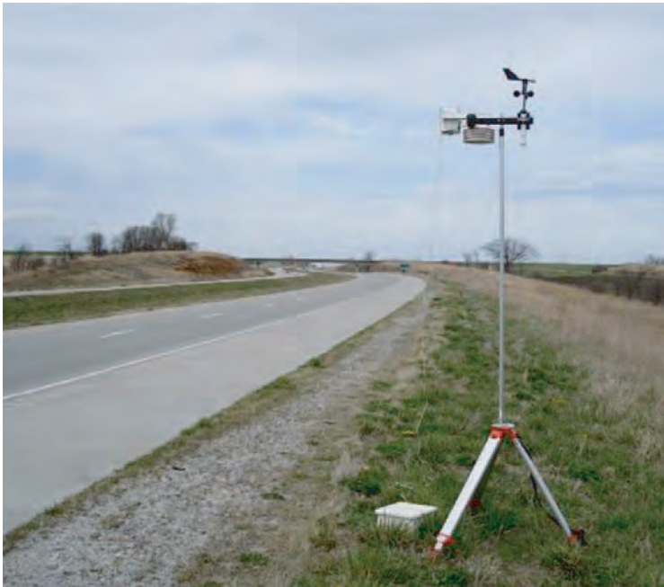
Figure C.2. Portable weather station.
