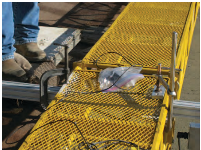
Figure 2.56. Inertia-Link mounted to the profiler bridge.
