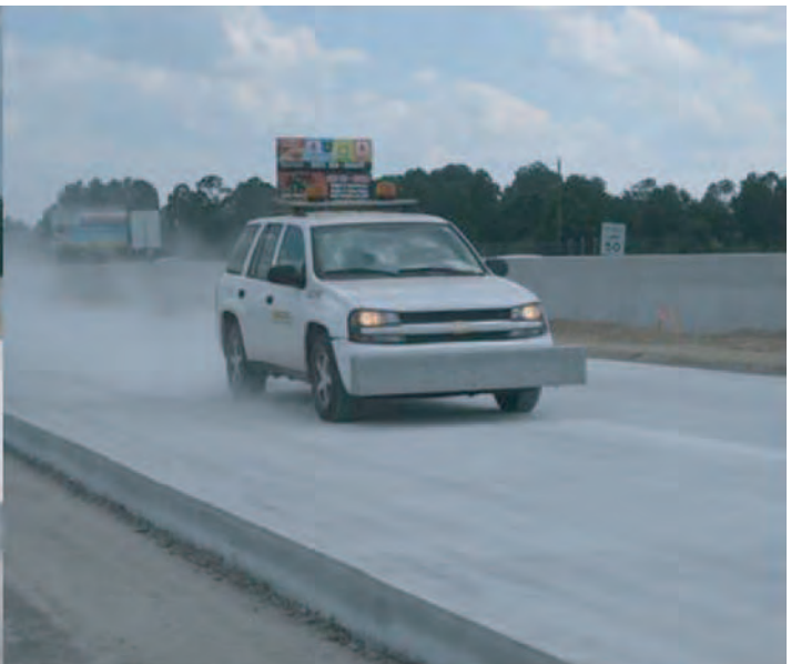
Figure 2.17. Hardened concrete measurements with SurPRO 2000 reference profiler (left) and the Georgia DOT high-speed inertial profiler (right).
