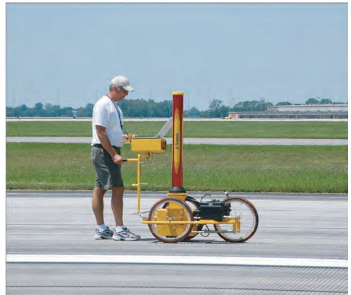
Figure 2.5. APR Auto Rod & Level.
