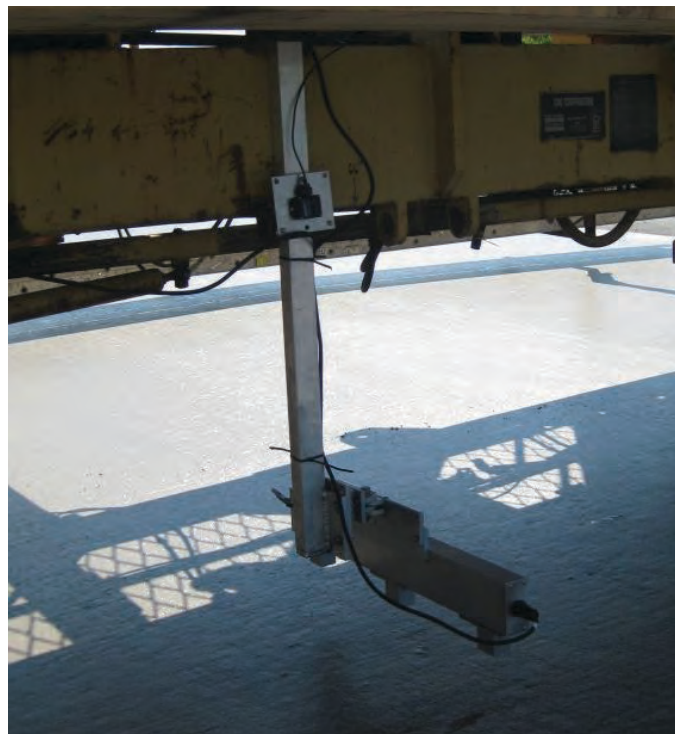
Figure 2.71. Location of Inertia-Link sensor on bridge-mounted Ames Engineering RTP.
