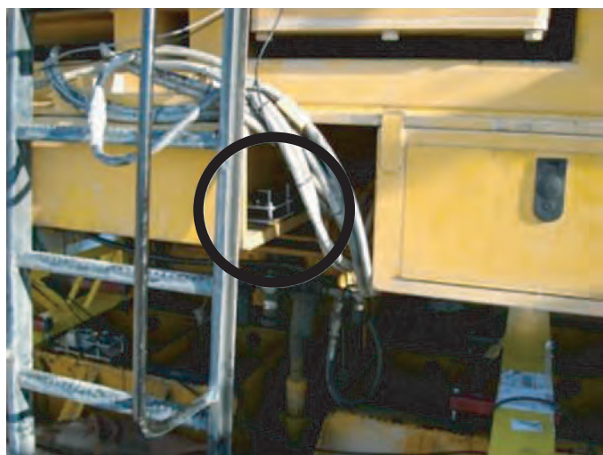
Figure 2.26. IMU sensor above the finishing pan on the paver.
