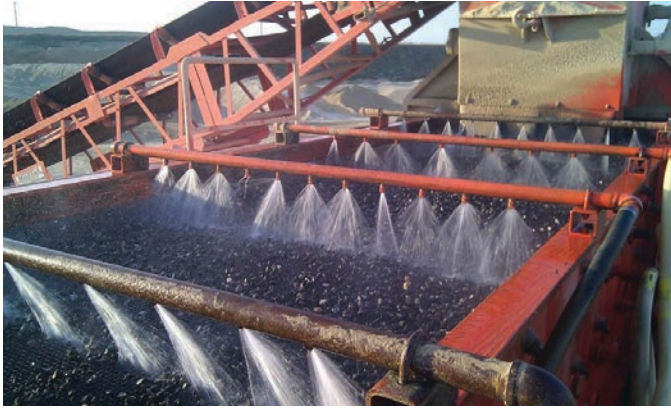
Figure 2.39. Fractionating, cleaning, and washing the RAP for use in the PCC mix.
