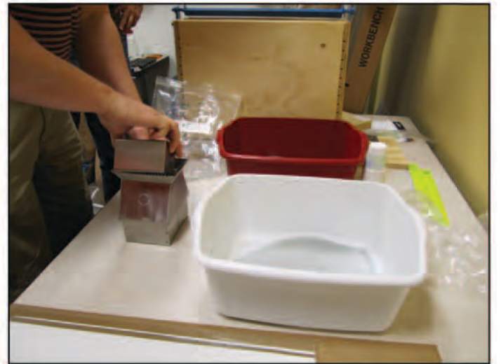
Using a 16:1 splitter to get a 3-pound sample and a 1:1 splitter for drawdown sample size.
