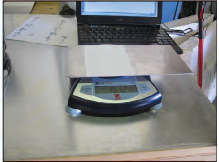
Calibrating the striper using a scale to ensure a delivered thickness of 15 mil wet.
