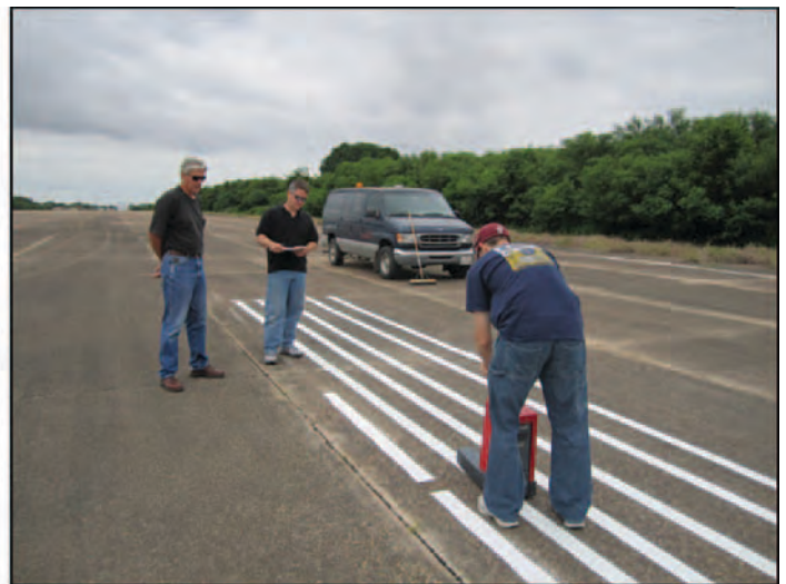
Placing two 20-foot stripes for each of the 5 bead packages. Measuring retroreflectivity after 24 hours.
