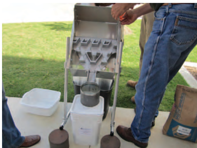
Figure 67. Large splitter 16:1 (left) and small splitter 1:1 (right).
