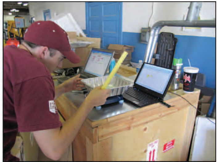
Using a scale to calibrate bead delivery rate to 8 pounds per gallon.
