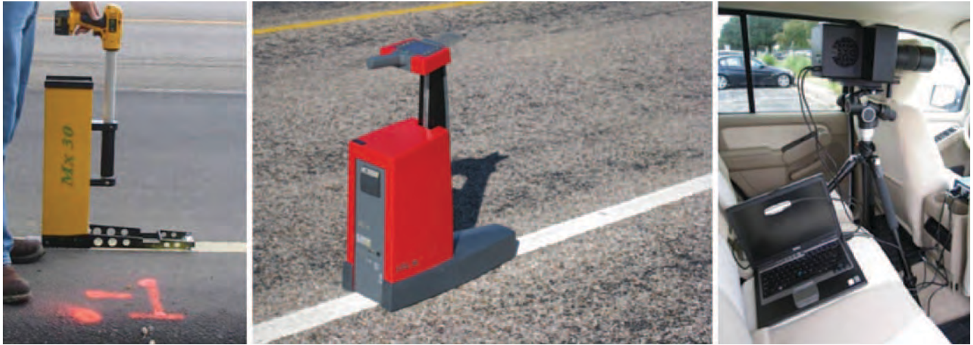
Figure 12. Pavement marking evaluation equipment.
