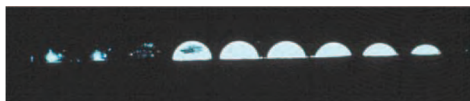
Figure 3. Glass bead embedment depth retroreflectivity comparison (Texas DOT 2004).
