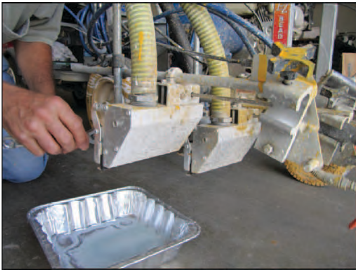
Using a scale to calibrate bead delivery rate to 8 pounds per gallon.
