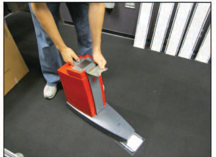
Delivering paint on the sample plate and measuring retroreflectivity after 24 hours.
