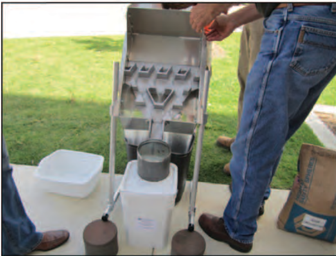
Using a 16:1 splitter to get a 3-pound sample and a 1:1 splitter for drawdown sample size.
