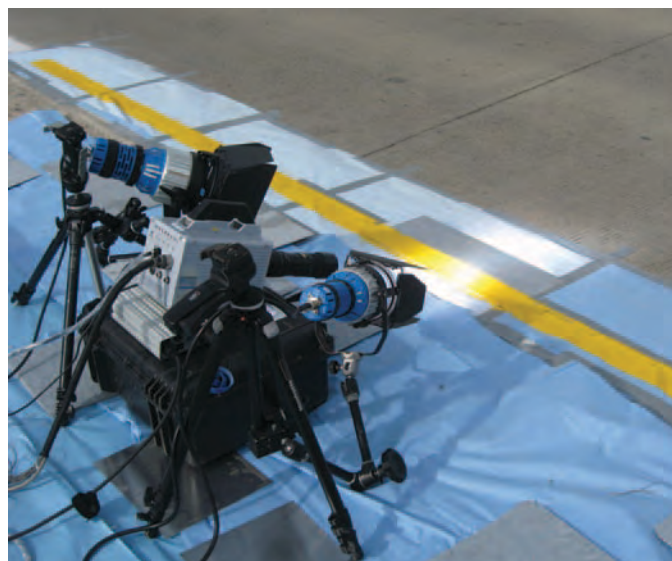
Figure 4. High-speed camera setup on side of roadway.
