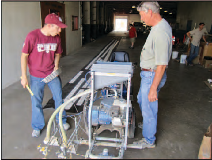
Calibrating the striper using a scale to ensure a delivered thickness of 15 mil wet.
