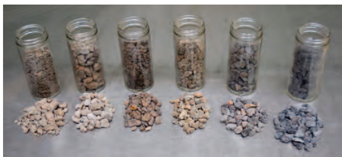
Figure 1. Lightweight aggregates (from left to right): CL1, SH1, SH2, CL2, SH3, and SL1.
