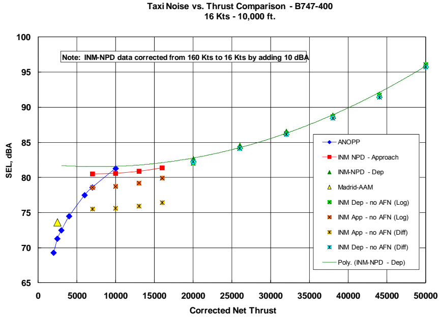
FIGURE E-15 Taxi noise vs. thrust comparison, B747-400 PW4096 for 16 knots at 10000 ft. distance.
