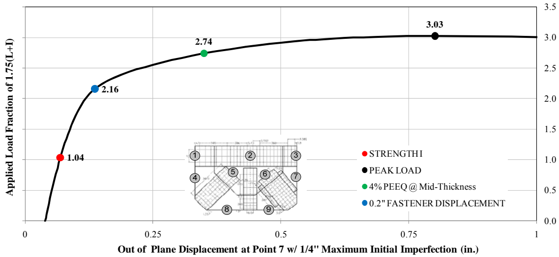
Figure 20. Plot of out-of-plane displacement motion of Point 7 versus the ALF.
