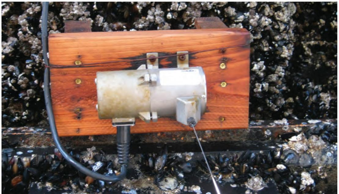
Closeup of linear motion transducer installed in Seattle.
