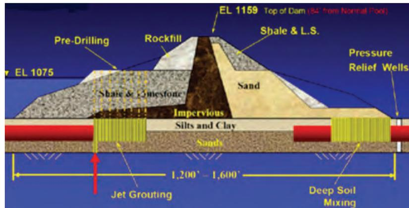
FIGURE 4 (above) Tuttle Creek Dam Project cross section, showing original remedial action to address deformation and drainage (EL = elevation, in feet).
