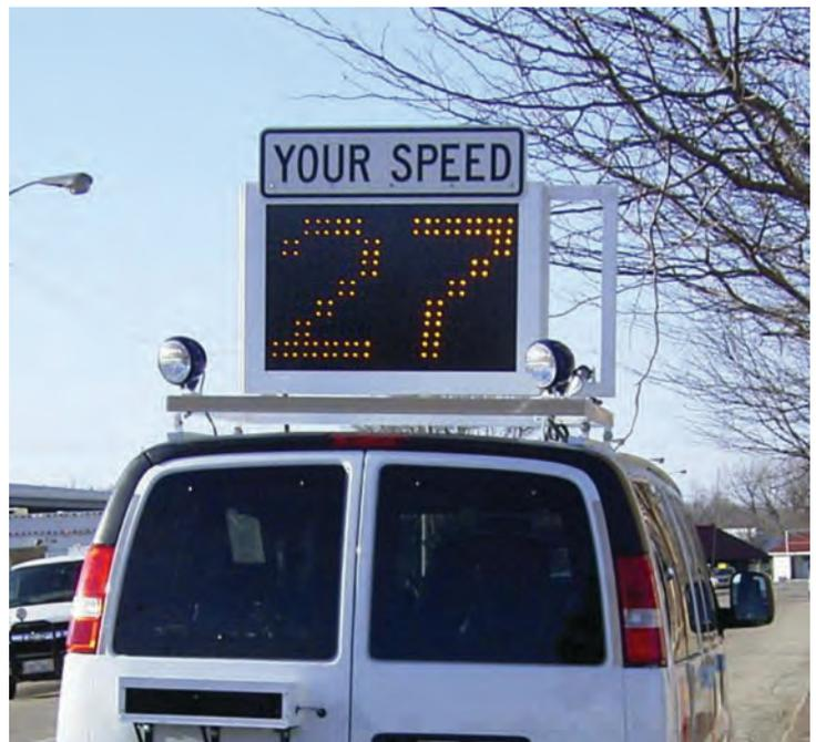
Figure 20. Example of motorist notification signing used with the Illinois work zone automated speed enforcement program.
