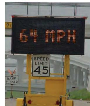
(b) Radar-Activated Portable Changeable Message Sign
