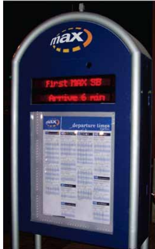
FIGURE 25 KCATA MAX (BRT service) DMS (Courtesy: TranSystems 2005).
