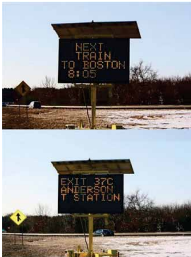
FIGURE 13 I-93 southbound VMS displaying next train departure time (19).
