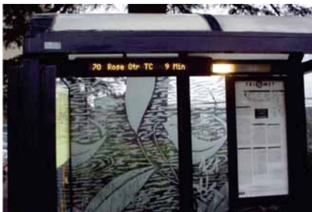
FIGURE 46 Single-line LED DMS in TriMet bus shelter (Courtesy: TriMet).
