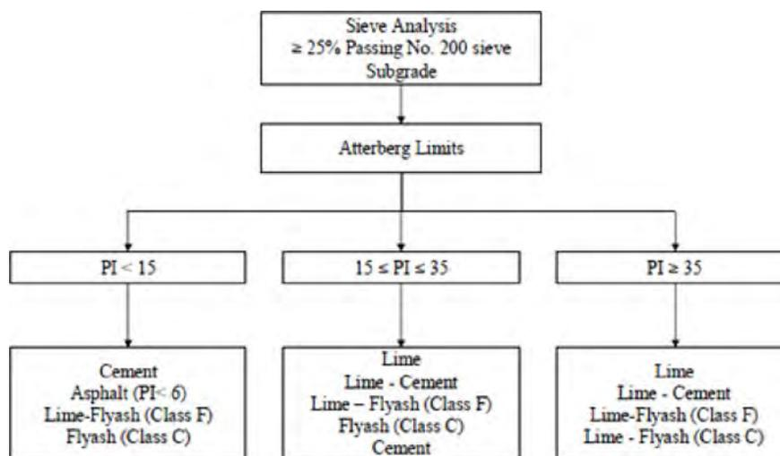
FIGURE 11 Flow chart for selecting additive for stabilizing soils (after Little and Nair 2009).
