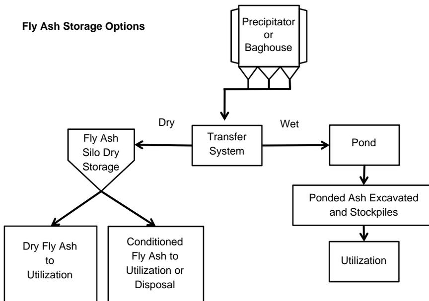
FIGURE 2 Fly ash storage options (continued from previous figure; after FHWA 2005).
