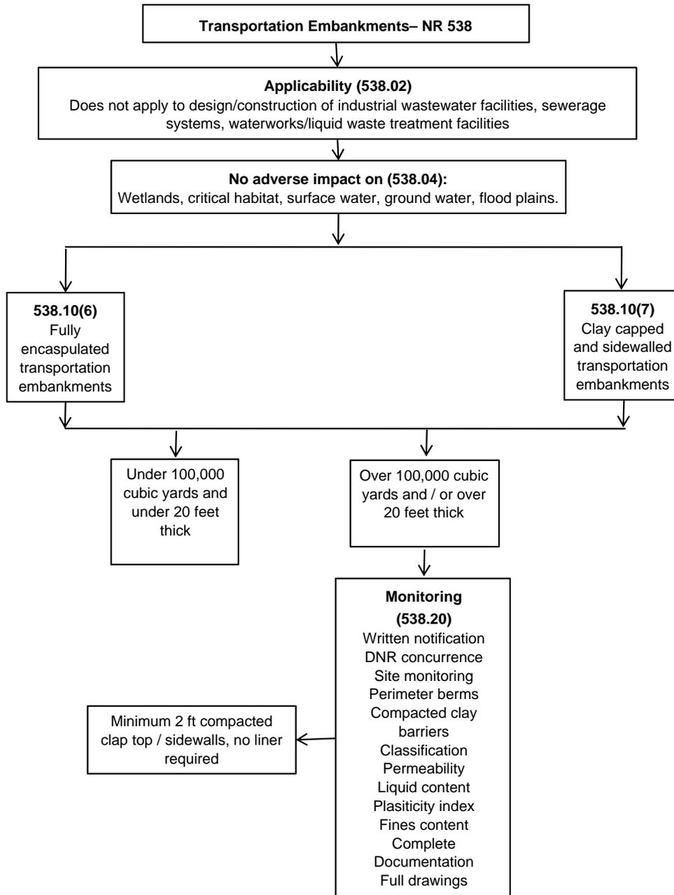
FIGURE 13 NR 538 Transportation Embankments Sections 538.6 and 538.7 (after WE Energies 2004).
