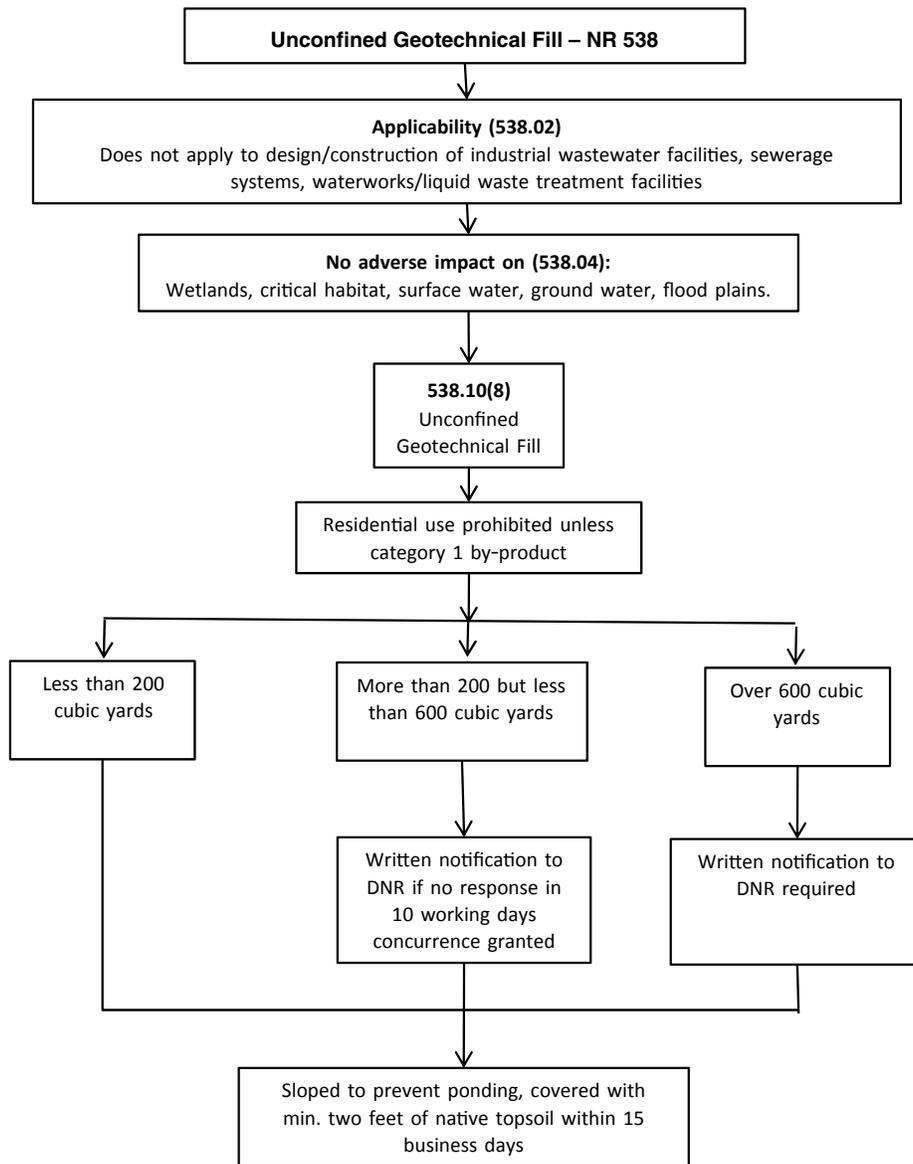
FIGURE 14 NR 538 Unconfined Geotechnical Fill Section 538.8 (after WE Energies 2004).
