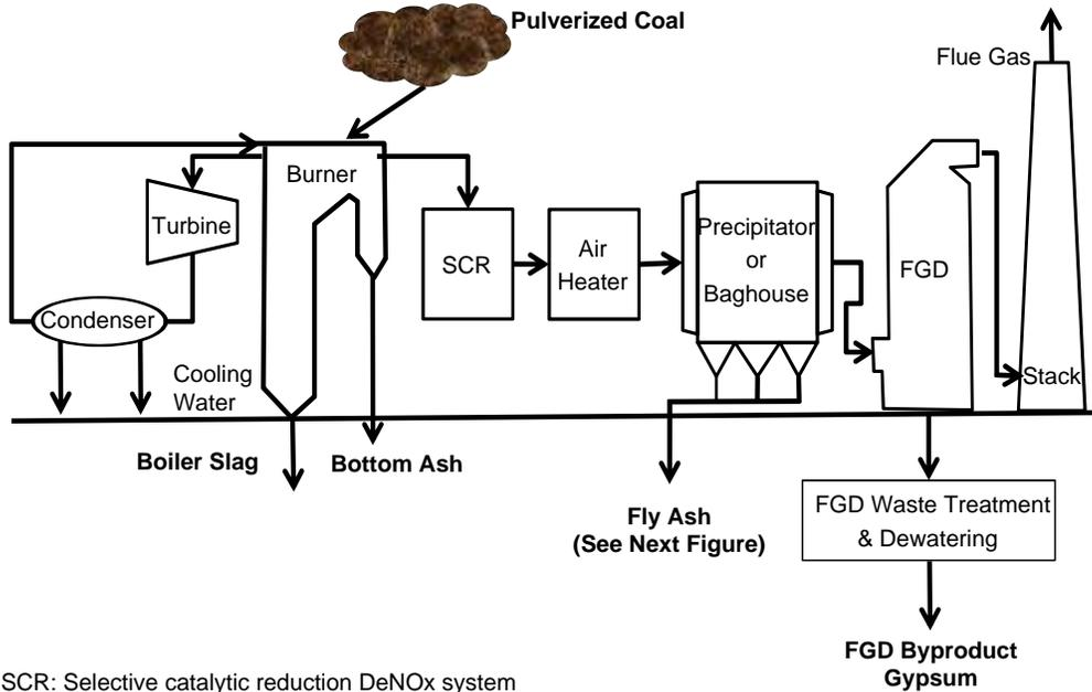
Schematic after Using Coal Ash in Highway Construction: A Guide to Benefits and Impacts. EPA April 2005
