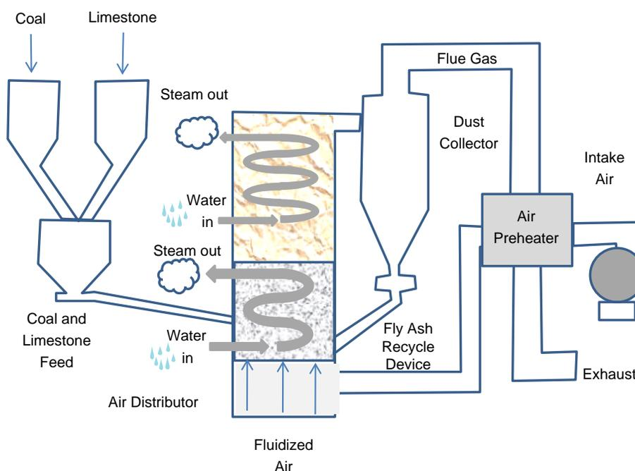
FIGURE 3 Schematic of a fluidized bed combustion boiler (EERC 2009).
