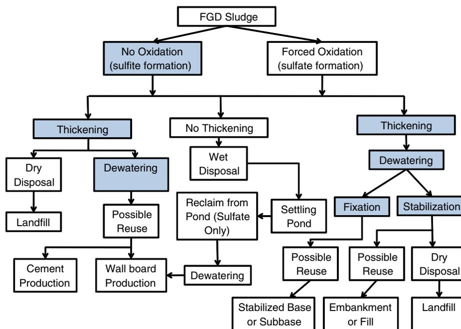
FIGURE 10 Flow chart for FGD sludge to product or landfill (after RMRC 2008).
