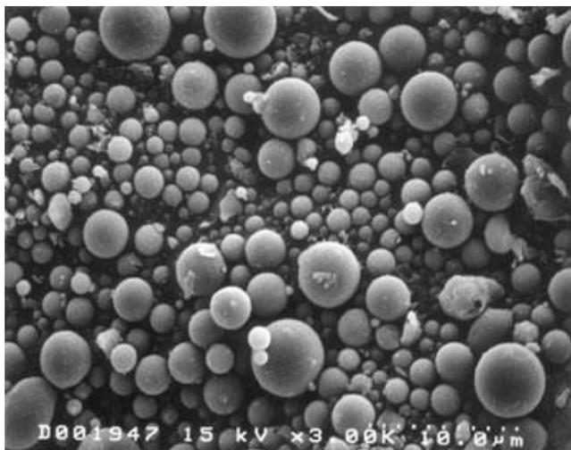
FIGURE 5 Fly ash at 2,000× magnification (FHWA and ACAA 2003).
