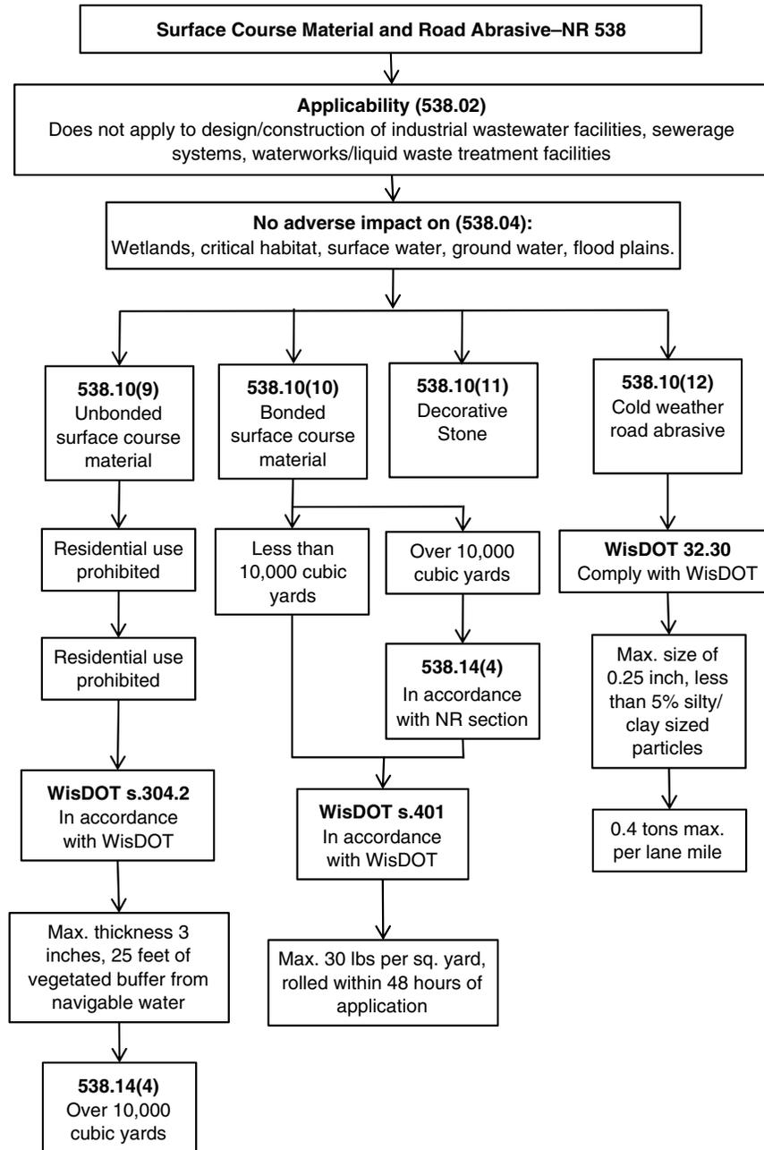
FIGURE 15 NR 538 Surface Course Material and Road Abrasive Sections 538.9 through 538.12 (after WE Energies 2004).
