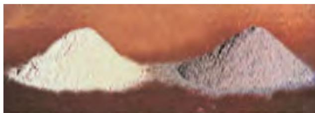
FIGURE 6 Examples of fly ash colors (FHWA and ACAA 2003).
