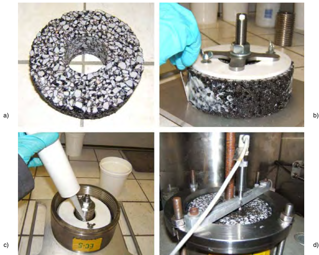
FIGURE 3 Coaxial shear test (CAST) for fatigue test (Partl et al. 2010): (a) sample cored out in the center then cut into 50 mm slices; (b) sealed with an epoxy resin; (c) samples are glued to an outer steel ring and an inner steel core; and (d) vertical deformation is recorded.
