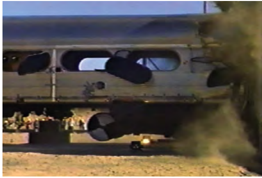
In tests of a single, conventional rail car crashing into a fixed barrier, the car body crippled haphazardly ( left ). The CEM equipment systematically absorbed the energy from the impact ( right ).
