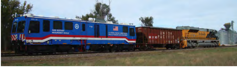
FRA DOTX-218 gage restraint measurement system with University of Nebraska–Lincoln’s track deflection system.
