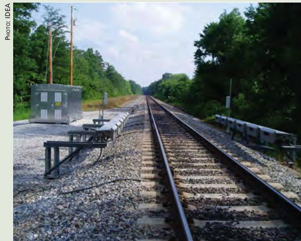
Installation of an IDEA project at the Transportation Technology Center, Inc., to detect railroad car truck hunting, or swaying.
