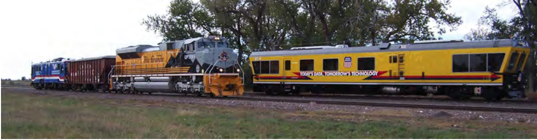
State-of-the-art track assessment vehicles near Cheyenne, Wyoming: Union Pacific EC-4 evaluation car and FRA DOTX-218 gage restraint measurement system in consist with University of Nebraska-Lincoln track deflection system.
