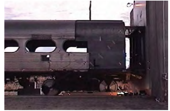
In tests of a single, conventional rail car crashing into a fixed barrier, the car body crippled haphazardly ( left ). The CEM equipment systematically absorbed the energy from the impact ( right ).
