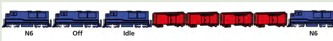
FIGURE 3 Trip Optimizer SmartHPT can calculate the optimal use of locomotive power and can dynamically autostart, shut down, or isolate locomotives as needed during a trip.
