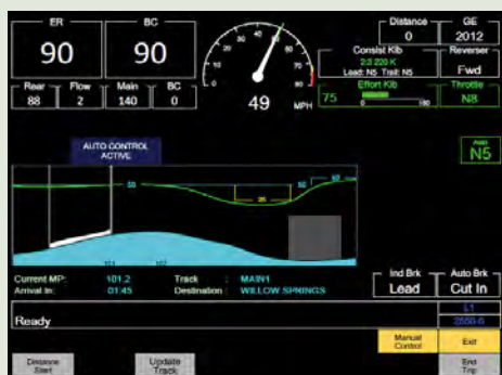
The Trip Optimizer handles throttle control for motoring and dynamic braking based on a route's topography. Fuel savings range from 3 to 17 percent.
