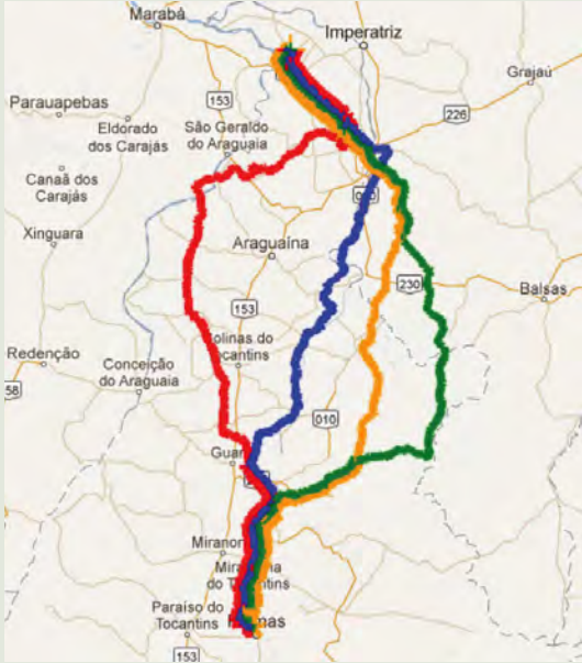
FIGURE A Illustrative example of four alternate routes for a hazardous material shipment. Each route (shown in a different color) is submitted to the RCRMS for a risk score. (NOTE: The illustration overlays hazardous material routes for a U.S. Class I railroad onto a Google map of Brazil to avoid security issues. The RCRMS is a U.S.-based risk model.)
