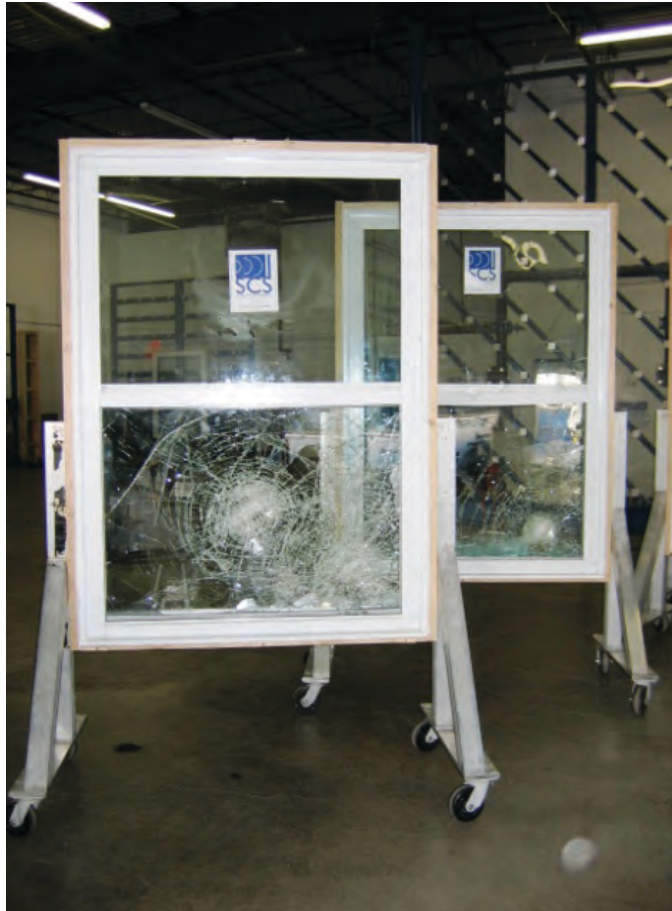
Figure 9.11. Successful completion of TAS 201 – Large Missile Impact Test and TAS 203 – Cyclic Load Test.
