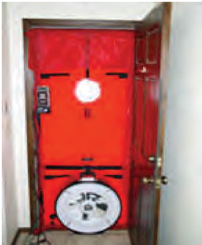
Figure 7.1. Blower-door test equipment.
