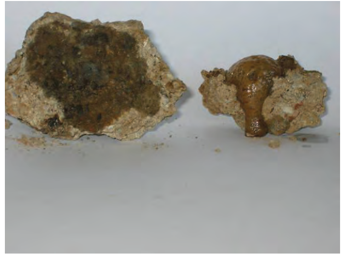
Hydrochloric acid reaction on disintegrated core
