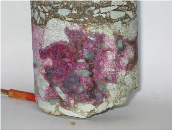
Phenolphthalein reaction on core
