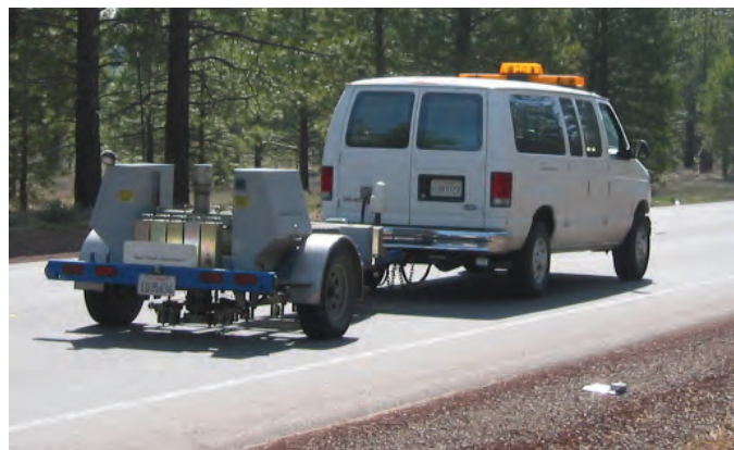
Figure 4.10. Falling Weight Deflectometer.
