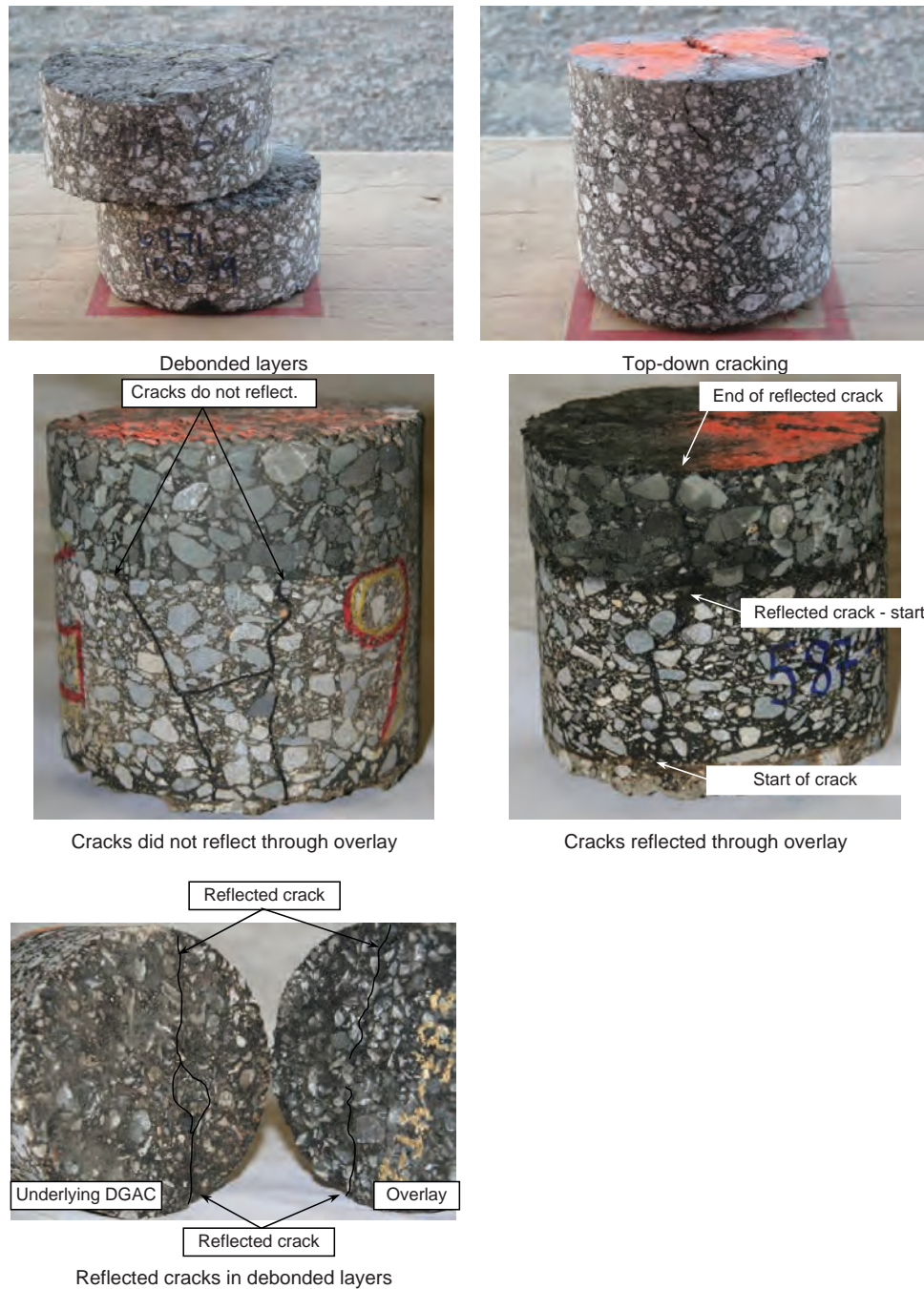
Figure 7.10. Examples of observations on asphalt cores.
