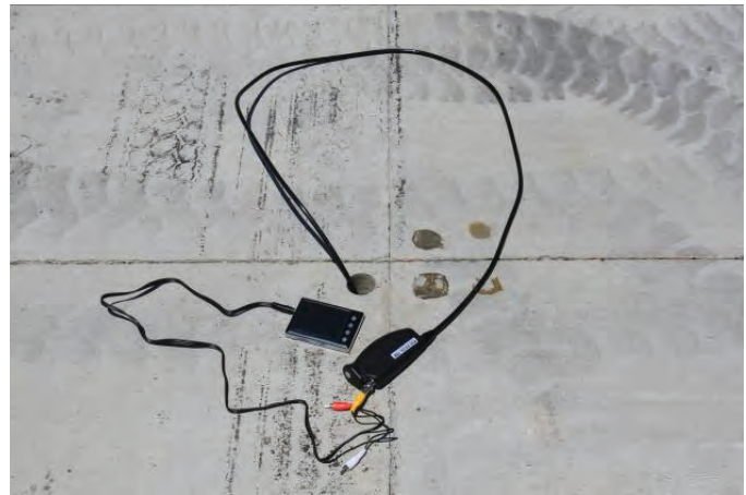
Figure 7.5. Example use of flexible video borescope in core hole.
