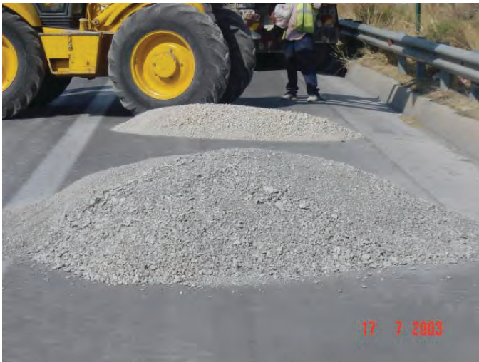
Figure 7.14. Separated layer samples from test pit excavation.
