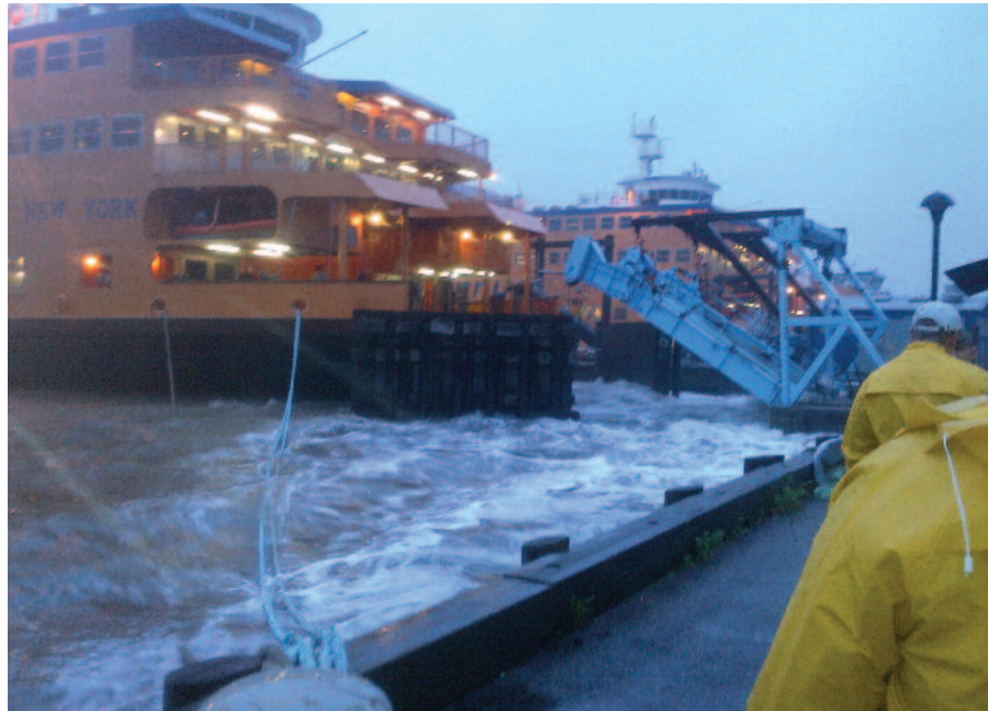
Staten Island Ferry crew and landside staff set heavy water moorings in advance of Superstorm Sandy, October 2012, at the Ferry Maintenance Facility piers in New York City harbor.
