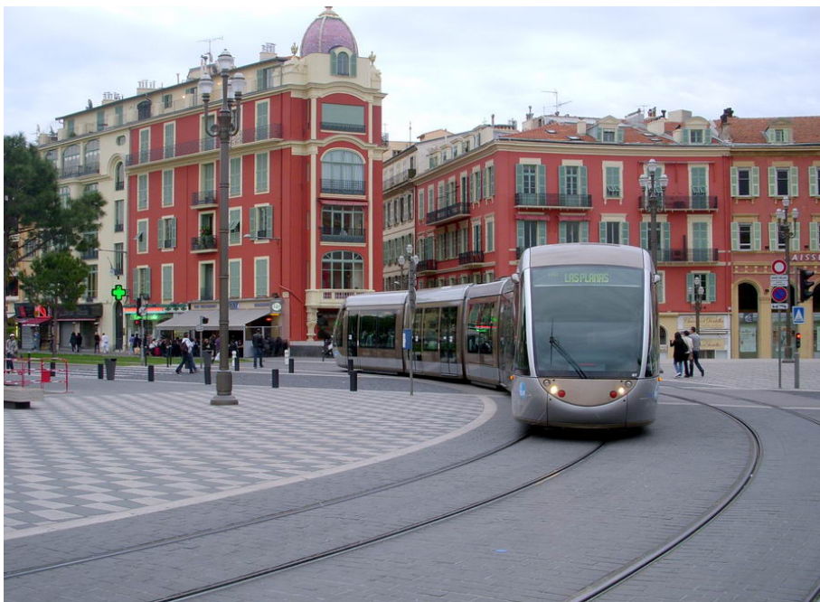
FIGURE 5 Off-wire operation in Nice, France.
