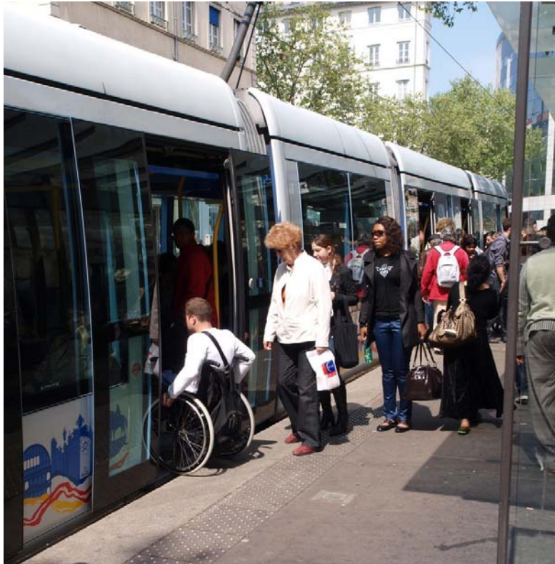
FIGURE 2 Step-free, level boarding: low-floor boarding allows step-free access for all, without the use of ramps or lifts (Lyon, France).
