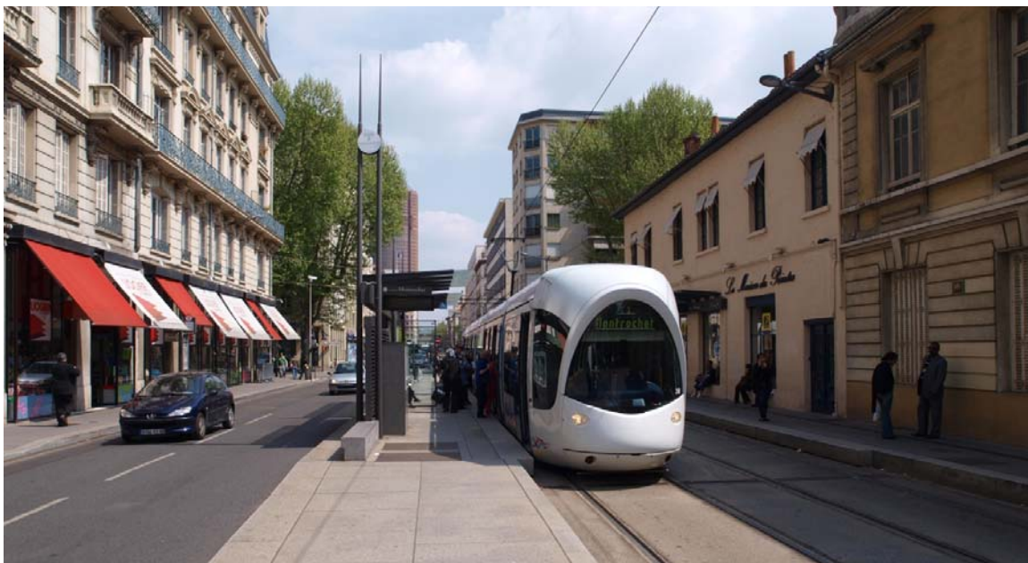
FIGURE 4 Segregated LRT operation. Segregated running maximizes the benefits of the LRT system through faster journey times and journey time reliability (Lyon, France).
