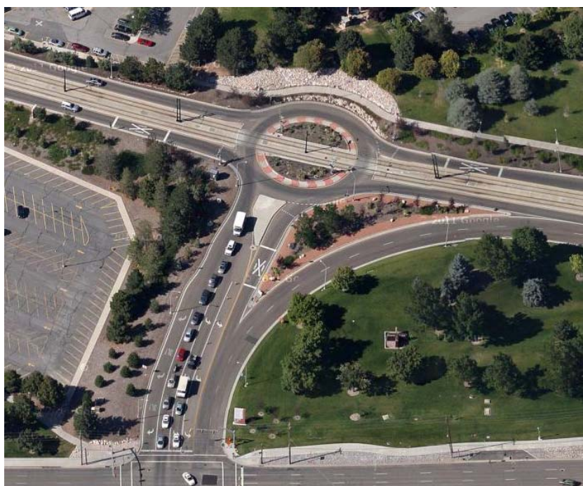
FIGURE 9 The University of Utah roundabout intersection in 2012. (Note two-lane bypass on the right side.) (Source: Google Maps.)
