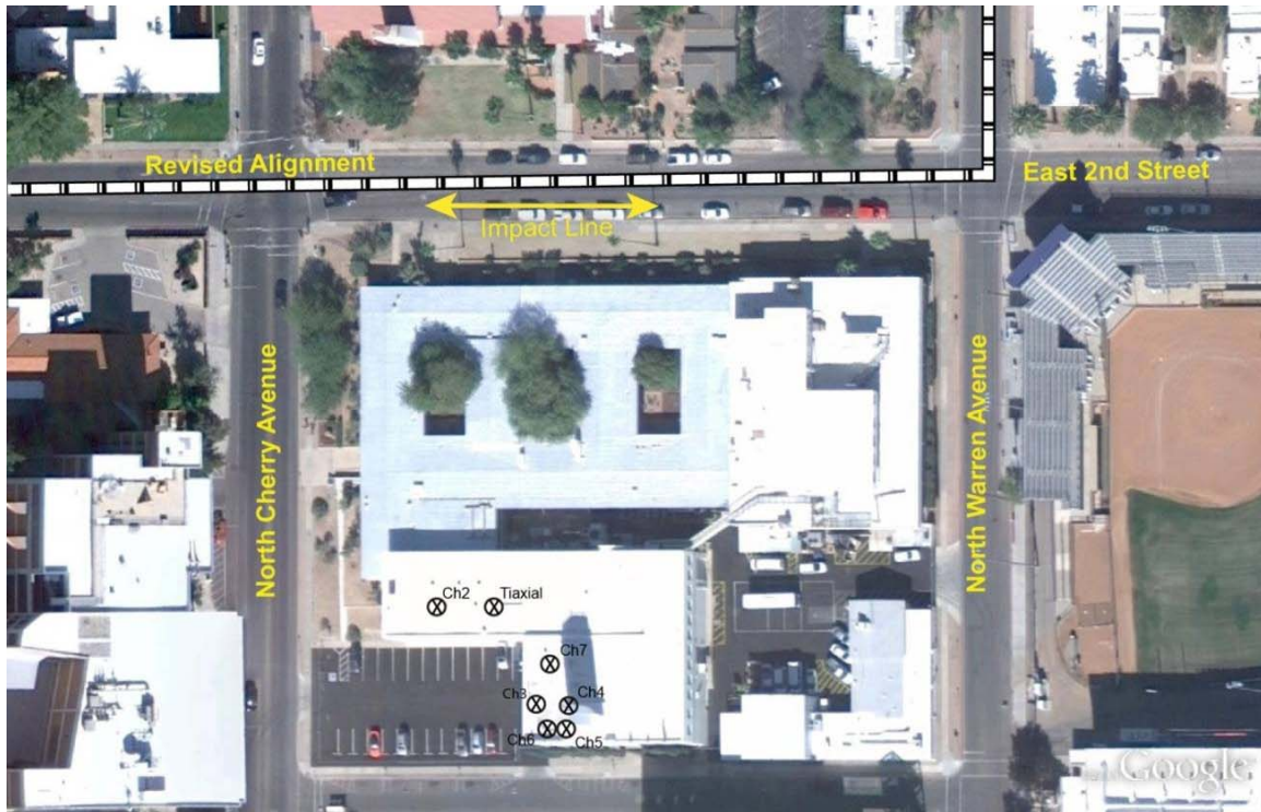
FIGURE 4 Vibration measurement positions for NOAO Optics Lab in Tucson (9).
