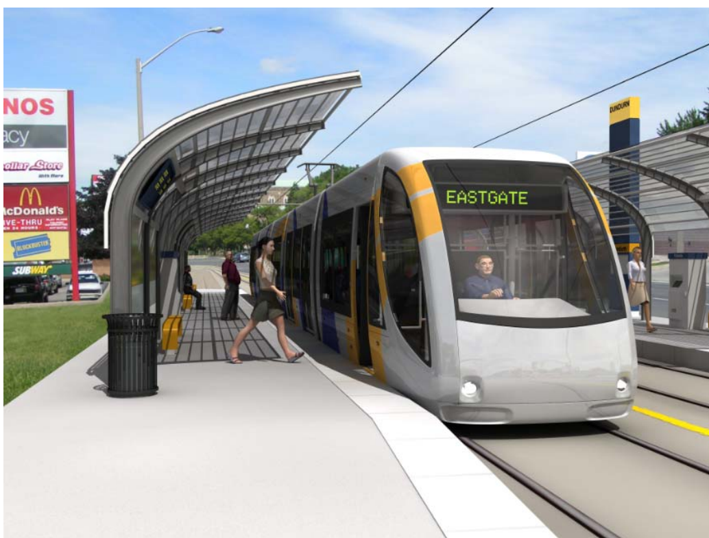
FIGURE 12 LRT envisaged on the Hamilton B-Line. The Hamilton B-Line will include 18 low-floor, level boarding stops, providing access for all.
