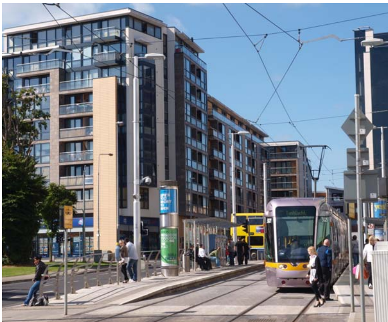
FIGURE 6 The Luas system is a European example of the urban-style LRT that is being designed in many cities in Canada, featuring level boarding, segregated running, and integration with TOD land uses.
