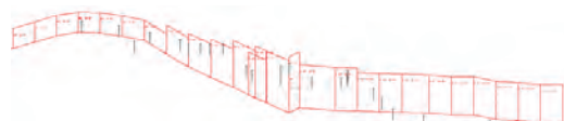
FIGURE 1 I-40–Jones Franklin Road noise wall with an initial jagged, acoustically inefficient top-of-wall profile.
