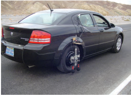
Vehicle equipped for research on tire-pavement noise on a roadway in Death Valley National Park.
