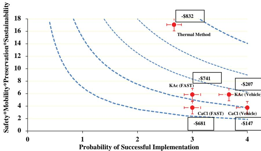
Figure B-13. Comparison of technology application bundles by integrating all summary metrics and POSI, using normative units, and including notations on agency-specific net cost (\$000s/bridge).
