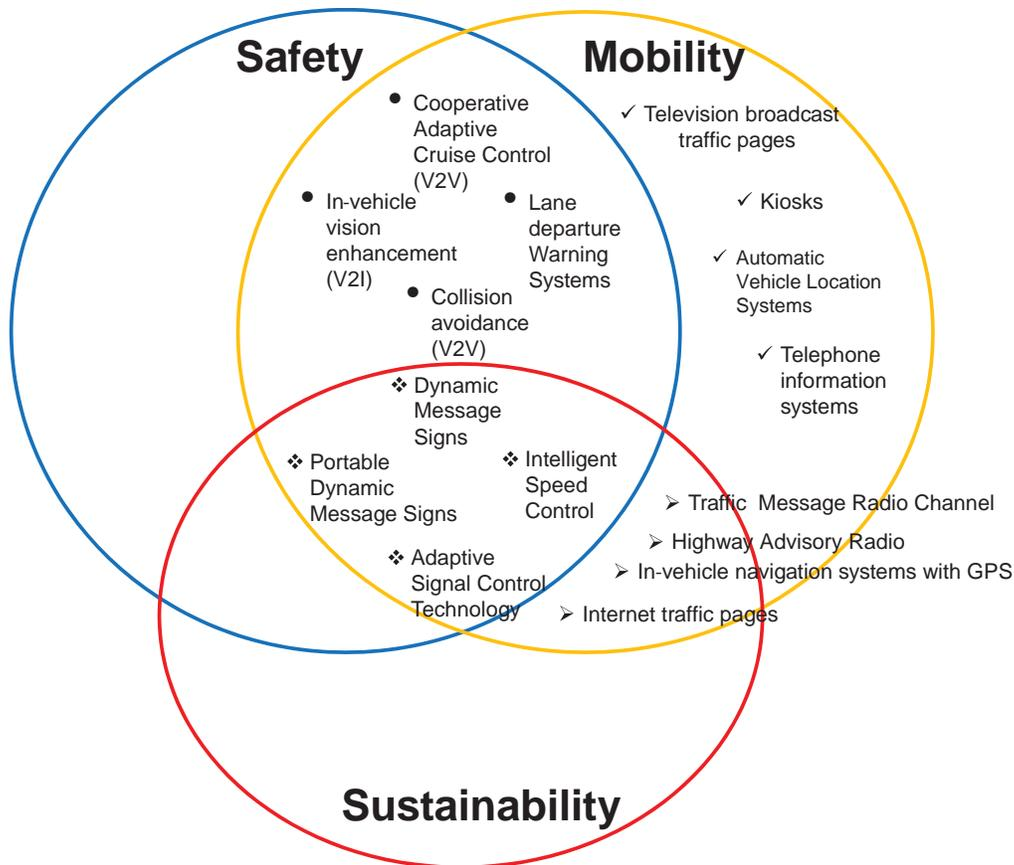
Figure C-1. Functional mapping of driver information system.
