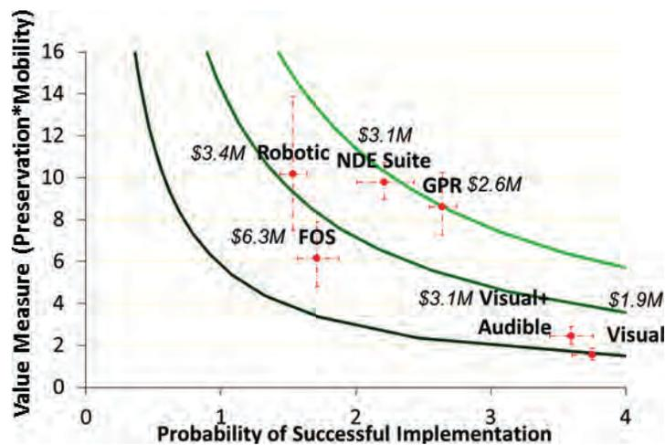
Figure 4-3. Value measure (preservation × mobility values) compared to implementation barriers with notations on equivalent costs
