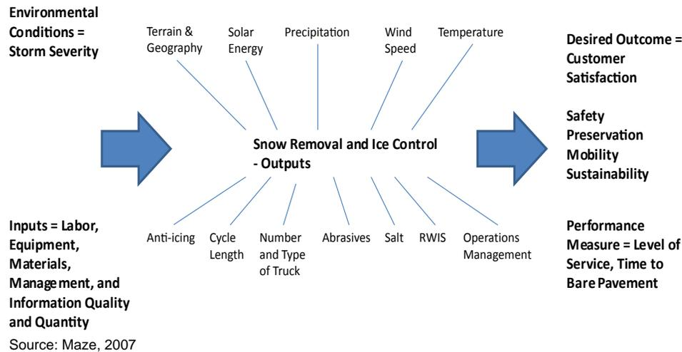
**Figure B-5. Relationship between inputs, outputs, and outcomes in snow removal and ice control.**
