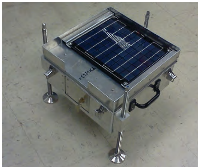
Figure 18. Photo of IR classifier cabinet with solar panel.
