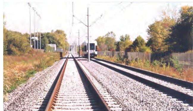
FIGURE 9 Ballasted track. Concrete ties, 115 rail, CWR, e-clip, with #3 ballast and overhead catenary.
