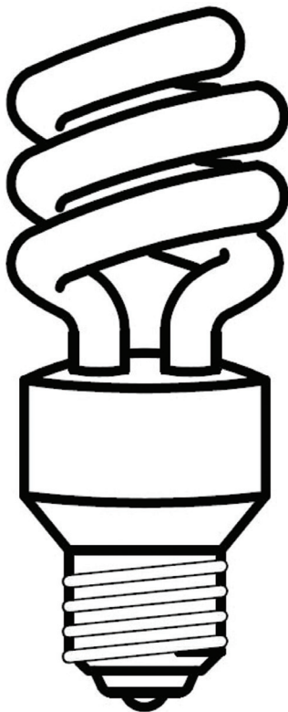
FIGURE 1.15 Compact fluorescent lamp (screw base with integral ballast).
