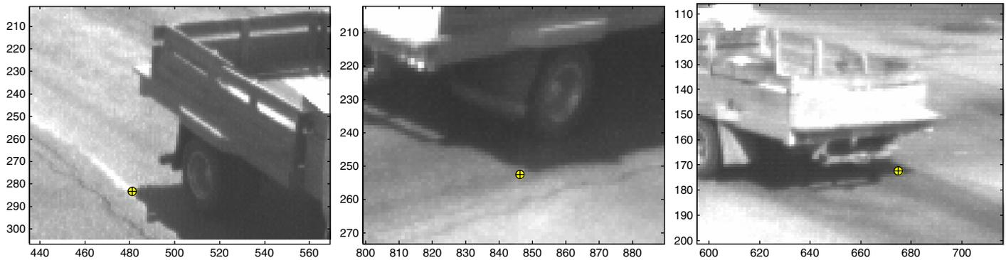
**Figure 7.12. Simultaneous images (zoomed in) from the NE, SE, and SW cameras. The marked point is coincident in time and in 3-D world coordinates. Scales are pixel coordinates.**
