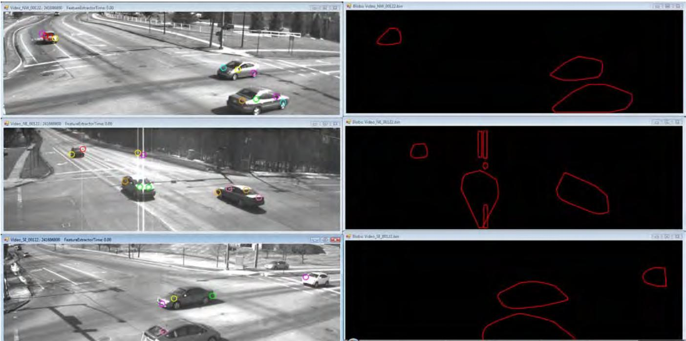
**Figure 8.4. Clusters and blobs, including effects of glare and erroneous features.**
