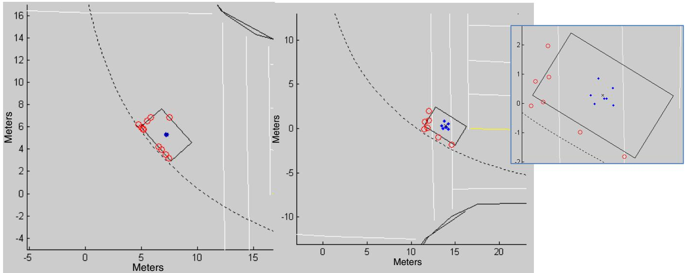
**Figure 10.2. Example of position refinement. Red circles are cluster projections; blue dots are centroid estimates. Left: At reference time. Right: At time  $t_{ref} + 1$ . Zoomed image also is at time  $t_{ref} + 1$ .**
