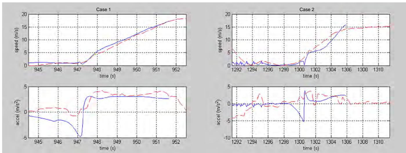
**Figure 11.8. Speed and acceleration estimates for slow-turning vehicles, right turn into path. Blue: video measurement; red dashes: vehicle measurement.**
