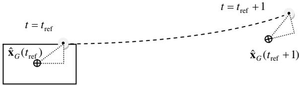
**Figure 10.1. Centroid position estimation by local coordinate rotation and offset. The dashed triangle indicates the fixed distances of lateral and longitudinal offset relative to the vehicle center.**
