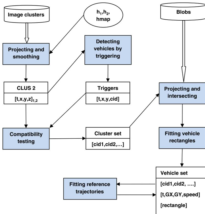
**Figure 9.13.** Block diagram summary of basic vehicle trajectory estimation.
