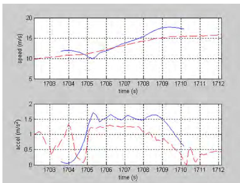
**Figure 11.9. LTAP/OD conflict—through vehicle. Blue: video based; red dashes: vehicle based.**
