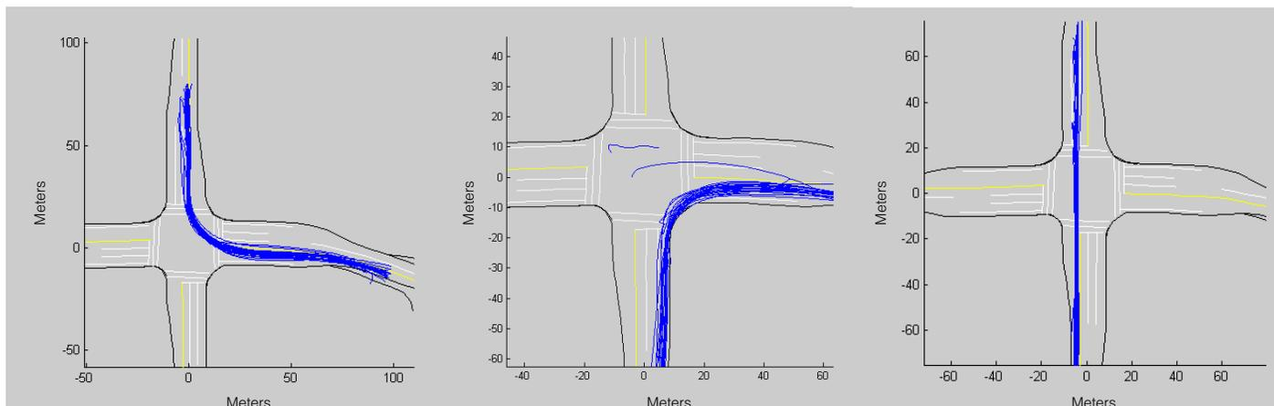
**Figure 11.4. Samples of detected trajectories in selected directions. The central plot shows a single corrupted trajectory. Less than 1% of trajectories are this type and can be removed by screening.**
