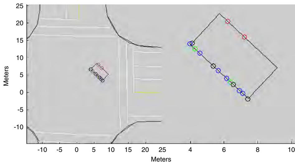
**Figure 9.9. Fitted rectangle and associated cluster points, including close-up (right plot). Colors according to camera corner location: NE, red; SE, green; SW, blue; and NW, black.**
