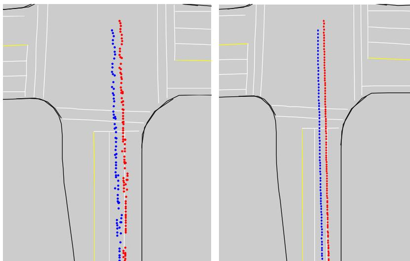
**Figure 9.1.** A single-cluster track resolved in world coordinates at an assumed height of 0.5 m (blue) and 1.5 m (red), with vehicle traveling to the north, viewed from NE camera.
