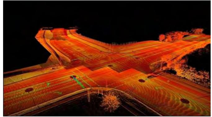
**Figure 7.4.** Virtual lidar survey image of the test intersection.
