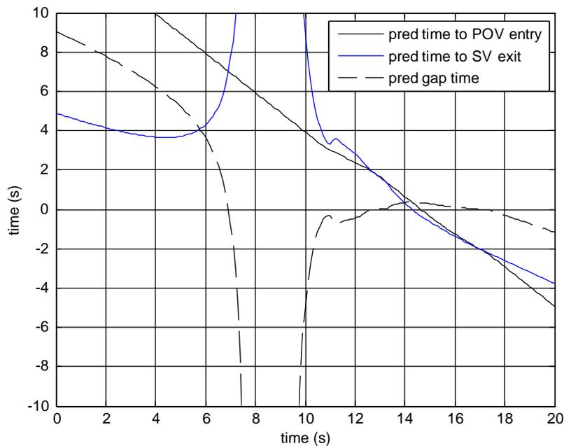
**Figure 5.4. Predicted times of encroachment and gap time for LTAP/OD scenario.**
