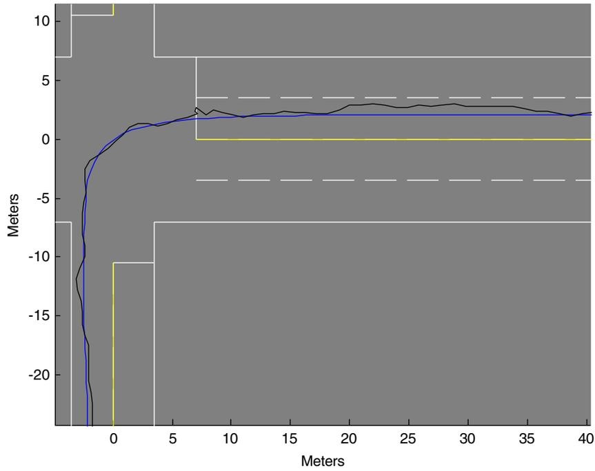
**Figure 5.8. Effect of medium level spatial errors on the trajectory (blue: reference; black: perturbed).**
