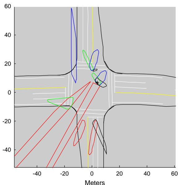
**Figure 9.5. Multicamera blob projections at time  $t_{ref}$ . The black star shows the location of the centroid of associated clusters. Colors denote camera source: NE, blue; SE, red; SW, green; and NW, black.**
