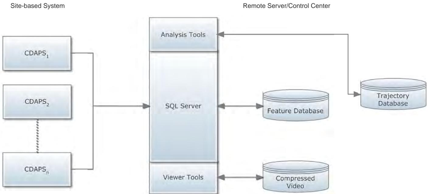
**Figure 6.6. Integrated vehicle tracking system—Site Observer.**
