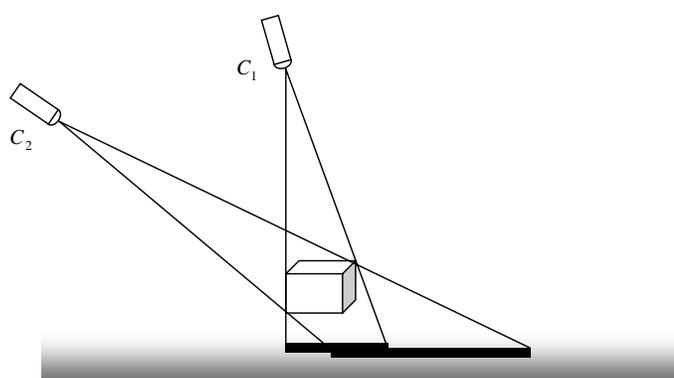
**Figure 6.2. Effect of camera viewing (altitude) angle on boundary estimation.**
