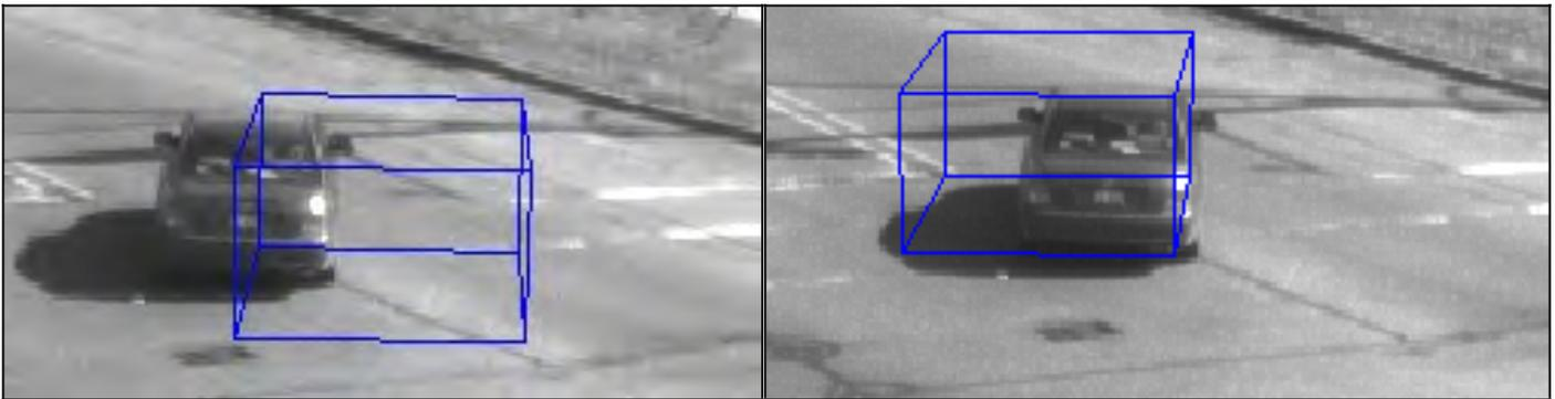
**Figure 10.4. Lateral offset attributable to vehicle shadow. No shadow compensation has been applied in this analysis. Time:  $t_{ref} + 1$ .**
