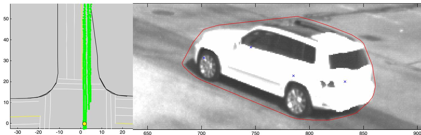
**Figure 8.6. World view and camera view of cluster tracks on a single vehicle (through vehicle traveling north).**
