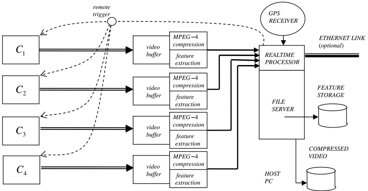
**Figure 6.5. Camera, data acquisition and preprocessing system (CDAPS).**
