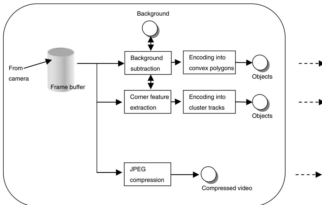
**Figure 8.1.** Image processing steps at an individual camera station.
