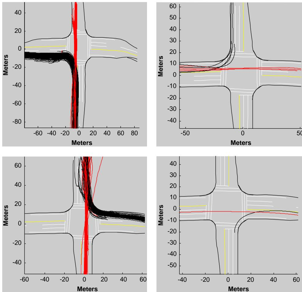
**Figure 12.4. Vehicle trajectories used for TTC analysis.**
