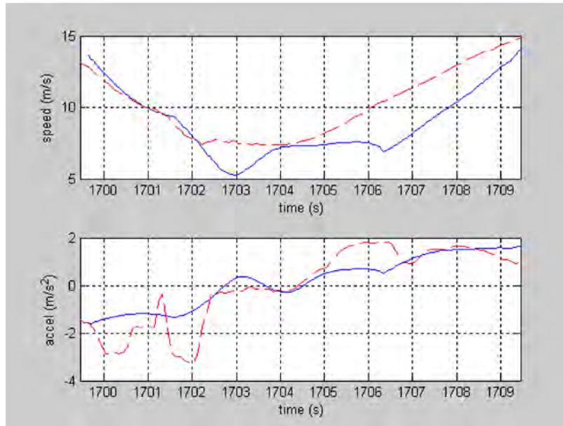
**Figure 11.10. LTAP/OD conflict—turning vehicle. Blue: video based; red dashes: vehicle based.**
