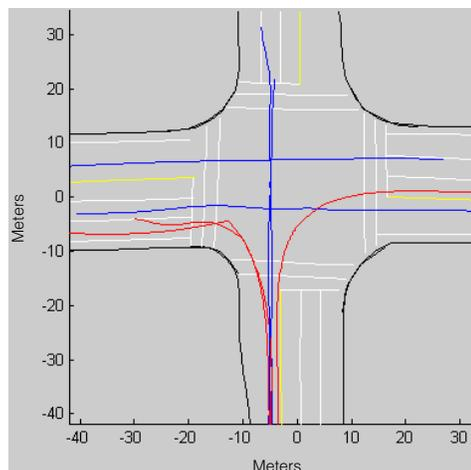
**Figure 11.6. Simulated conflict paths using instrumented vehicles.**
