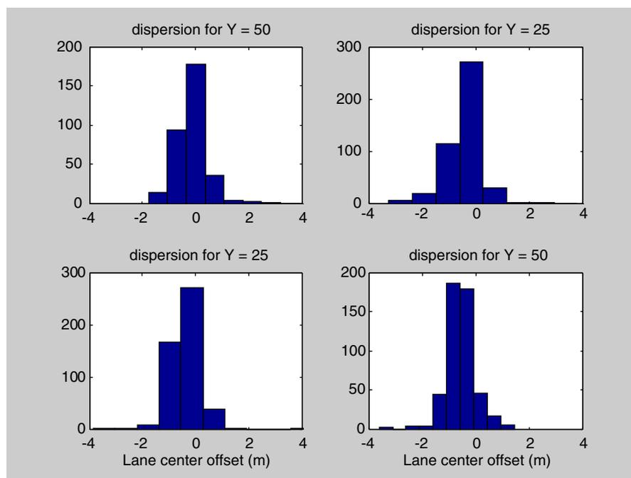
**Figure 11.5. Frequency distributions for lateral dispersion within the lane for through vehicles. North-to-south movement: upper left, 50 m north; upper right, 25 m north; lower left, 25 m south; and lower right, 50 m south.**
