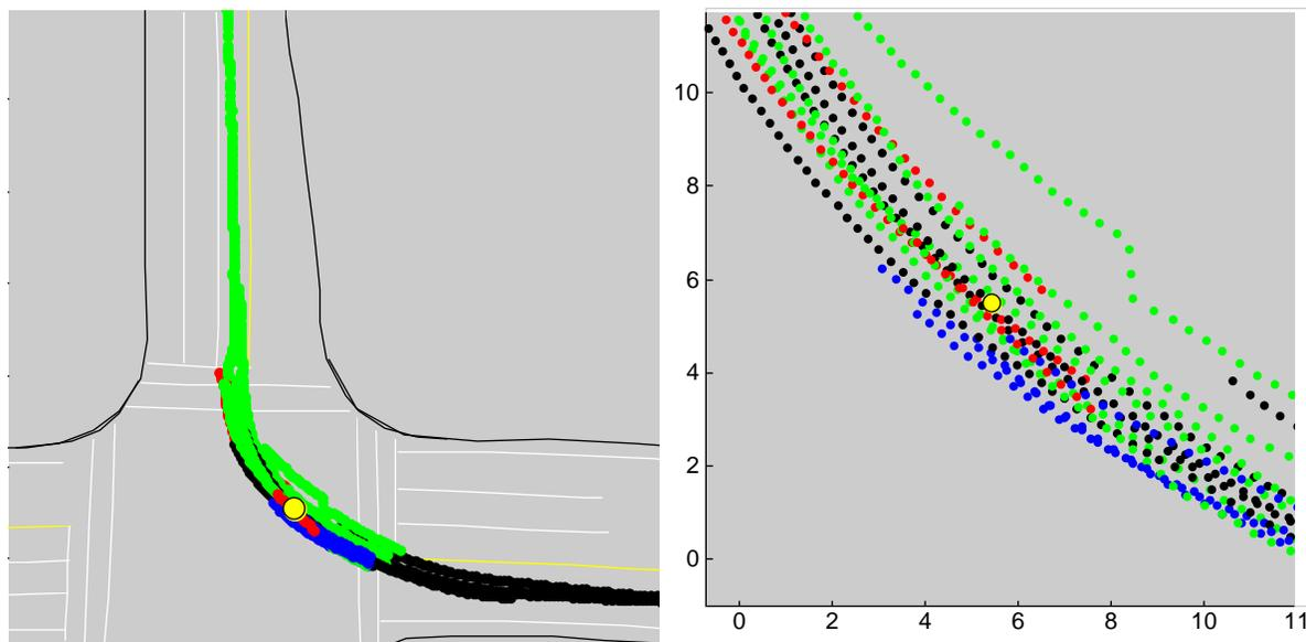
**Figure 9.4. Multicamera cluster tracks using a nominal 0.5-m assumed height above ground. Left plot shows detail. Yellow dot is reference track at reference time. Tracks are seen from cameras at the NE (blue), SE (red), SW (green), and NW (black) corners. Scales are in meters.**
