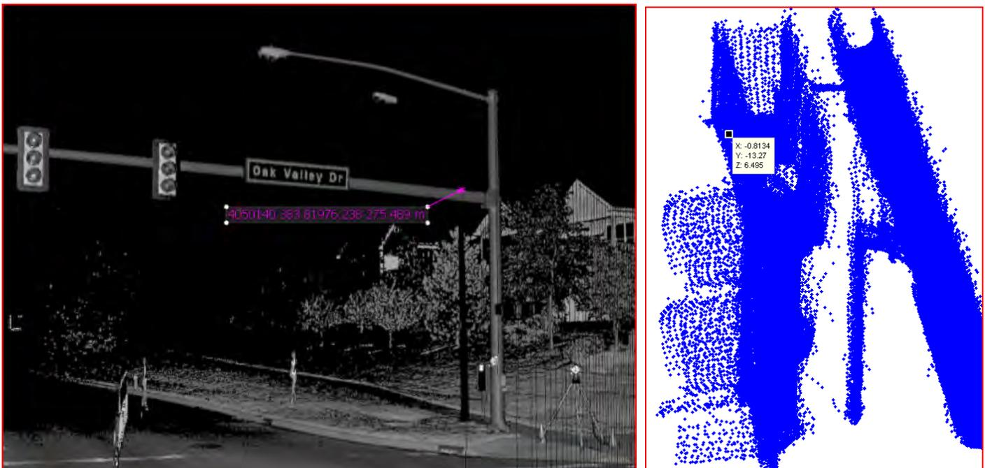
**Figure 7.5.** Virtual view from lidar survey using Leica TruView software. Right: detail of reference point on traffic signal used for camera calibration.
