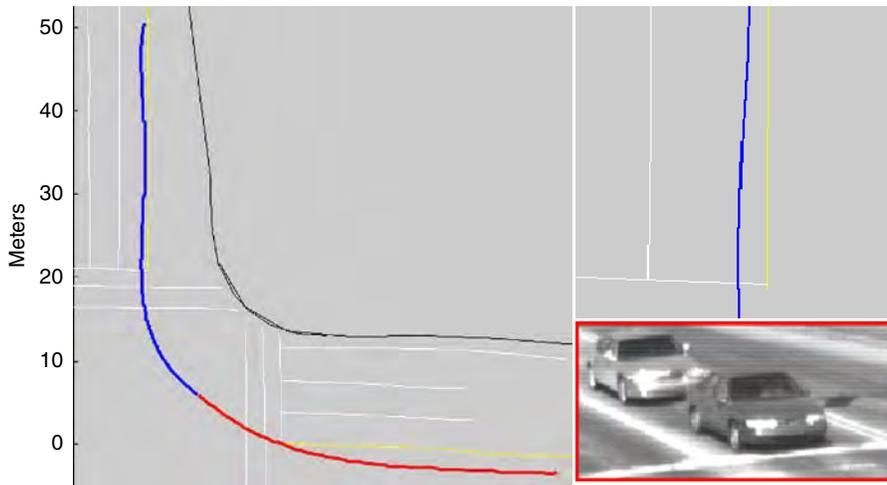
**Figure 9.11. Basic vehicle fitted path (red: using outgoing cluster; blue: using incoming cluster). The right plot shows a detail of the track near the stop bar; corresponding vehicle image is for the front car at the stop bar.**
