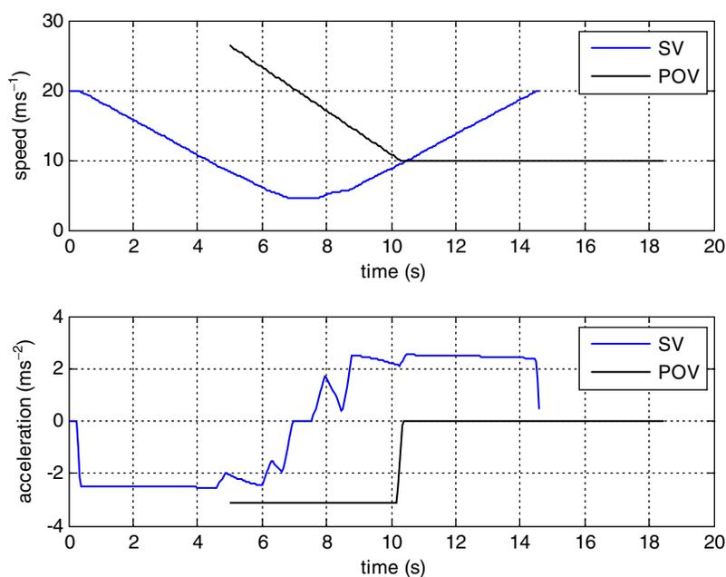
**Figure 5.6. Vehicle's speeds and longitudinal accelerations.**
