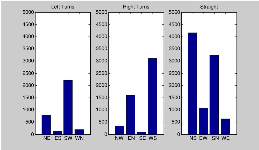
**Figure 11.1.** Traffic volumes during the 30-h study period (NE: enter from the north, exit toward the east, and so forth; 17,593 vehicle trajectories were recorded).
