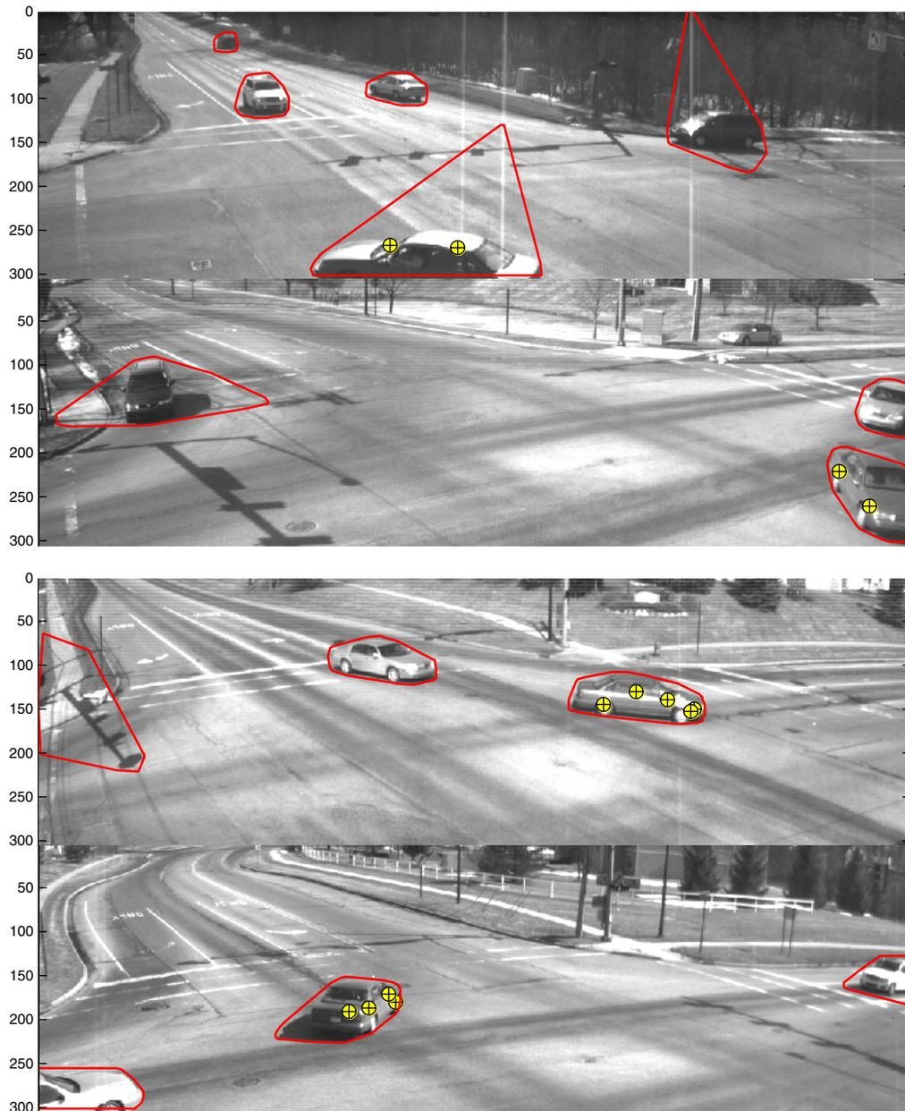
**Figure 9.3.** Simultaneous images of a turning vehicle identified with 18 cluster tracks. From the top, the cameras are located at the NE, SE, SW, and NW corners, respectively. Scales are in pixel coordinates.
