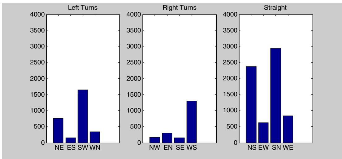
**Figure 11.2.** Traffic volumes during a comparable 24-h study period (from Traffic Signal Camera System, courtesy of Washtenaw County Road Commission; 11,622 vehicle movements were detected).
