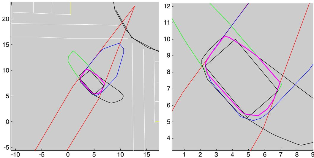
**Figure 9.6. Detail and vehicle localization by intersecting blobs. Blob color codes are the same as in Figure 9.5, with the addition of a magenta bounding polygon and fitted rectangle (black). Distances are in meters.**
