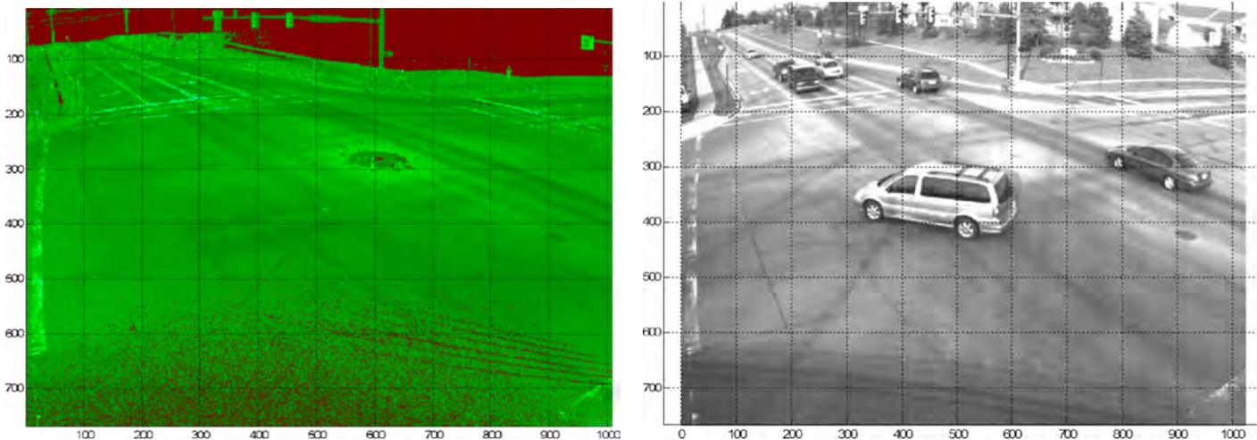
**Figure 7.9. Virtual and actual camera views (SW camera).**
