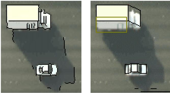
**Figure 3.4. Detected line segments (left) and the detection result (right).**
