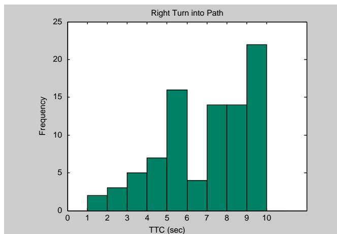
**Figure 12.7. Distribution of time-to-collision times, right turn into path (200 events).**
