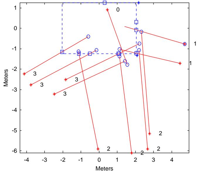
**Figure 9.8. Cluster localization using a vehicle rectangle (vehicle coordinate system:  $X_v$  is horizontal,  $Y_v$  is vertical; units are in meters). Numeric values adjacent to cluster lines indicate the camera location: 0 = NE, 1 = SE, 2 = SW, and 3 = NW.**
