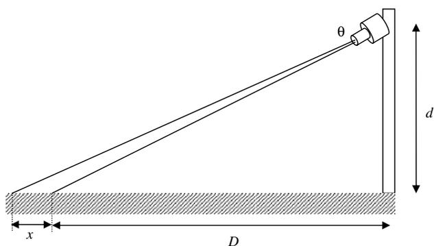
**Figure 6.1. Basic camera geometry and resulting pixelation error.**
