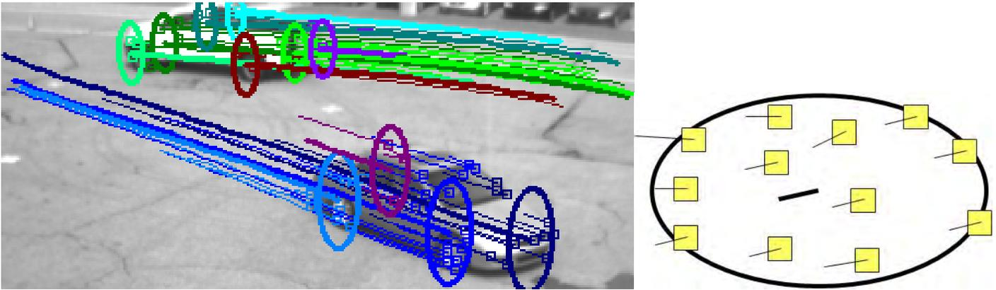
**Figure 8.3.** The clustering algorithm uses corner feature grouping and is sensitive to distances in the image. **Left:** Feature tracks and clusters on two vehicles (parking lot test at UMTRI). **Right:** Dispersion and mean velocities are recorded as part of the cluster properties.
