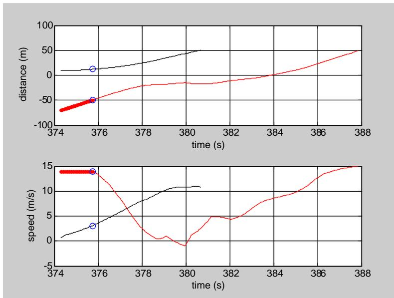
**Figure 12.5. RTIP conflict. Red: through vehicle; black: turning vehicle; blue circle: point of minimum time to collision.**
