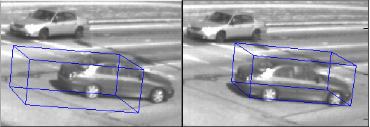
**Figure 10.3. Effect of position refinement. Left: Initial approximation from single cluster and nominal height estimate. Right: Uses position refinement by coordinate offsets. Time:  $t_{ref} + 0.7$ .**
