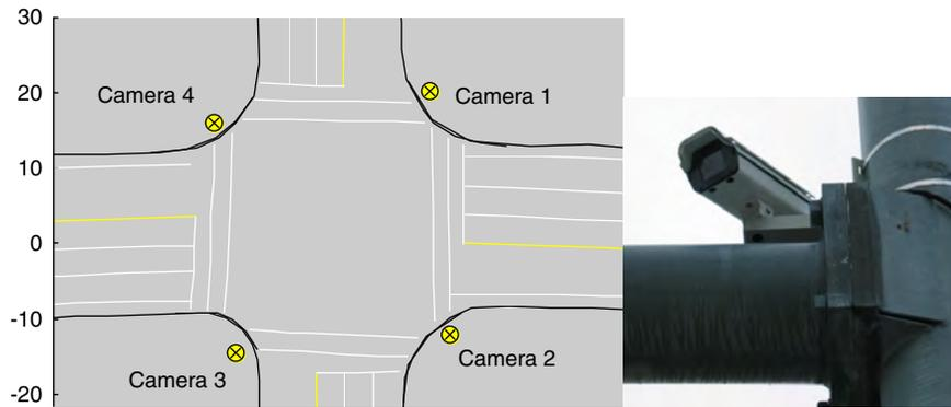
**Figure 7.8. Camera positions. Left: Plan view. Right: Mounting positions are on traffic signal mast arms, close to the signal mast (Camera 3 is shown here).**
