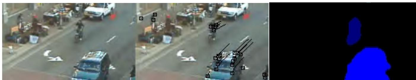
**Figure 8.2.** An example video image (left), a corner feature detection and tracking result (center), and a background subtraction result (right).
