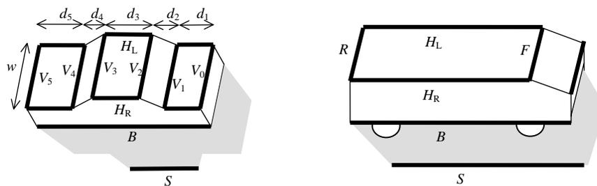
**Figure 3.3. The wireframe models used by the NGSIM system to detect a passenger vehicle (left) and a container truck (right).**
