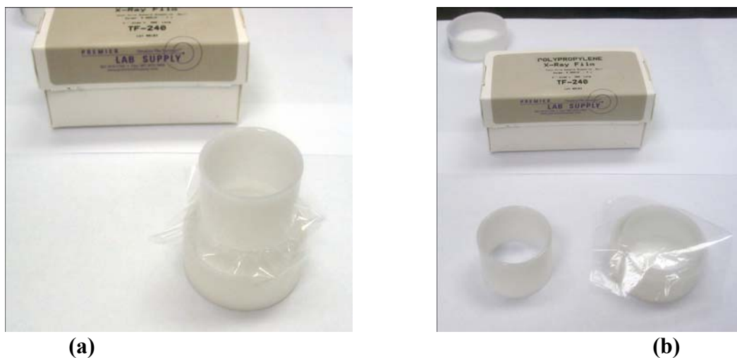
FIGURE 1 (a) Two cup halves and film and (b) assembling cup halves to form test cup.
