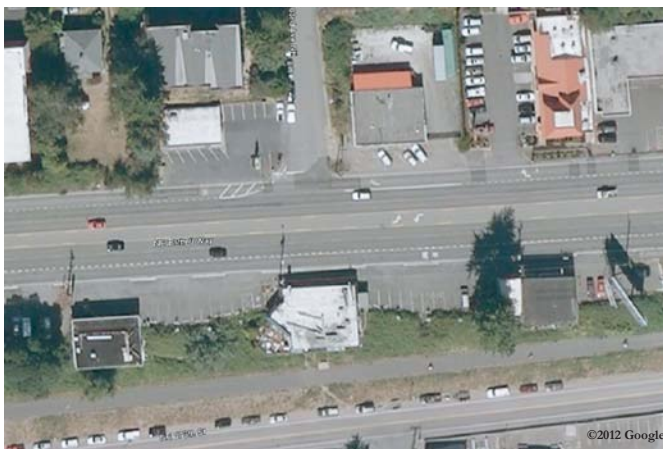
Figure 5-2. SR-522 at 63rd Avenue, arterial BOS pavement markings at minor intersection (Kenmore, Washington—Image via Google Earth).
